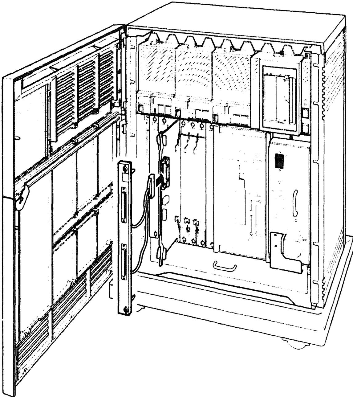
Figure 5-2 Installing the Gap Filler Assembly
