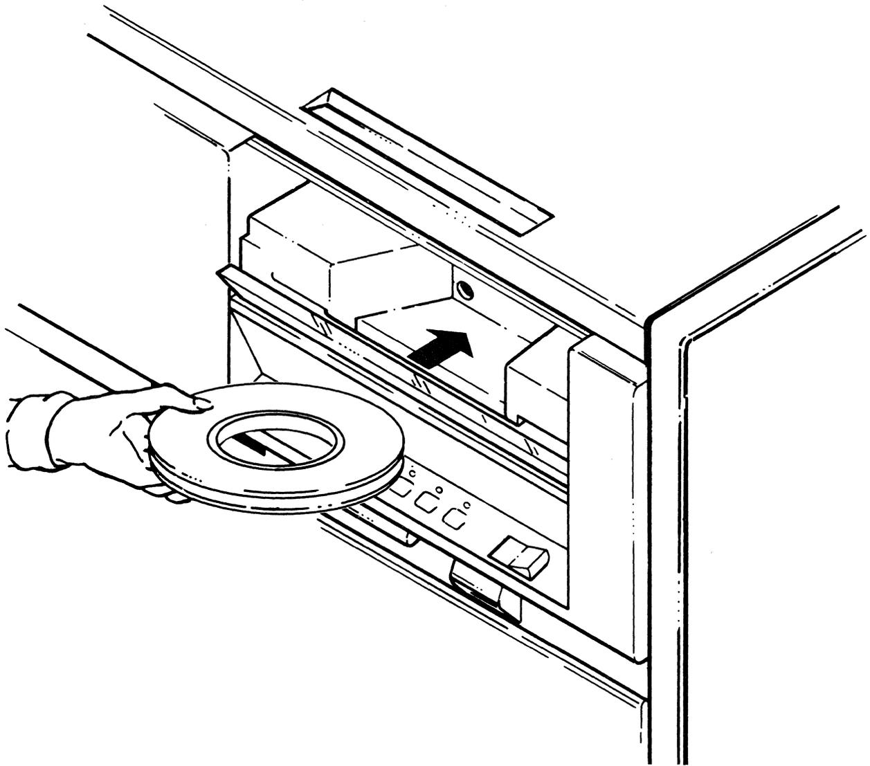
Figure 2-17 Inserting Tape
