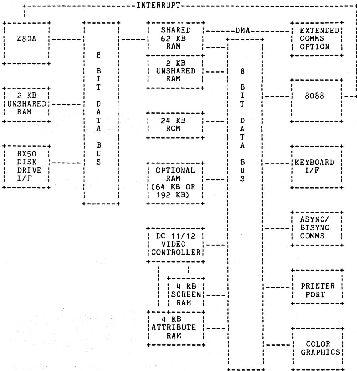
Figure 1. Mother Board Block Diagram
