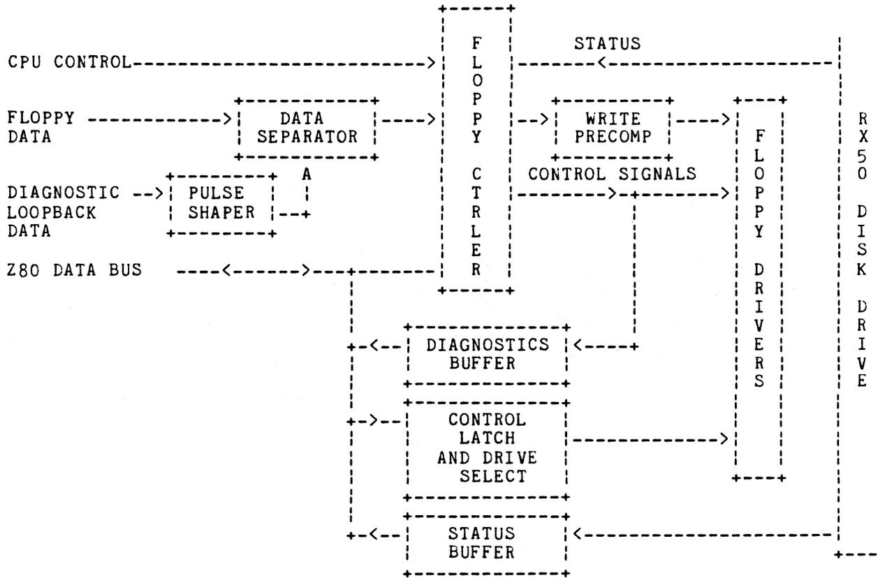
Figure 7. Floppy Controller Block Diagram
