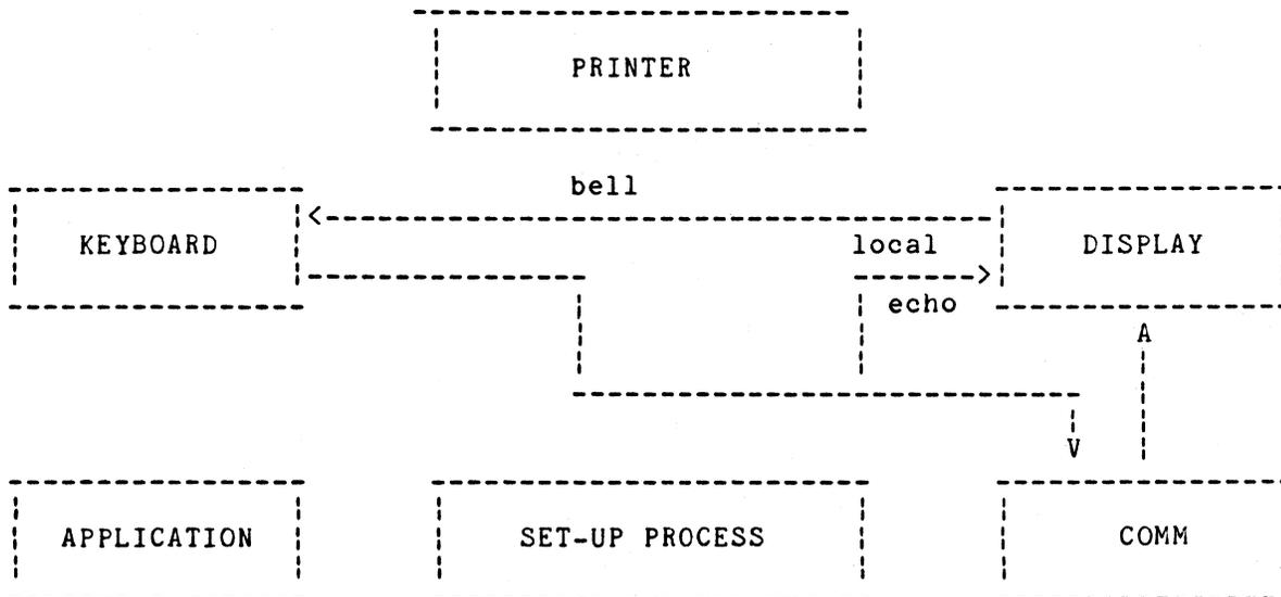
Figure 3. "Terminal" Mode "On Line" No Printer Functions
