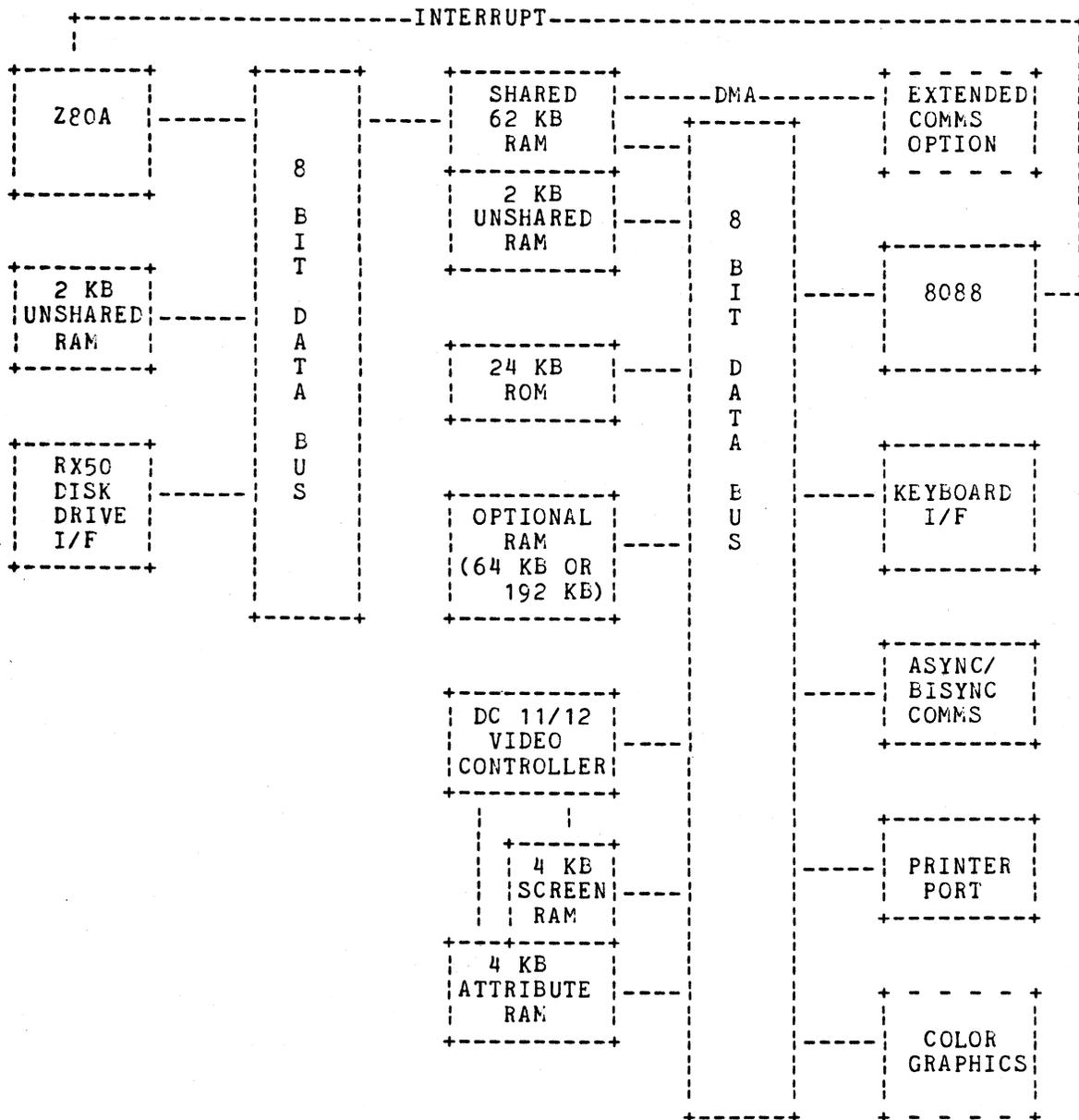
Figure 1. System Module Block Diagram
