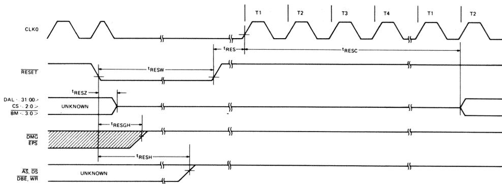
Figure 43 • MicroVAX 78032 Reset Timing Sequence
