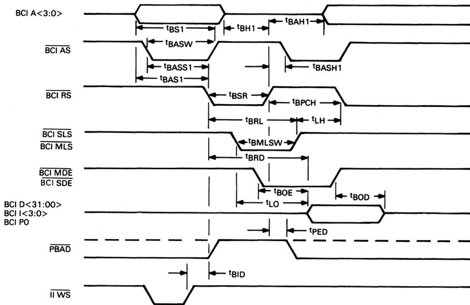
Figure 6 • VAXBI 78743 BCI Bus Interface Read Transaction Timing
