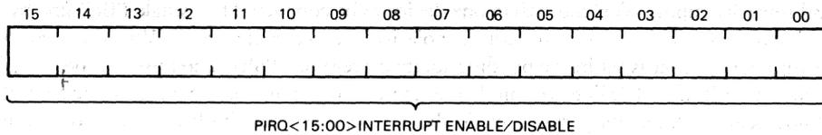
Figure 7 • MicroVAX 78516 Interrupt Enable Register Format
