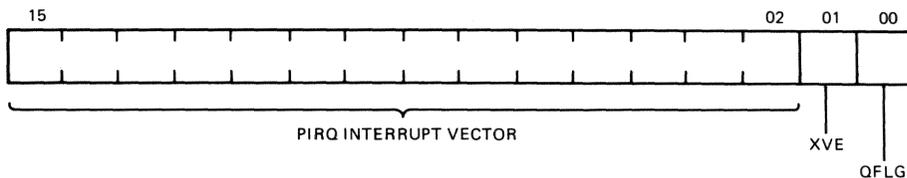
Figure 10 • MicroVAX 78516 Interrupt Vector Registers (0-15) Format
