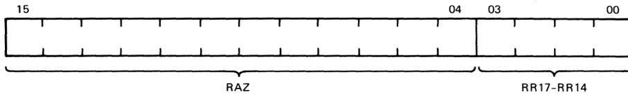
Figure 9 • MicroVAX 78516 Round Robin Register Format
