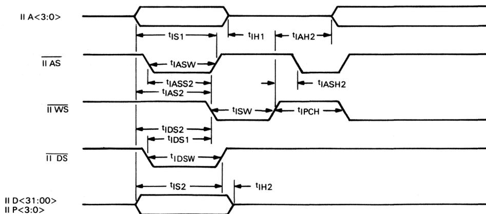
Figure 9 • VAXBI 78743 II Bus Interface Write Transaction
