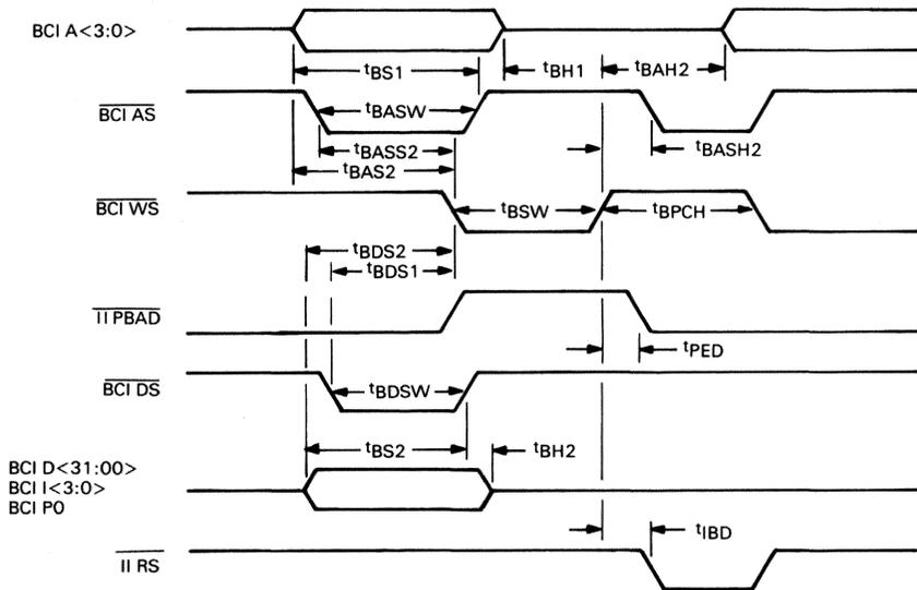
Figure 7 • VAXBI 78743 BCI Bus Interface Write Transaction Timing
