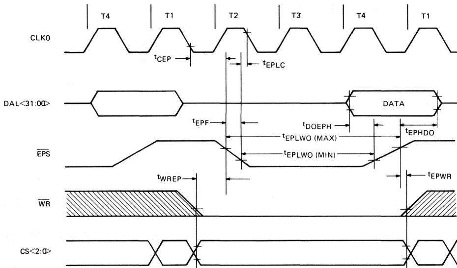
External Processor Write/Command Timing
