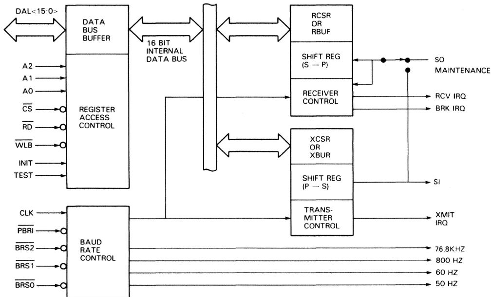
Figure 1 • DC319-AA DLART Block Diagram
