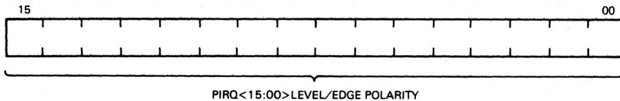
Figure 4 • MicroVAX 78516 Polarity Register Format
