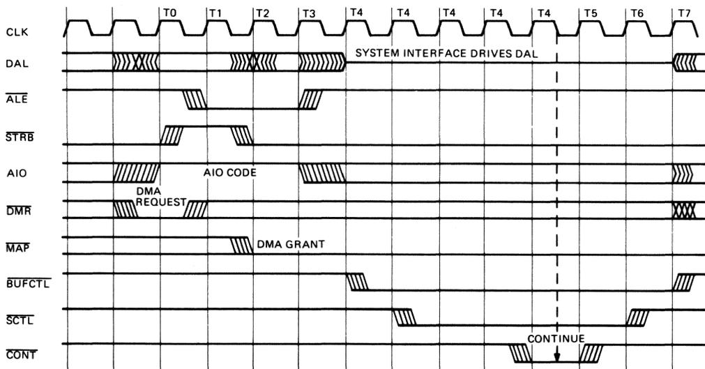
Figure 18 • DCJ11 Stretched Non-I/O Timing Sequence
