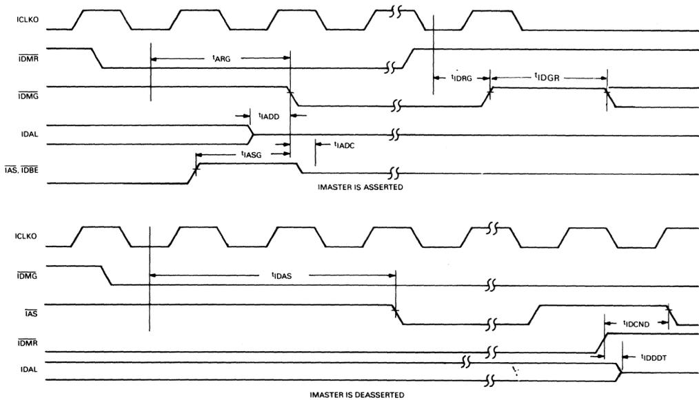
Figure 40 • MicroVAX 78532 I/O Bus DMA Cycle Timing
