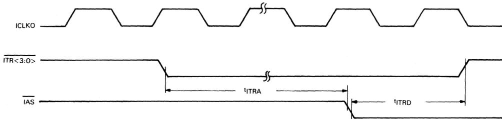
*Figure 41 • MicroVAX 78532 I/O Bus Transfer Request Timing*
