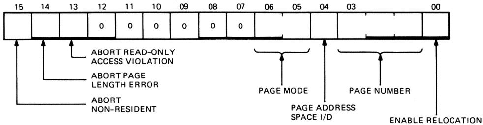
Figure 14 • DCJ11 Memory Management Register 0 Format
