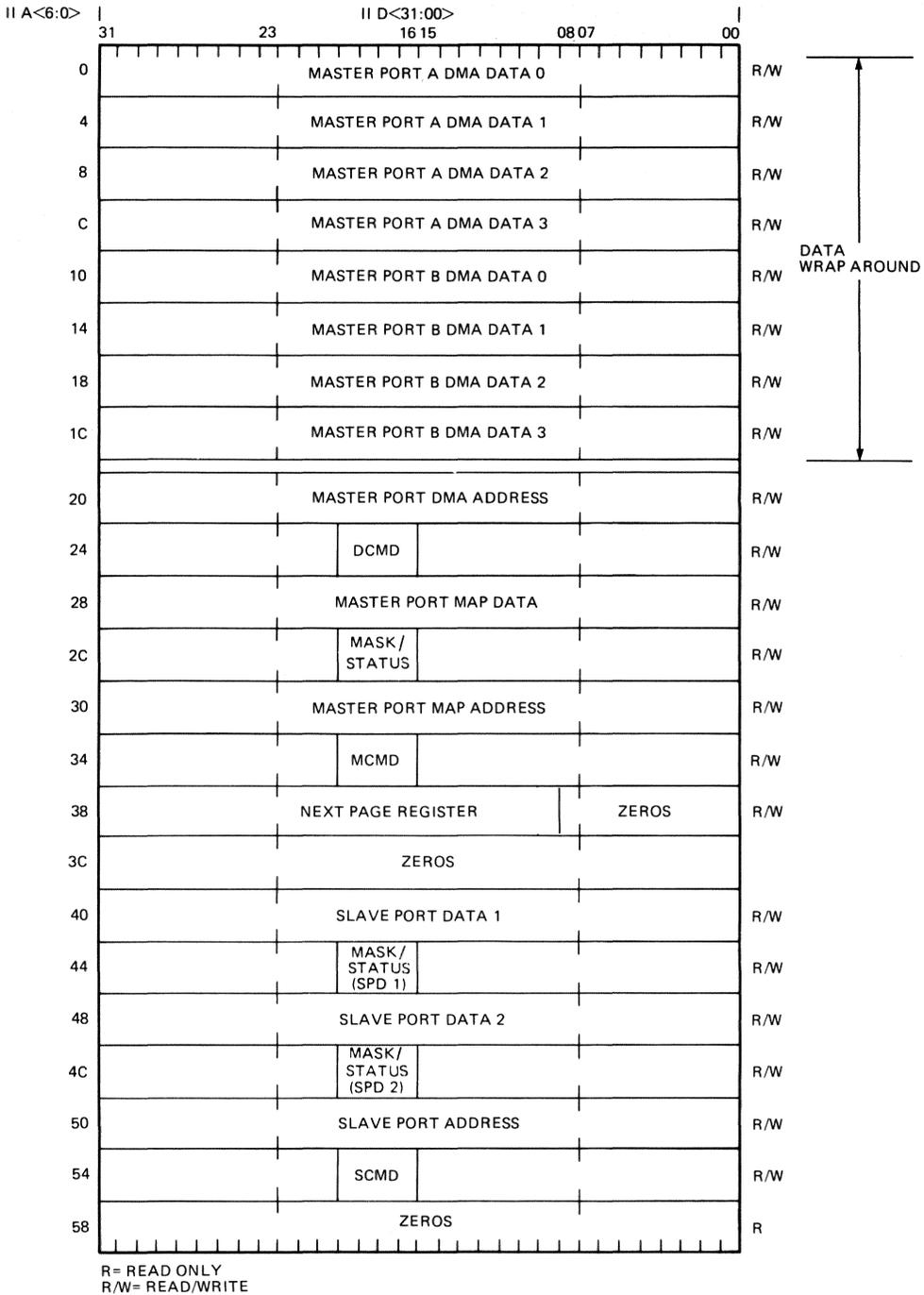
Figure 4 - VAXBI 78743 II Bus Interface Register Memory Map
