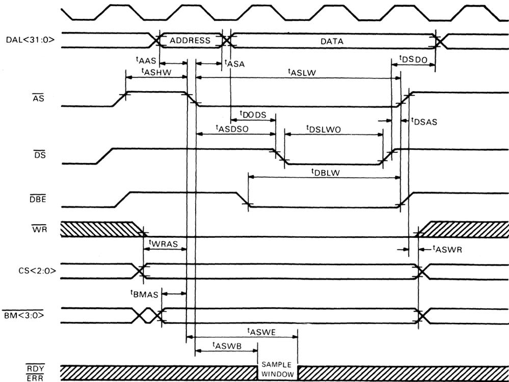
Figure 31 • MicroVAX 78532 MicroVAX Bus Master Write Cycle Timing
