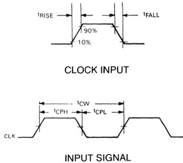
Figure 16 • MicroVAX 78516 Input and Clock Signal Timing
