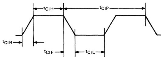
Figure 38 • MicroVAX 78032 CLK1 Timing Waveform
