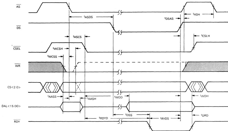
Figure 18 • MicroVAX 78516 Register Write Cycle Timing
