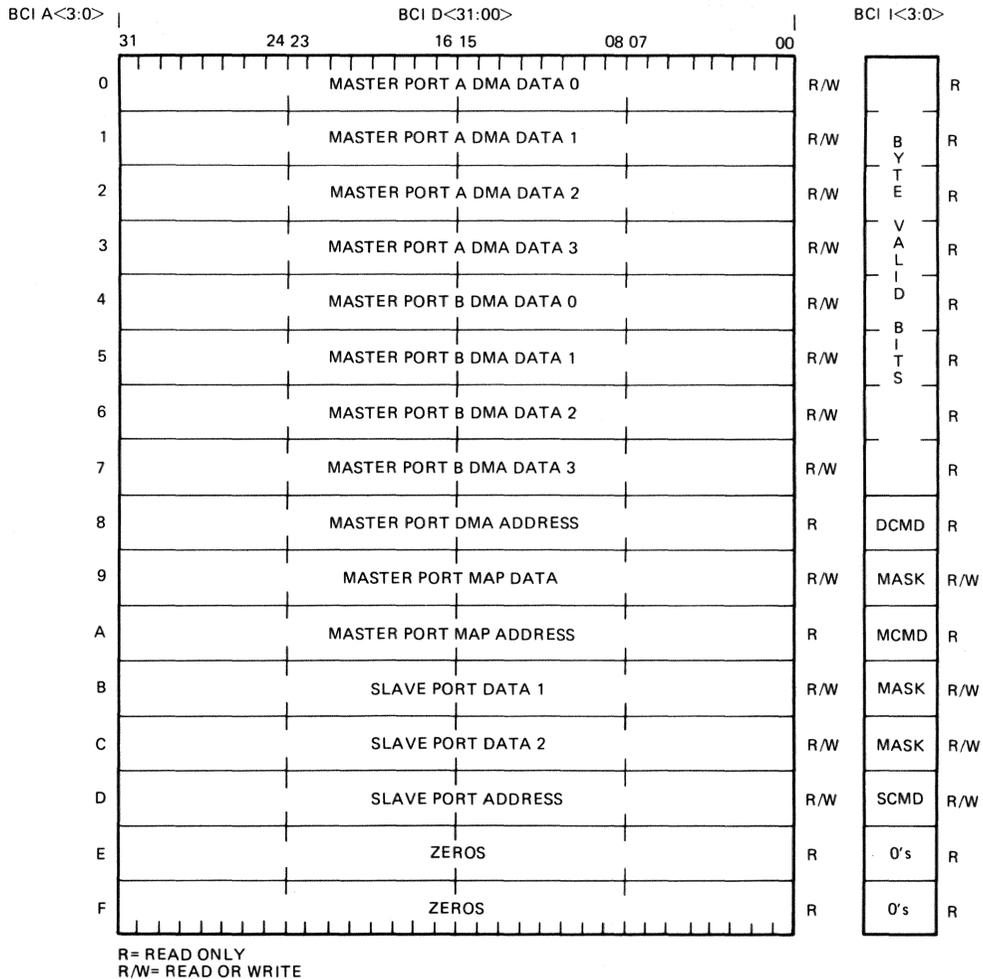
Figure 5 • VAXBI 78743 BCI Bus Interface Register Memory Map
