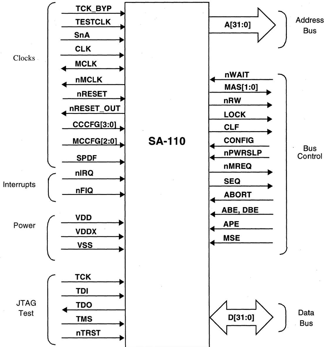
Figure 2: Functional Diagram
