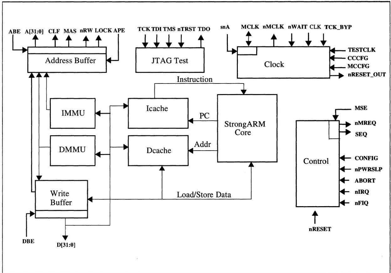
Figure 1: SA-110 Block Diagram
