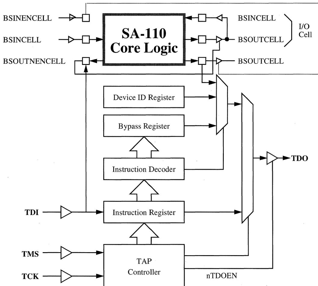
Figure 10: Boundary Scan Block Diagram
