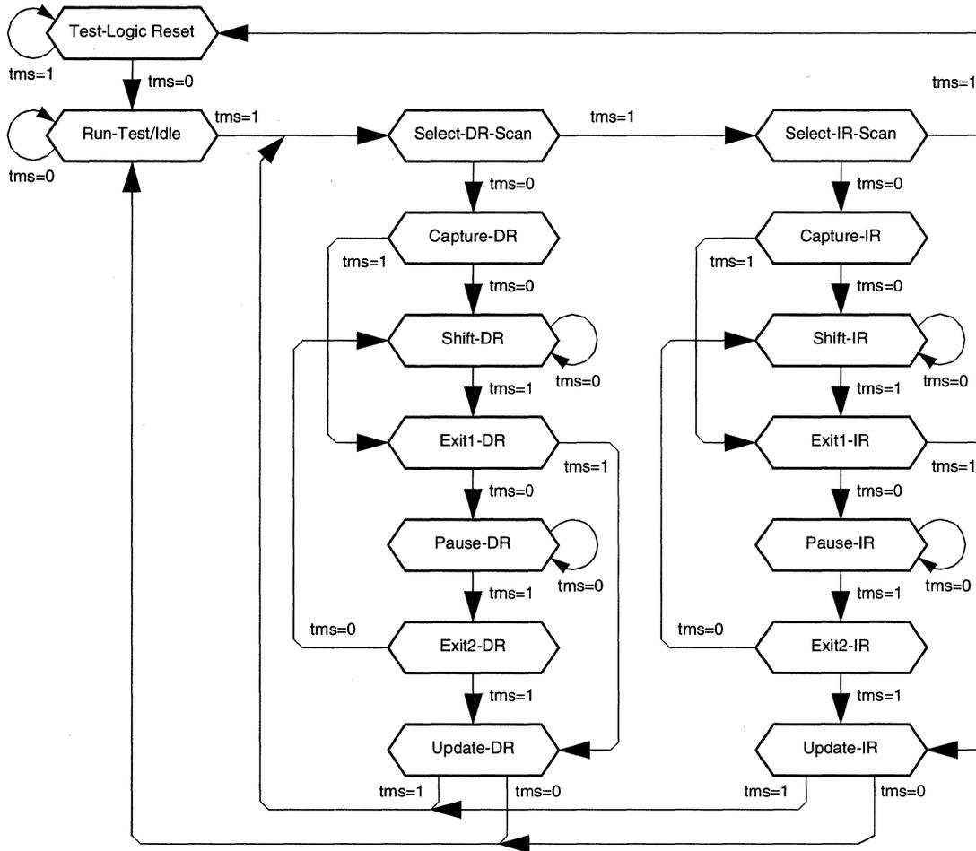
Figure 9: Test Access Port (TAP) Controller State Transitions
