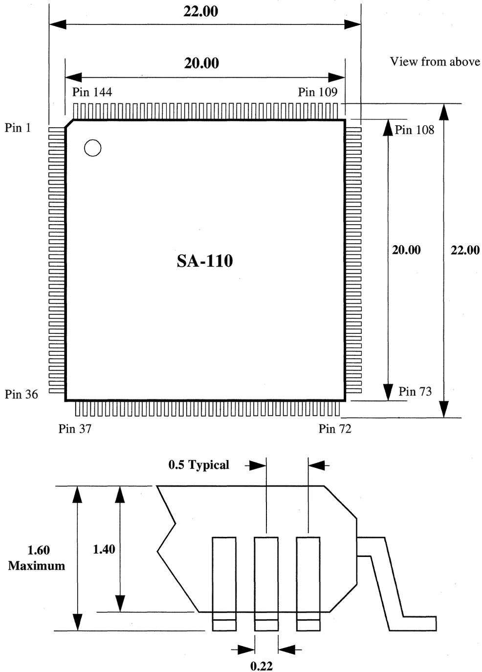
Figure 17: SA-110 144-Pin TQFP Mechanical Dimensions in mm
