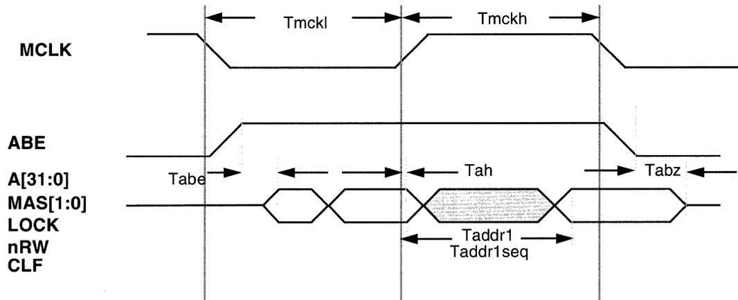
Figure 16: SA-110 Address Timing with APE=HIGH
