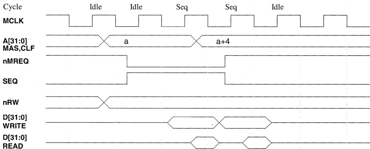
Figure 4: Sequential Read or Write (Two Word)
