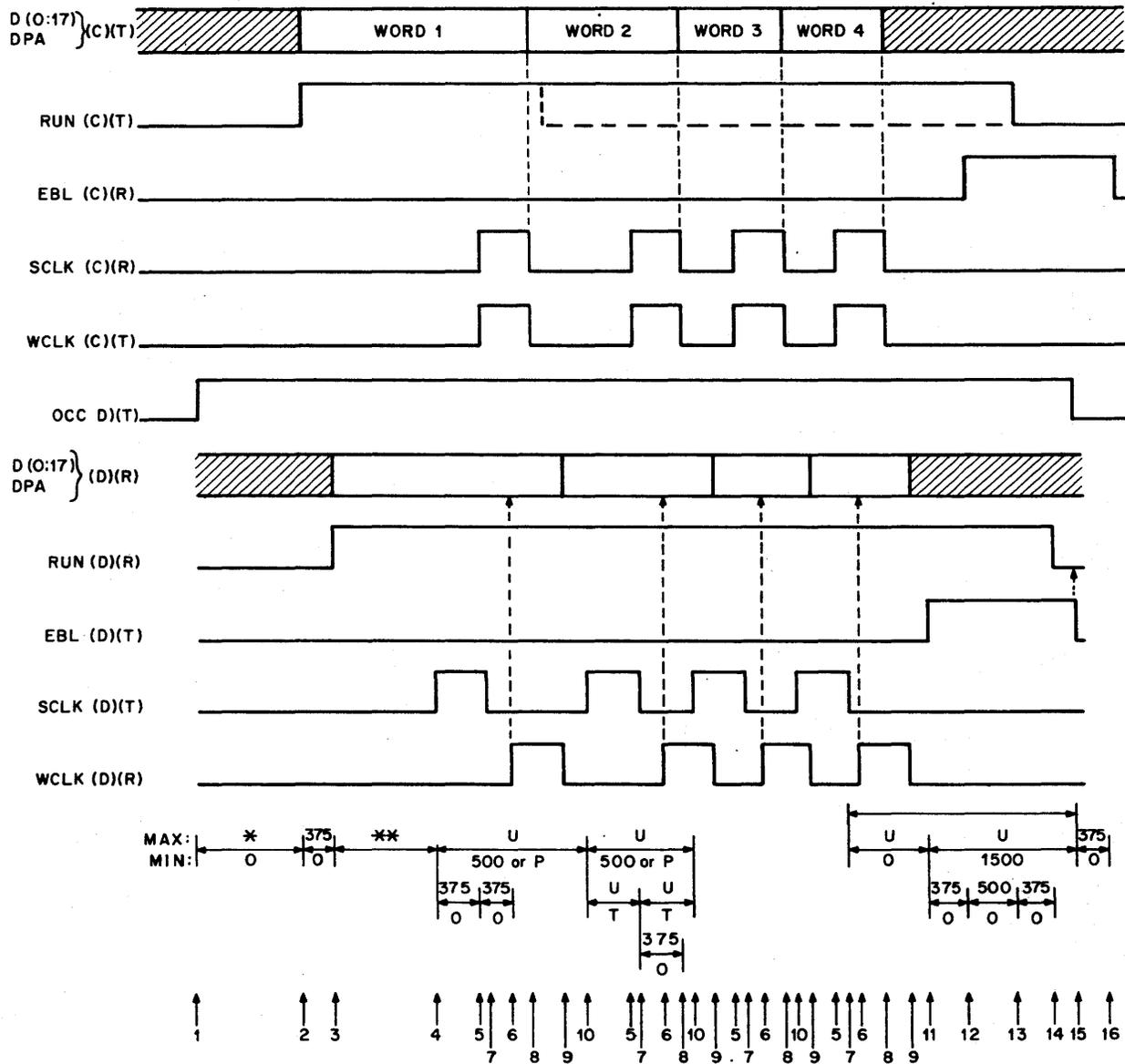
(C) = AT THE CONTROLLER (T) = TRANSMITTING \* 100 MICROSEC. MAX.
