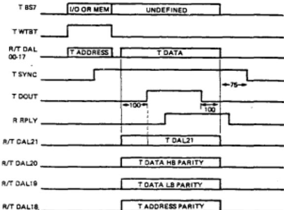
Figure A-2. DATO Timing Diagram at Master (with Parity)
