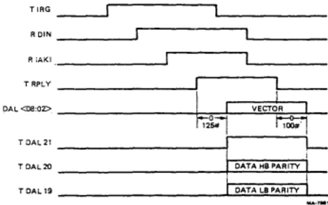
Figure A-3. Interrupt Request Timing Diagram at Slave (with Parity)
