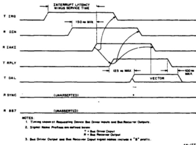
Figure 11. Interrupt Transaction Timing
