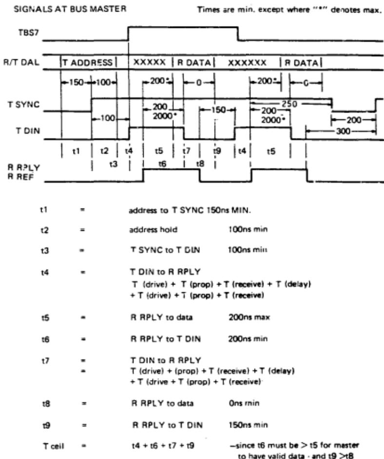
Figure 9. DATBI Bus Cycle Timing
