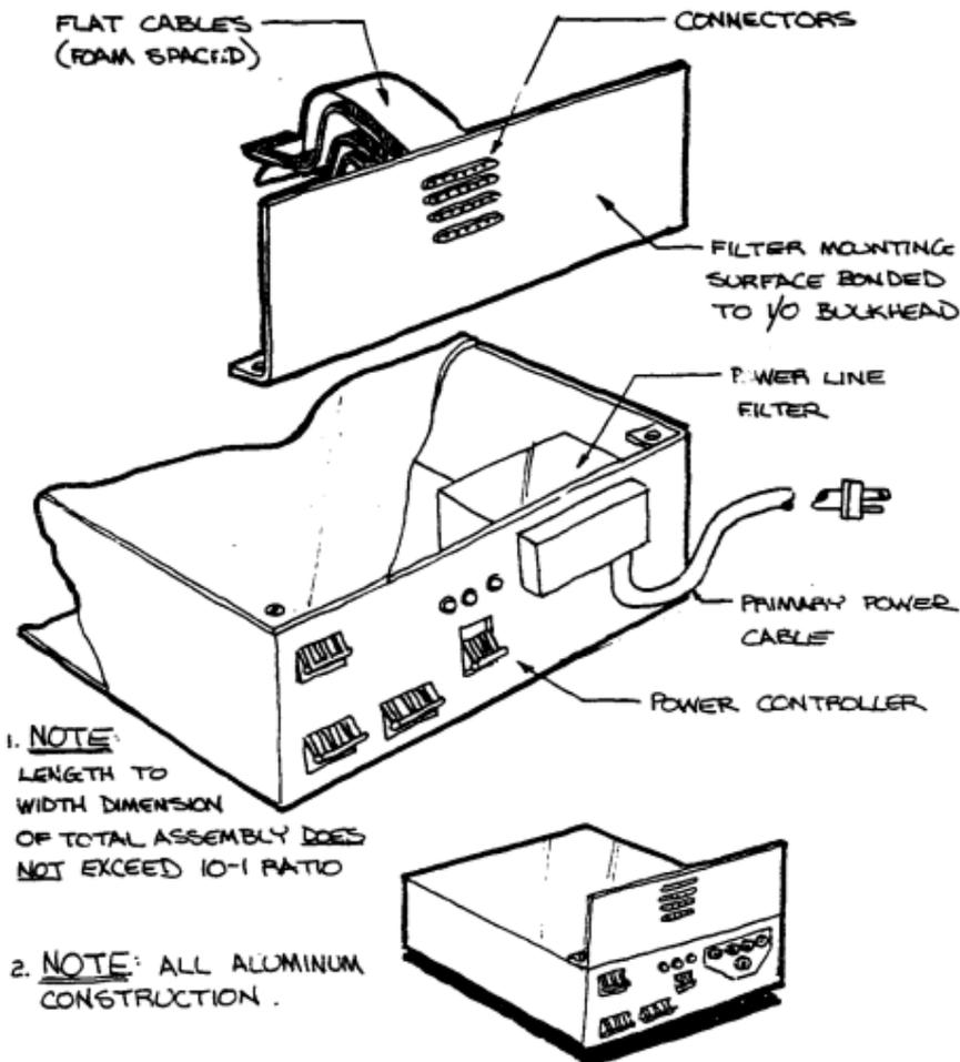
Figure 6 I/O Interface Bulkhead
