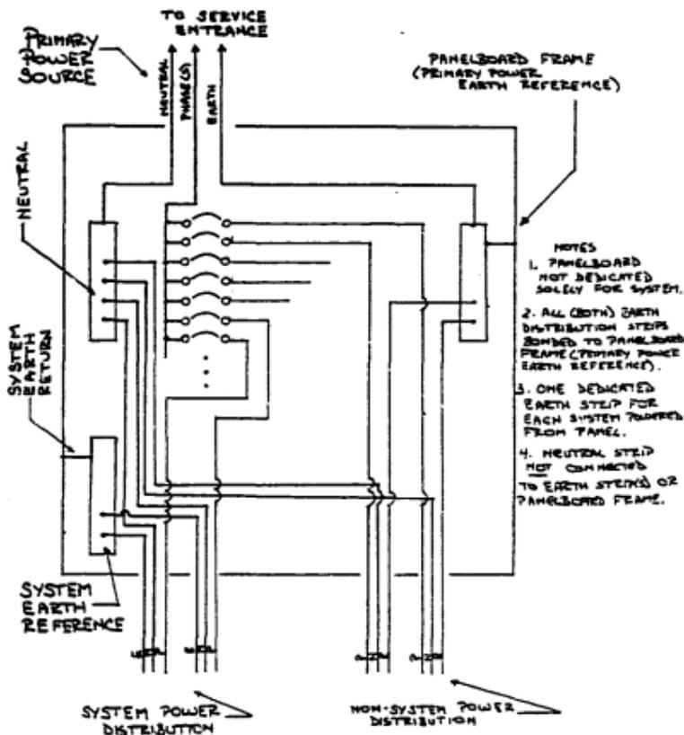
Figure 3 System Distribution Panel (medium/large system)
