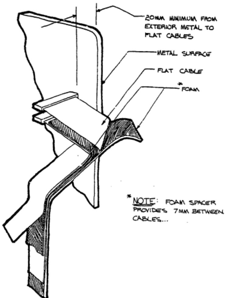
Figure 8 Flat Cable Stacking
