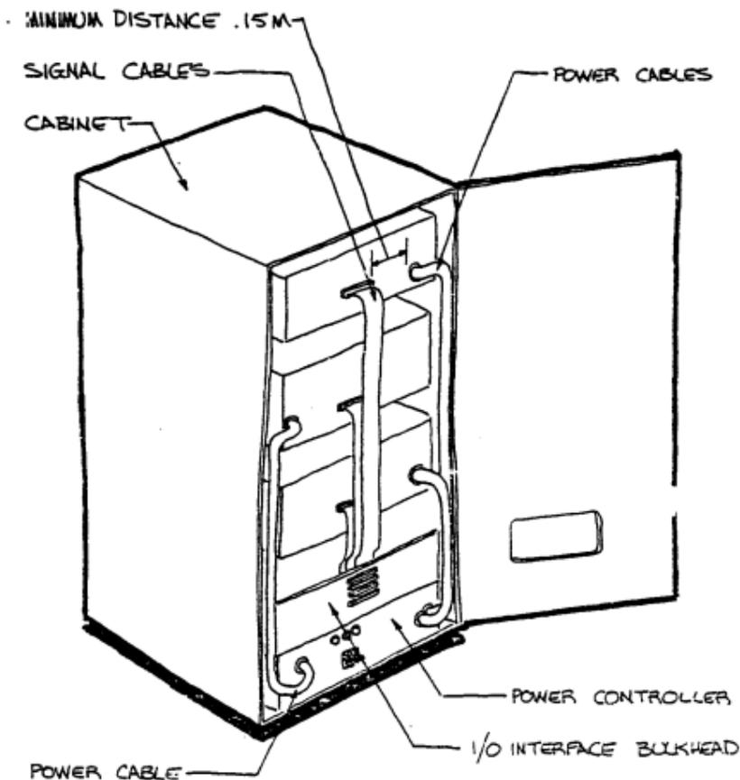
Figure 9 Cabinet Cable Configuration
