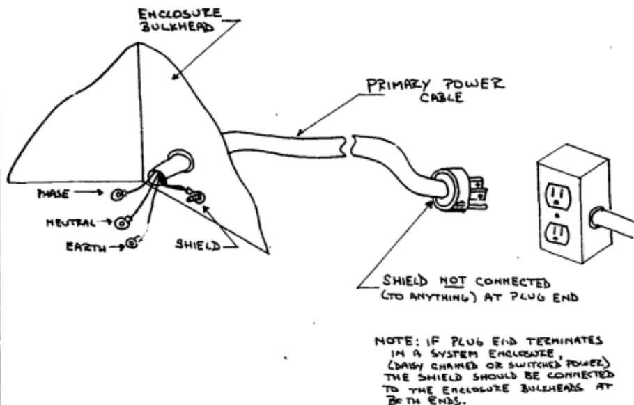
Figure 13 Primary Power Cable Shielding
