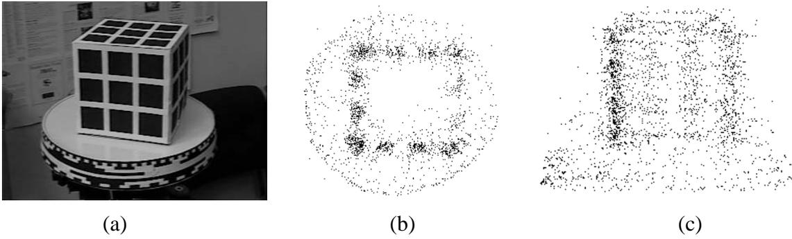
Figure 6: Rotating cube (complete rotation, 48 frames): (a) first frame, (b) top view of recovered 3-D points (2500 points), (c) side view of 3-D points.
