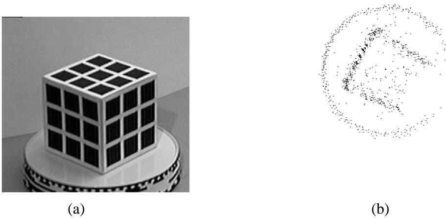
Figure 7: Rotating cube (not complete rotation): (a) First frame of the sequence, and (b) Top view of recovered points for the cube scene using 96 frames and known camera parameters. (From [25].) Notice the pinching effect.
