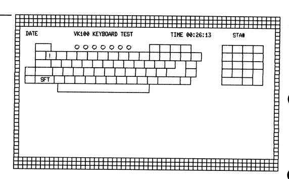
During this test, the Exerciser sometimes requires that you press two keys at the same time. When this is the case, both keys are blinking. For example, the first row of characters to be entered requires that you press the SHIFT key and the first row of keys on the keypad at the same time; however, you enter the next row of characters by pressing a single key.
