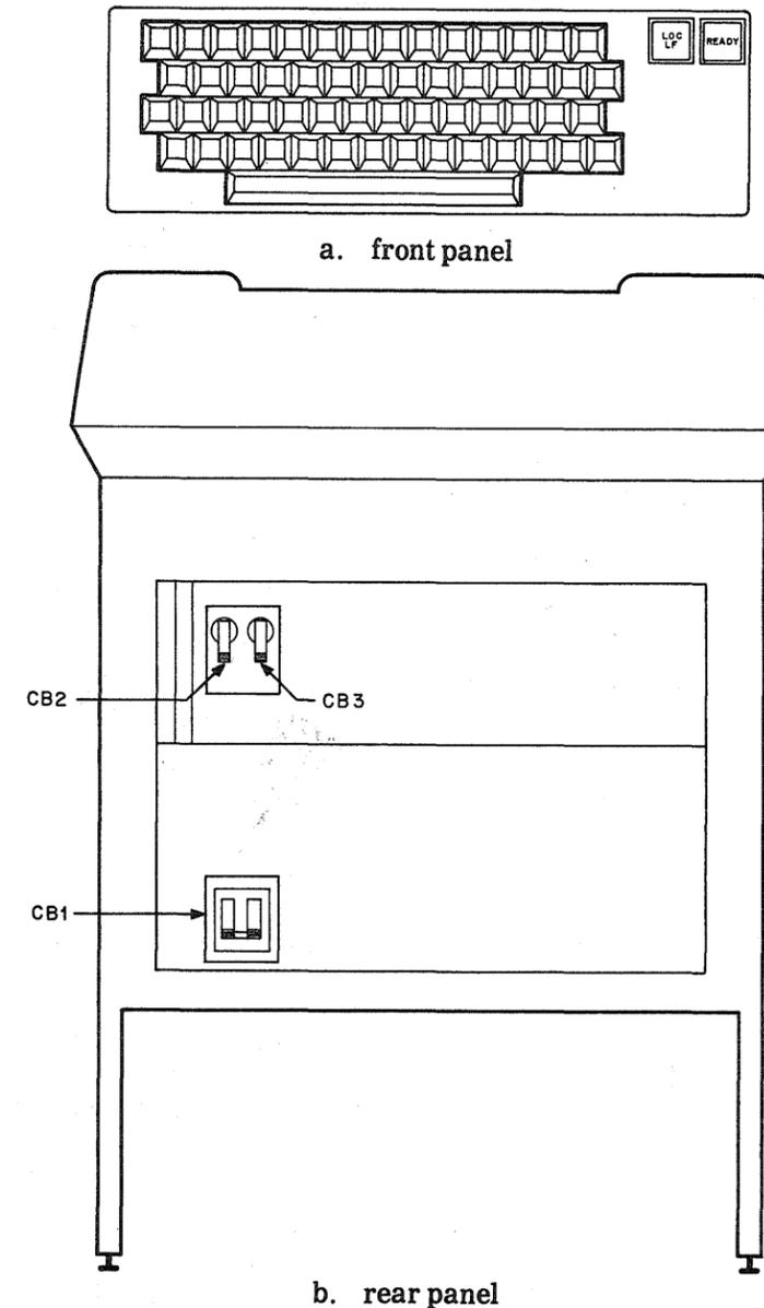
Figure 3-1 DECwriter Controls and Indicators
