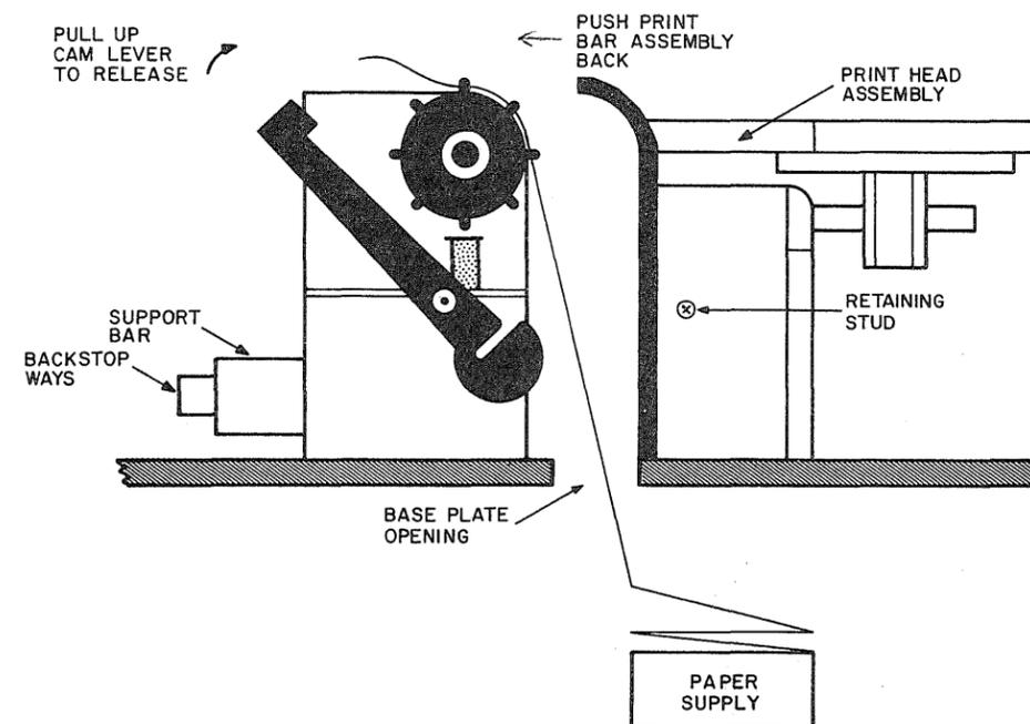
Figure 3-2 Loading Paper into LA30 DECwriter
