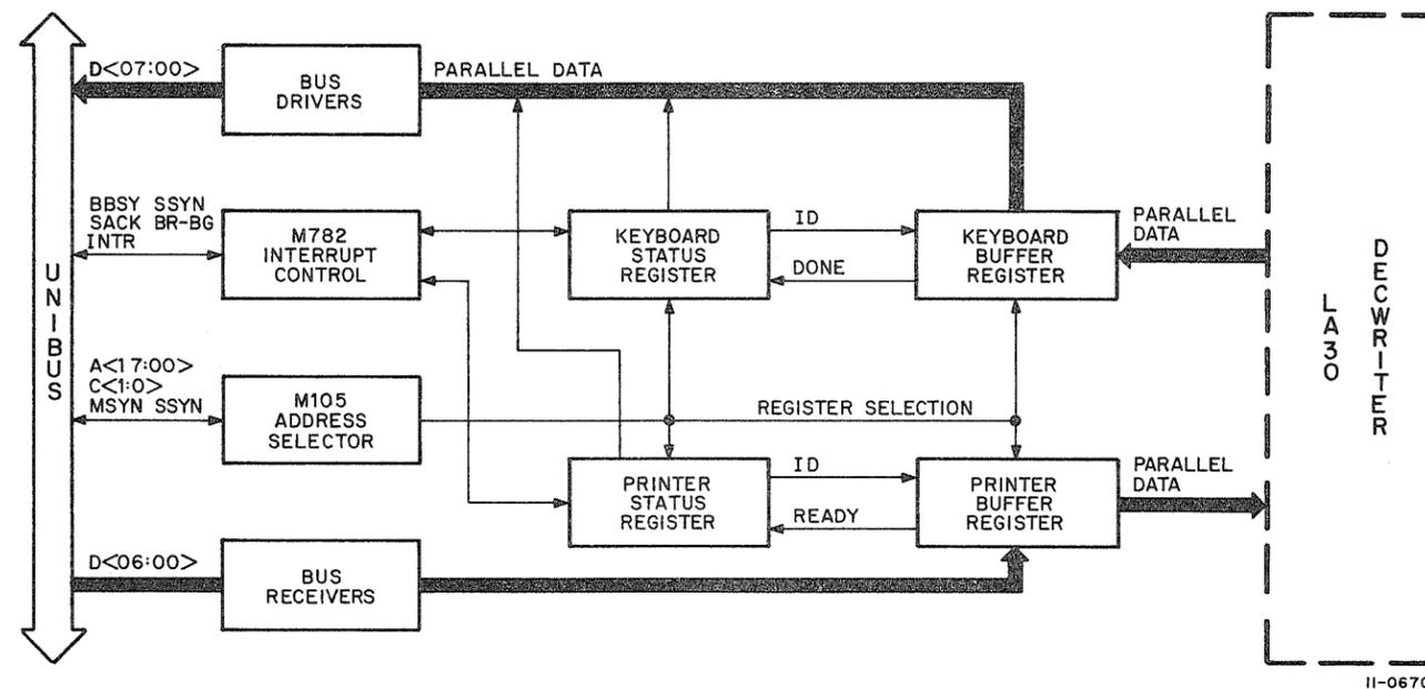
Figure 2-1 LC11 Controller—Simplified Block Diagram
