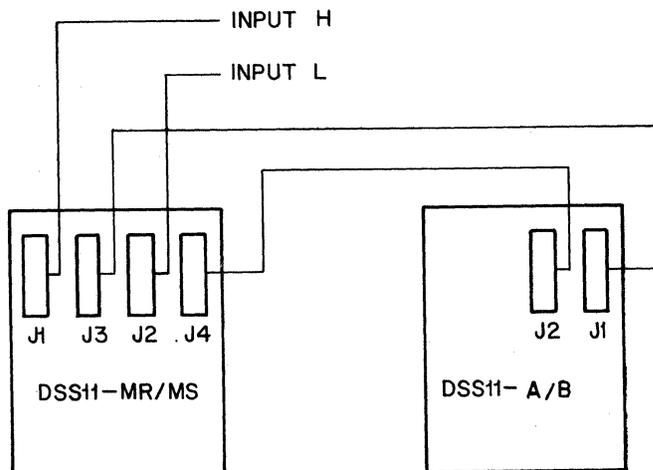
Figure 2-10 User Cabling Using DSS11-MR or DSS11-MS
