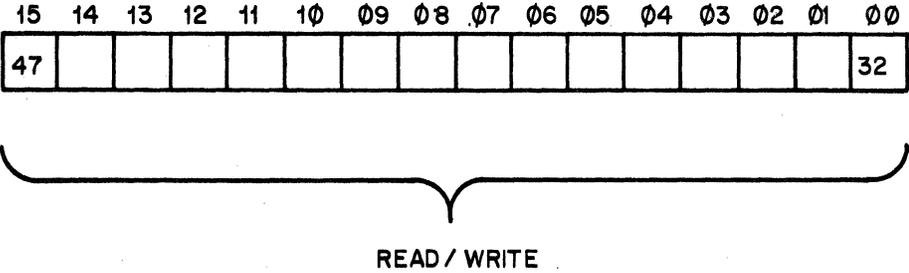
Figure 3-4 Third Data Register Out (RG3-DRS)
