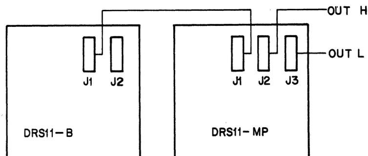
Figure 2-5 DRS11-MP Connected To User Equipment
