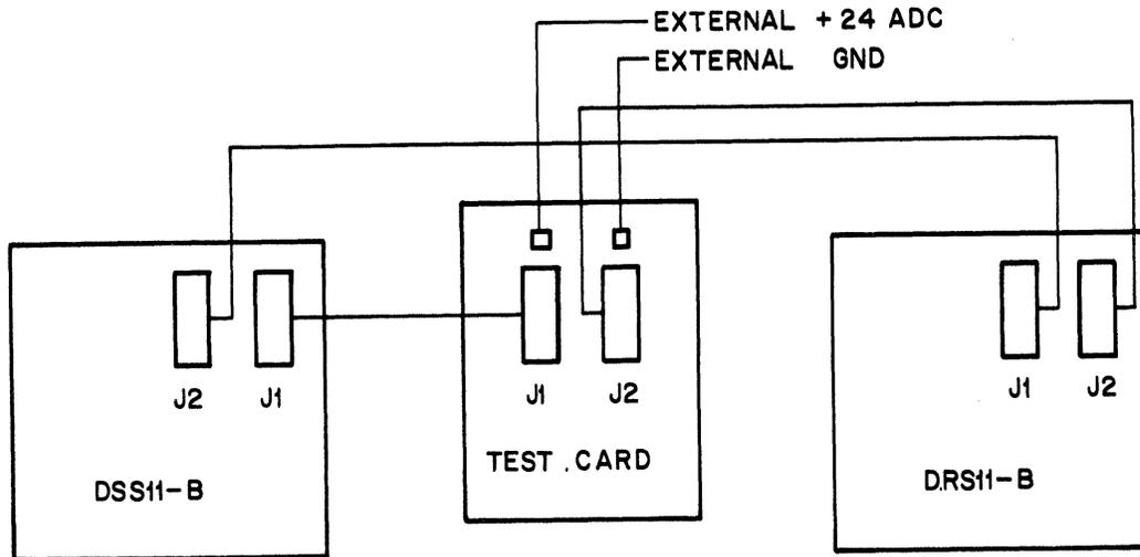
Figure 2-4 DRS11-B Looped With DSS11-B
