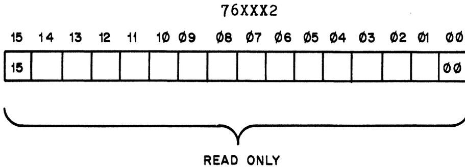
Figure 3-5 First Data Register In (RG1-DSS)
