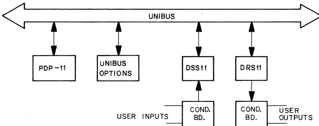
Figure 1-1 Typical DRS11/DSS11 Configuration
