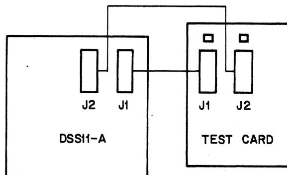
Figure 2-1 DSS11-A Stand Alone Test 6
