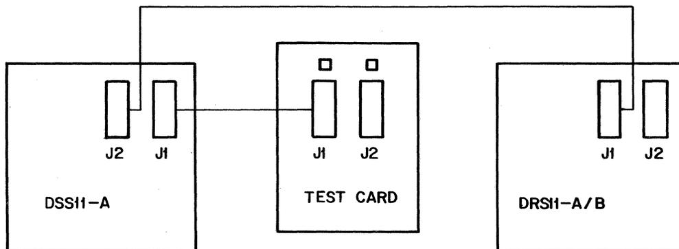
Figure 2-3 DRS11-A/B Looped With DSS11-A
