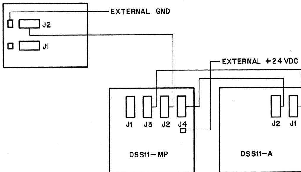
Figure 2-8 Cabling For Test 6 Static Patterns
