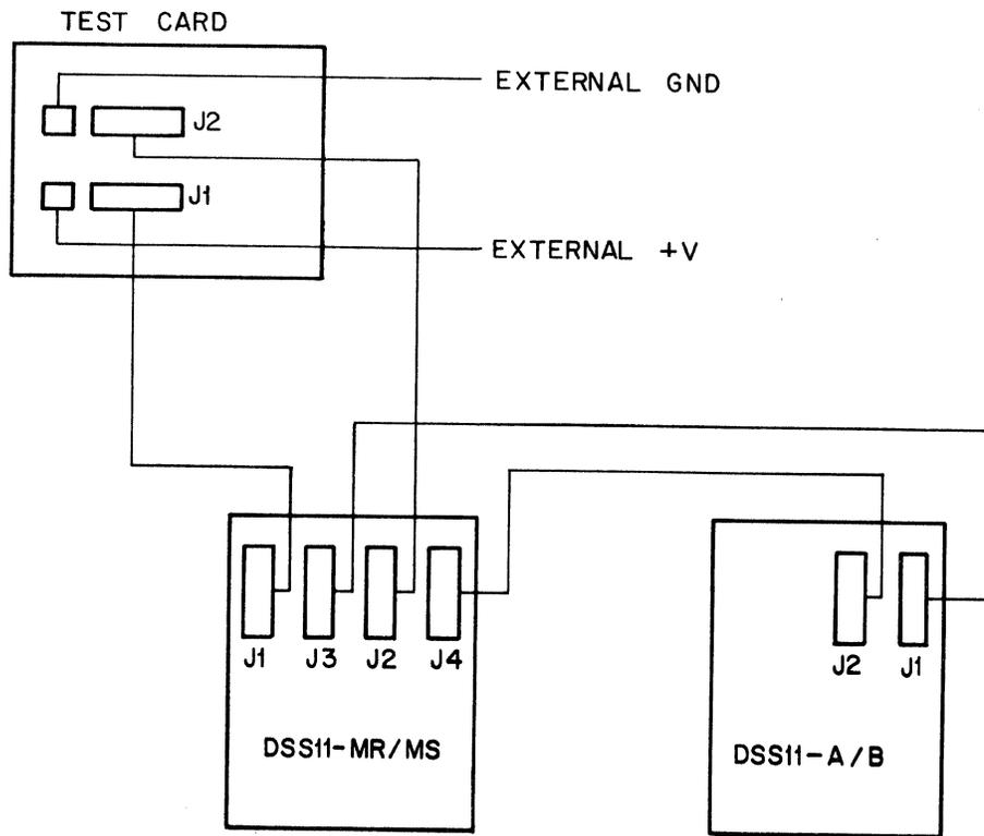
Figure 2-11 Static Pattern Test Cabling
