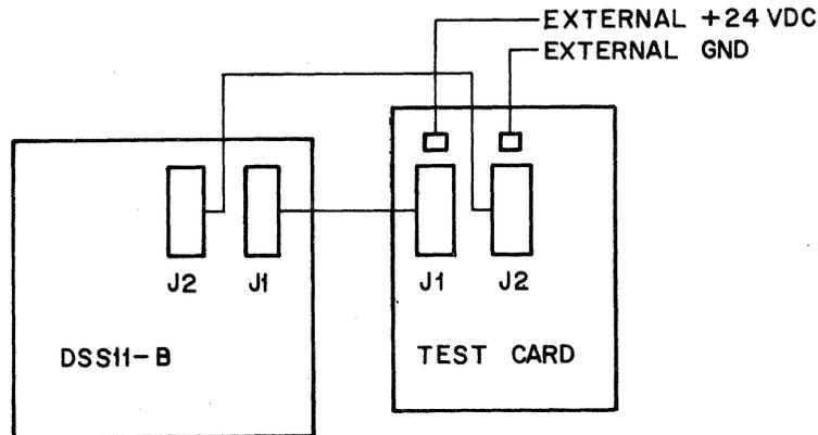
Figure 2-2 DSS11-B Stand Alone Test 6
