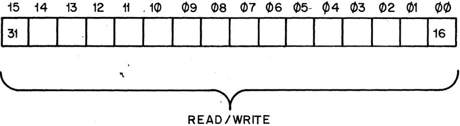
Figure 3-3 Second Data register Out (RG2-DRS)
