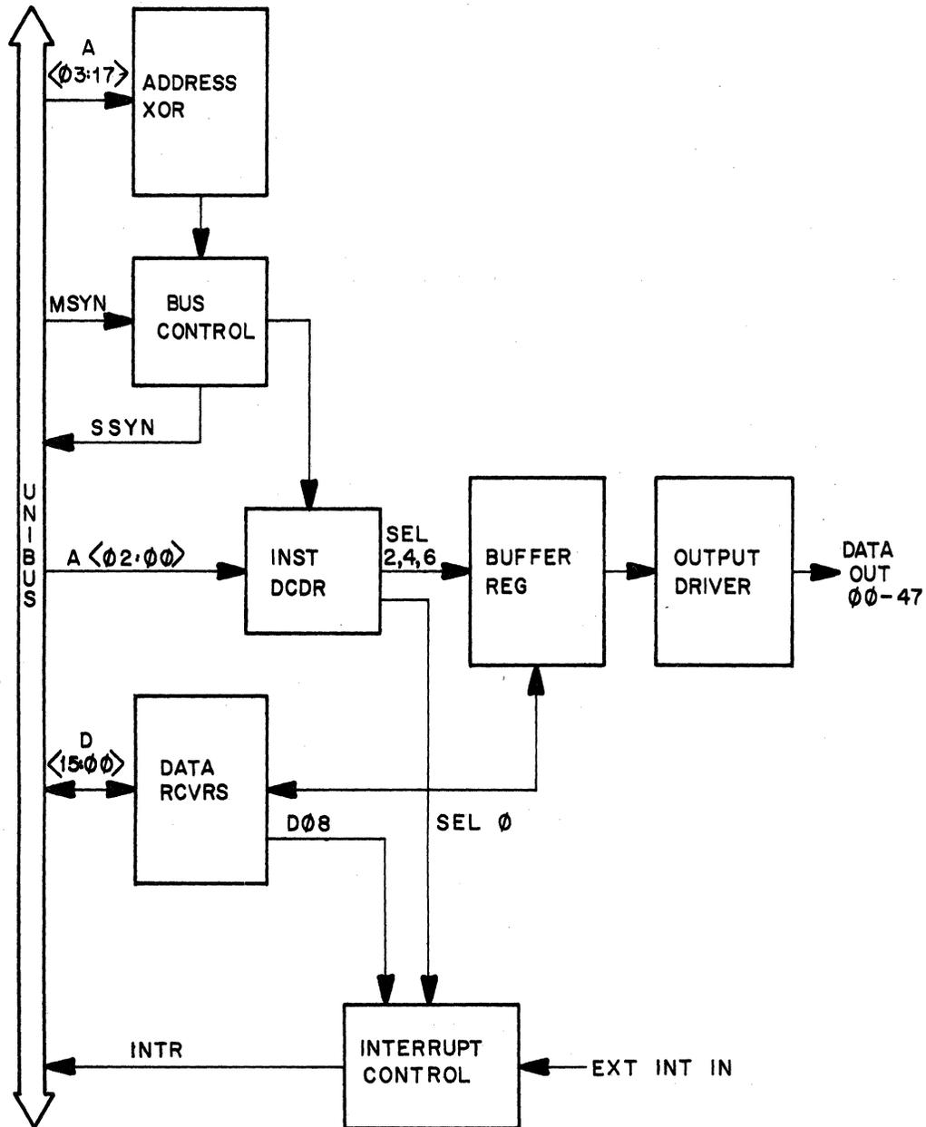
Figure 4-1 DRS11-A/B Block Diagram
