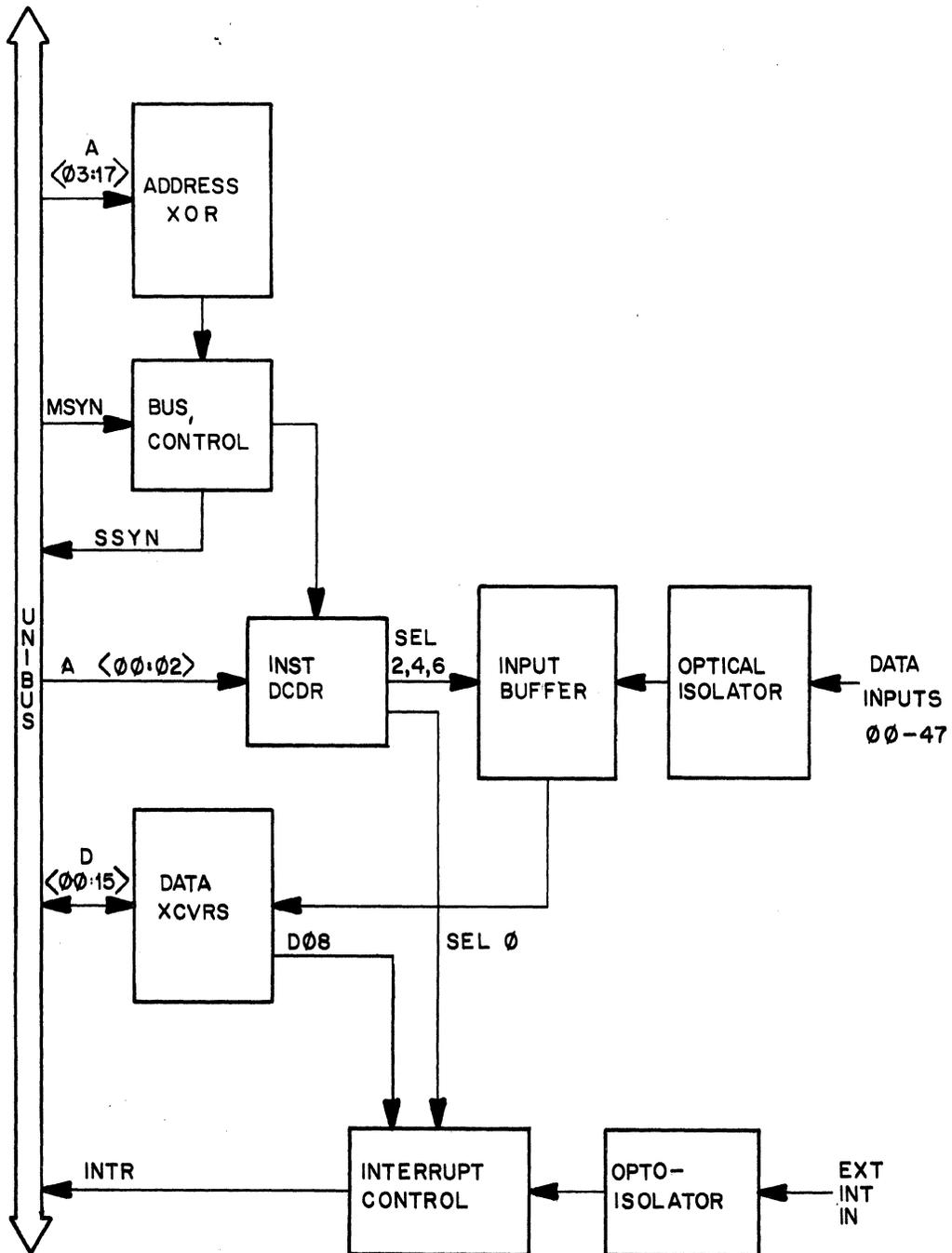
Figure 4-2 DSS11-A/B Block Diagram
