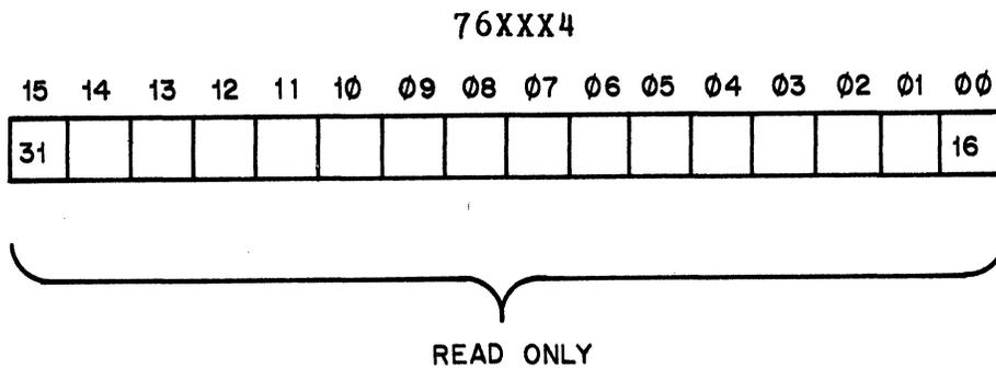
Figure 3-6 Second Data Register In (RG2-DSS)
