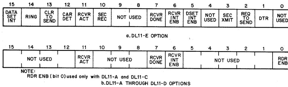
Figure 4-1 Receiver Status Register (RCSR) – Bit Assignments
