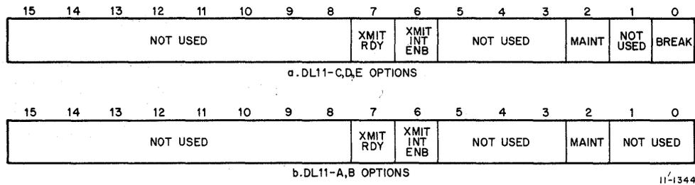
Figure 4-3 Transmitter Status Register (XCSR) – Bit Assignments
