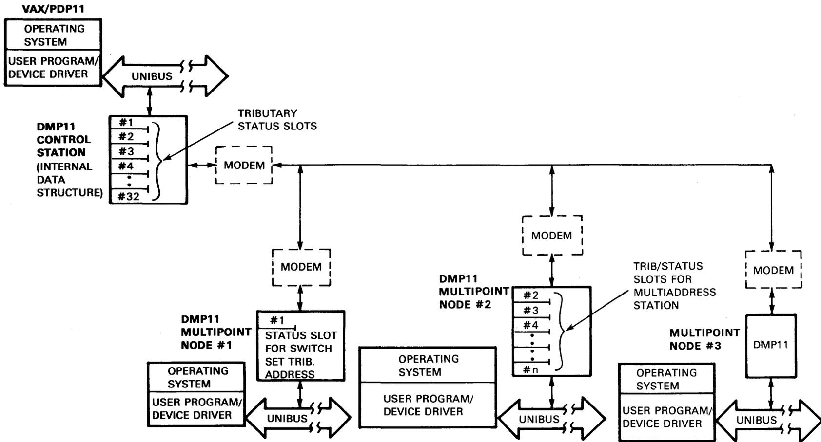
Figure 1-4 Block Diagram of a Multipoint Network with Multiple Tributary Addresses
