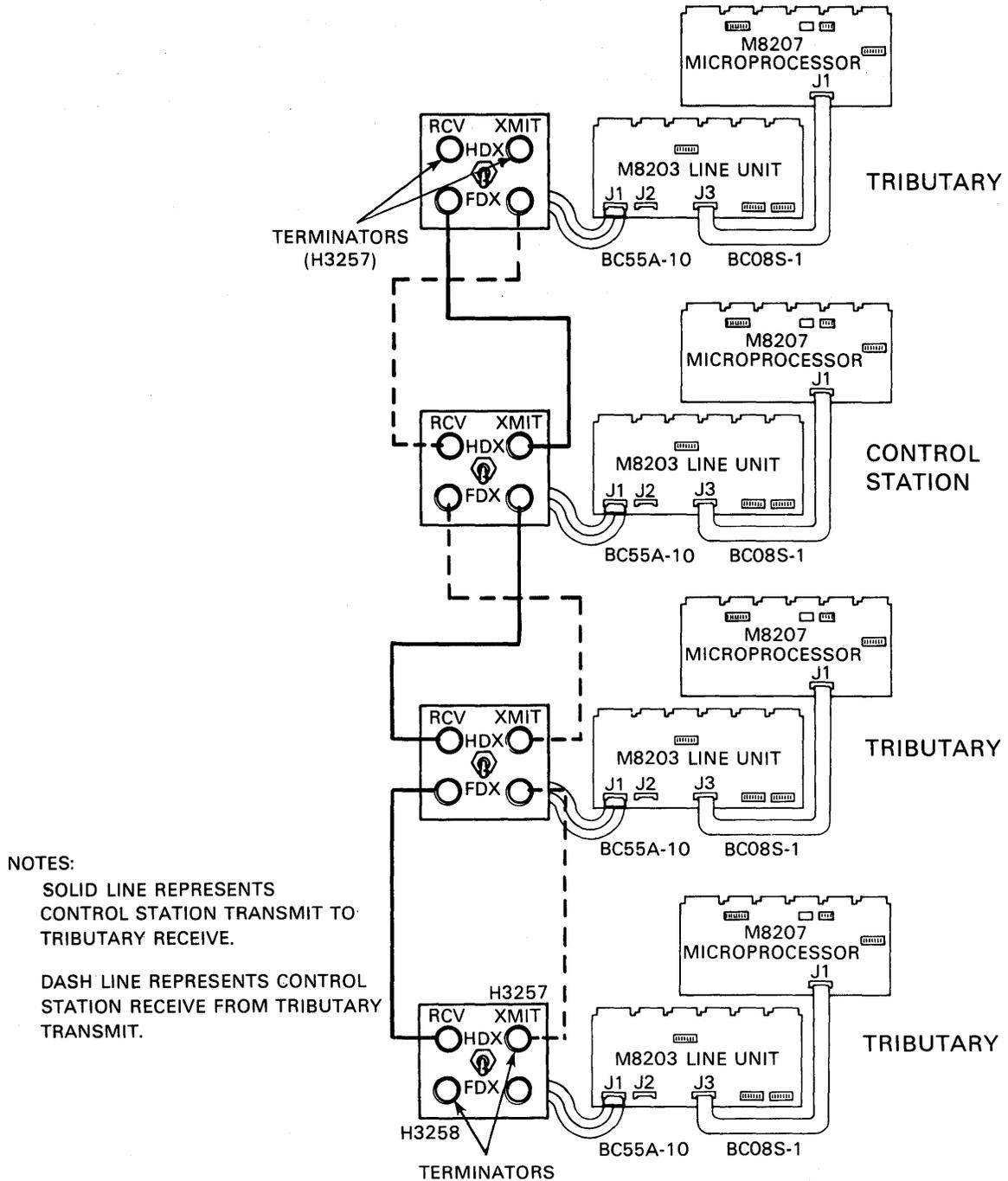
SINCE THE CONTROL STATION IS NOT AN END MODE, THERE IS NEED TO TERMINATE TWO SETS OF TRANSMIT LINES FROM THE CONTROL STATION, ADDITIONALLY BOTH ENDS OF THE TRANSMIT LINE FROM THE TRIBUTARIES
