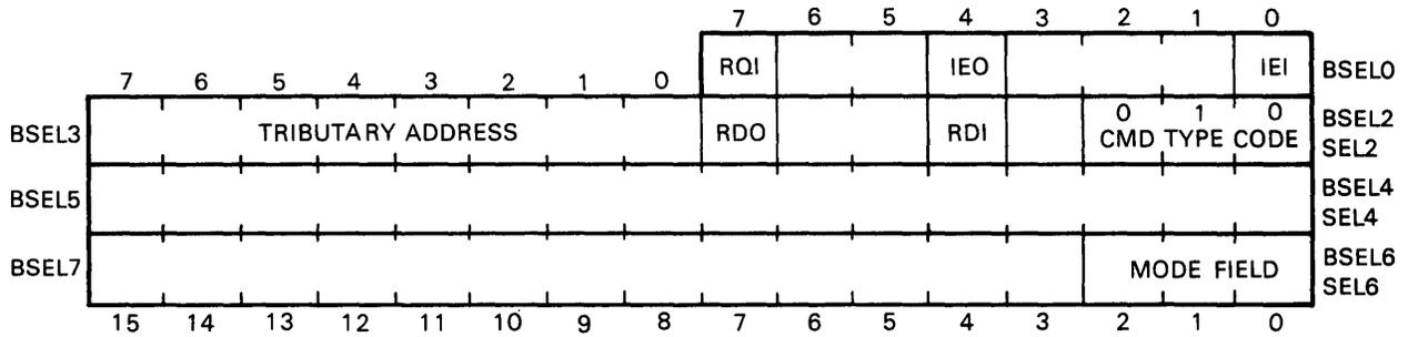
Figure 3-5 Mode Definition Command Format
