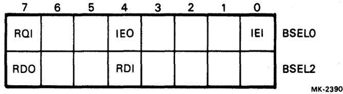
Figure 4-1 CSR Interface Control Bits
