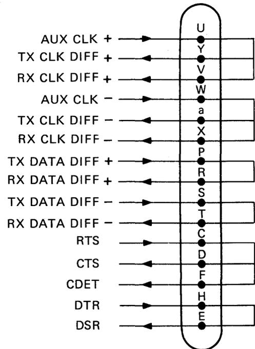
Figure 2-7 DMP11 Turnaround Test Connectors (Sheet 1 of 4)
