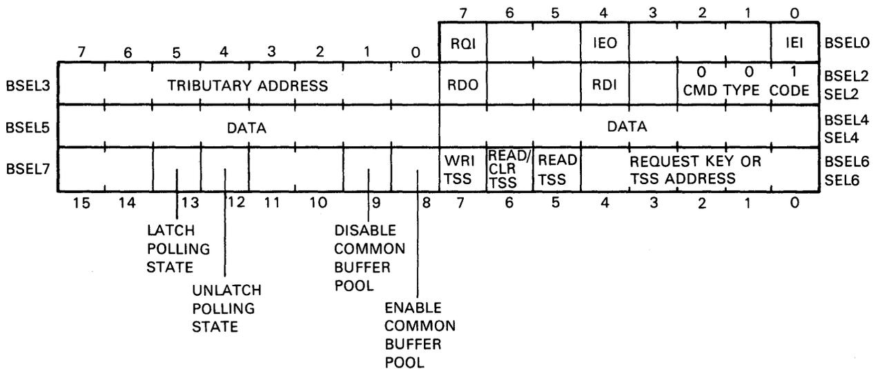
Figure 3-6 Control Command Format
