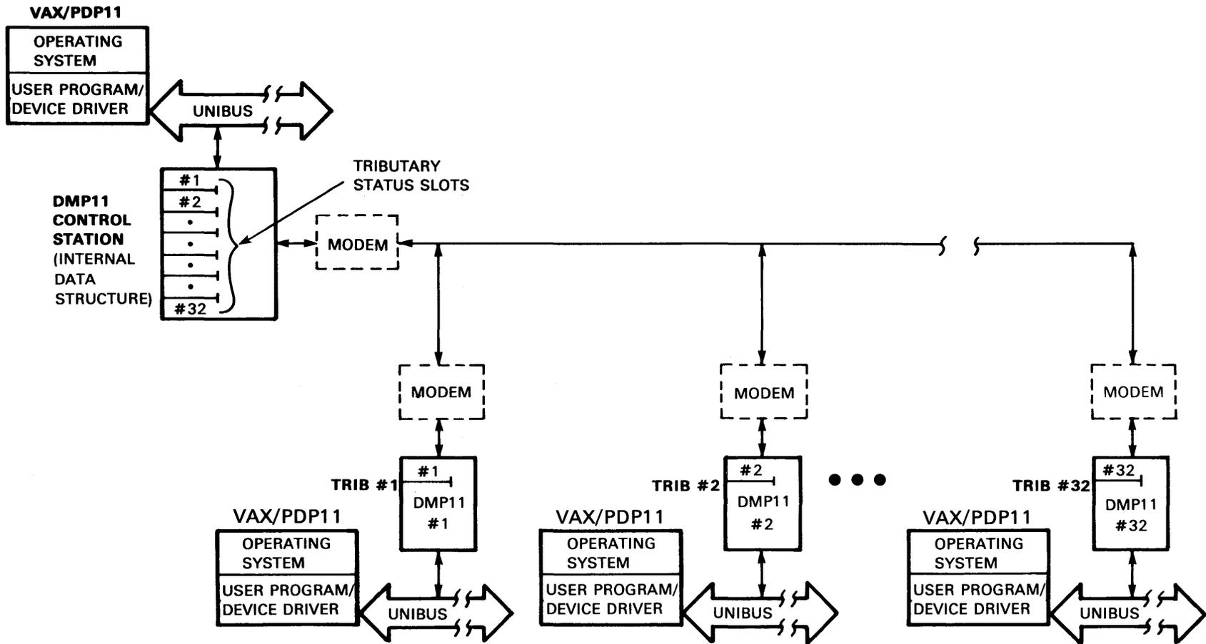
Figure 1-3 Block Diagram of a Multipoint Network with Single Assigned Addresses
