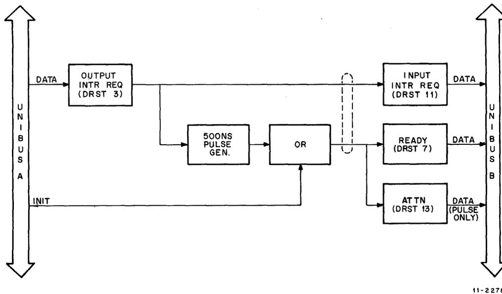
Figure C-3 Cross-Interrupt Block Diagram
