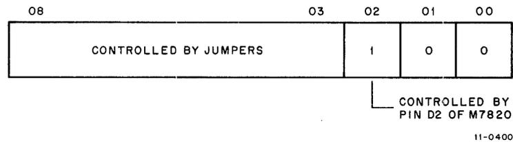
Vector address bits (08:03) are determined by jumpers on the M7821 (a jumper “in” indicates a 1 for the M7821 and for the M7820 in earlier models a jumper “in” indicates a 0). Bit 02 of the address is controlled by pin D2 of the M7821; because this input is at a high level whenever the interrupt operation is occurring, bit 02 of the vector address will be a 1. Pin D2 can be rewired and a ground applied to it, thereby causing bit 02 of the address to be a 0.
