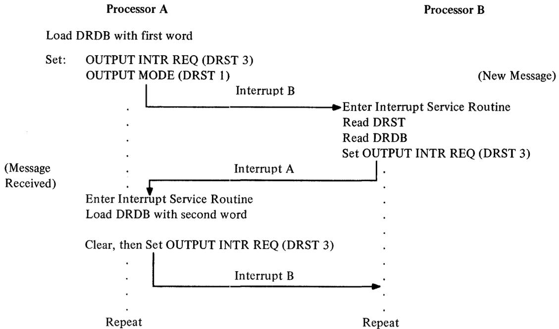
**C.3.5.2 Block Mode** – During block transfers under NPR control, DRDB temporarily stores the word read by the transmitter until it is written into memory by the receiver. Because this sequence of operations is transparent to the program, DRDB may *not* be used for Word mode transfers until the block transfer has been completed. If DRDB is loaded by the program during a block transfer, incorrect data may be transmitted between computers. DRDB is cleared by INIT.
