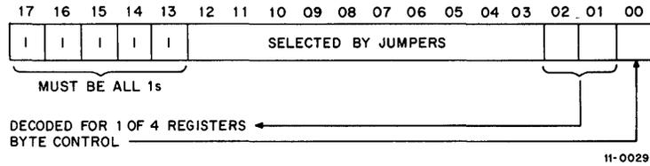
Figure 4-3 Interface Select Address Format
