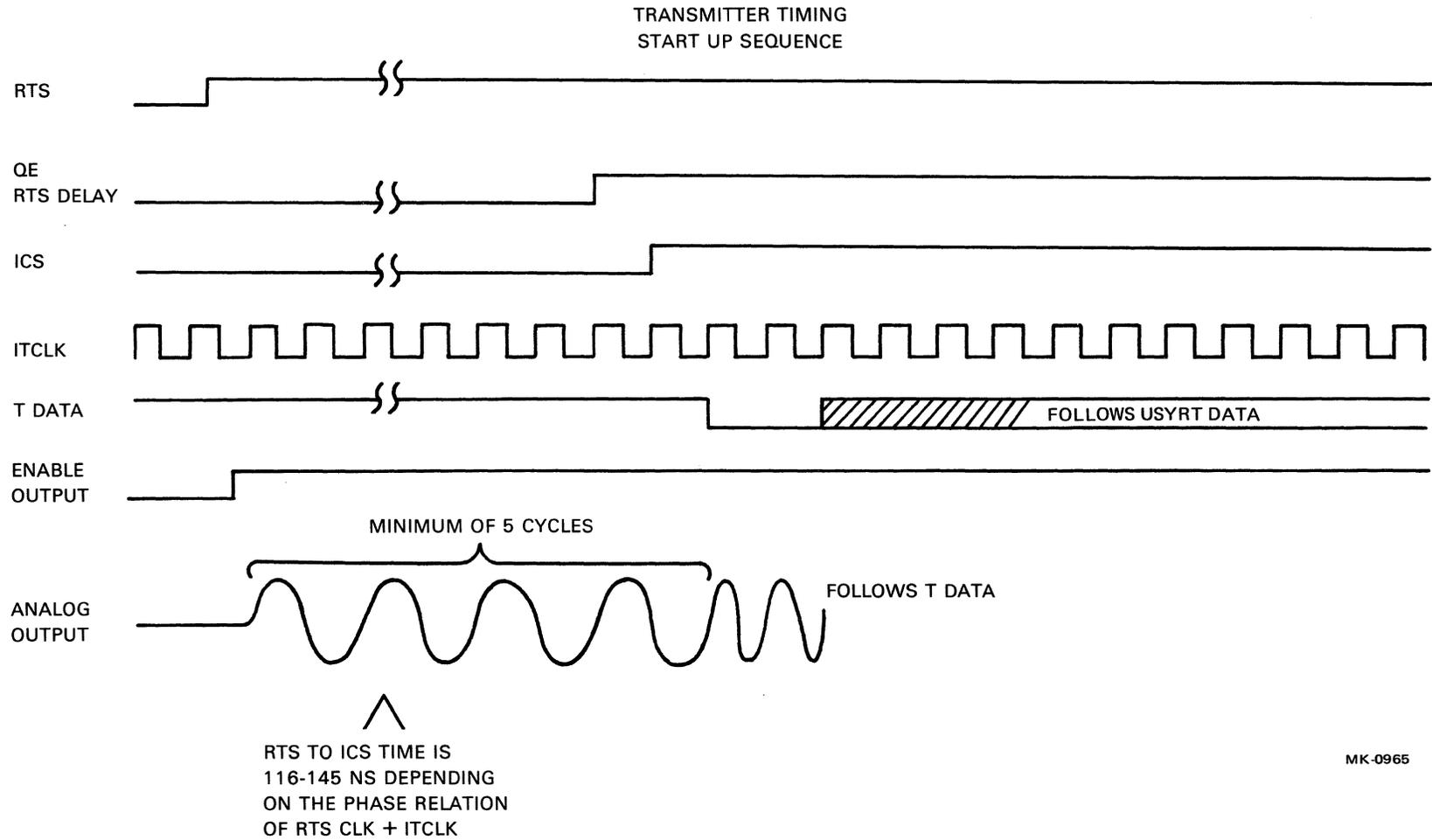
Figure 3-41 Modem Transmitter Timing Diagram - Start-Up
