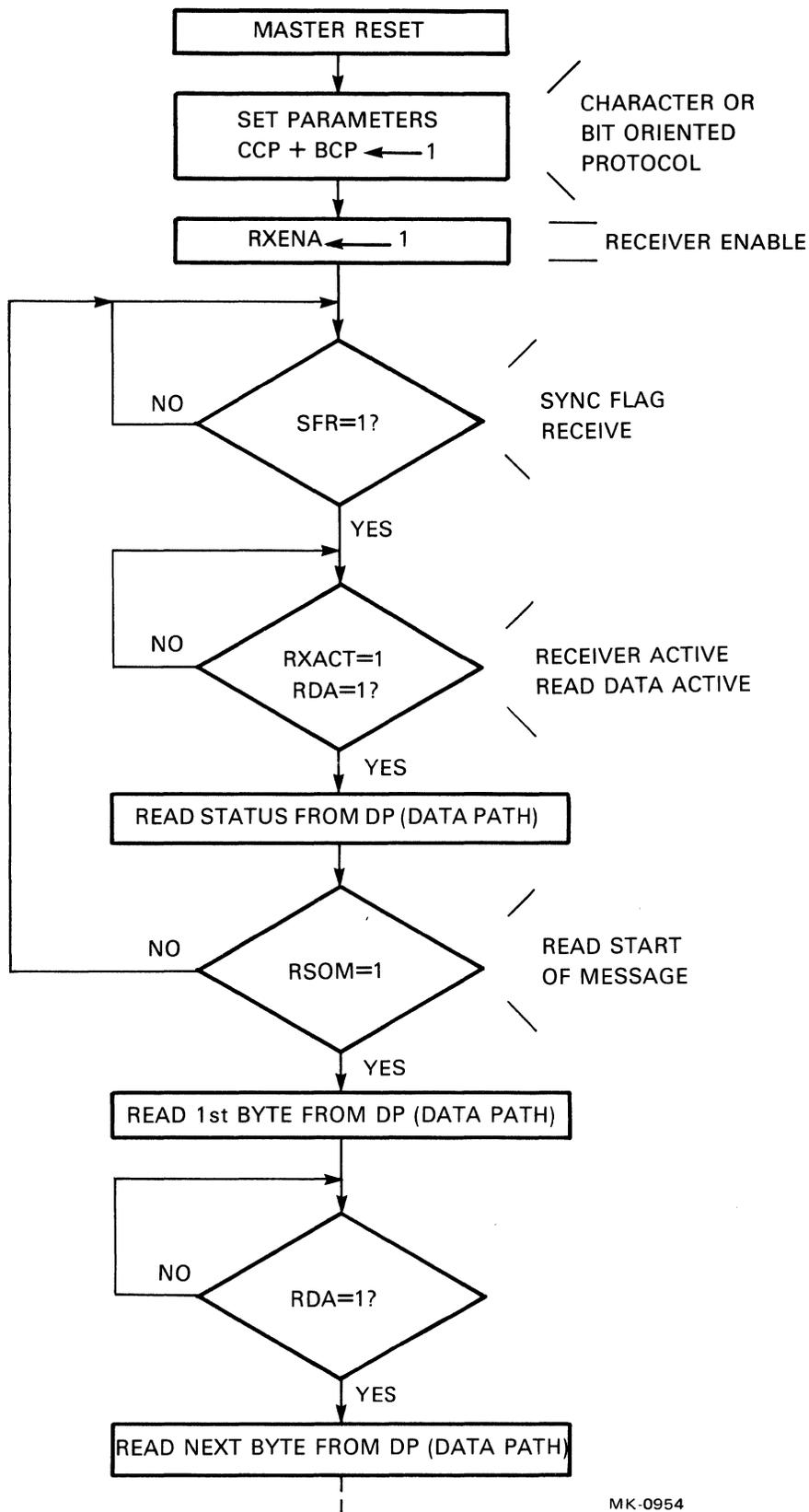
Figure 3-35 Typical Receive Sequence for the USYRT Character Oriented Protocol Flowchart
