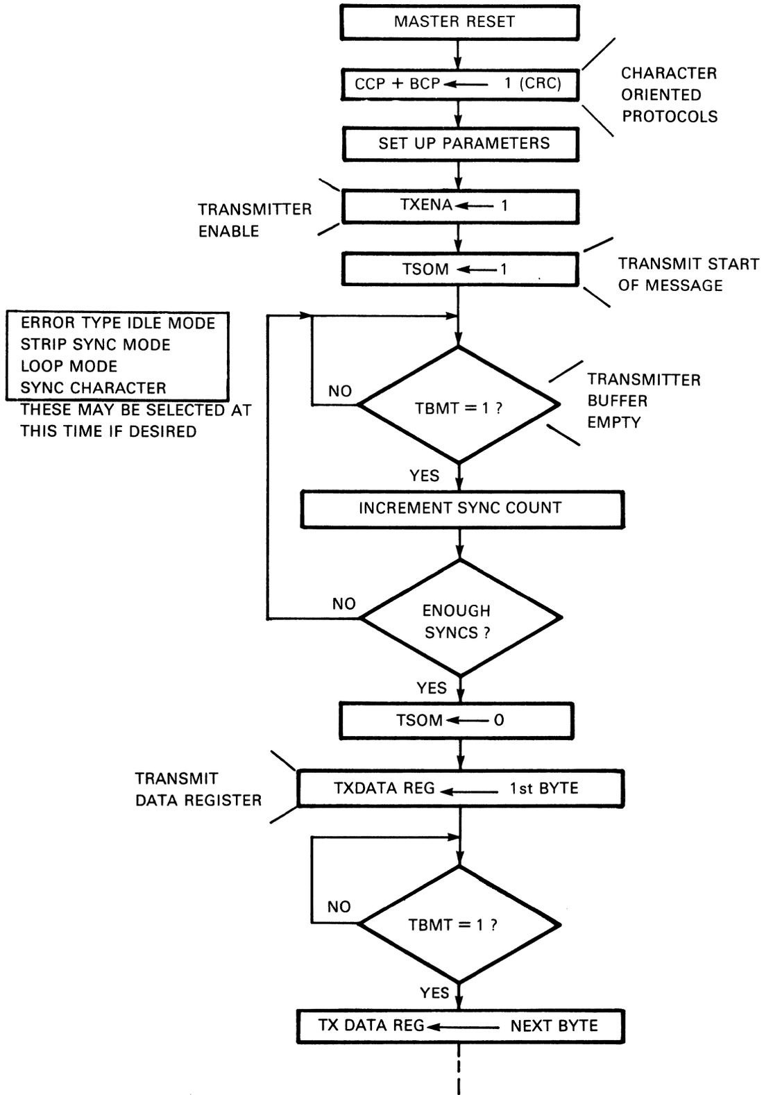
Figure 3-33 Typical Start Sequence for the USYRT Character Oriented Protocol Transmission Flowchart
