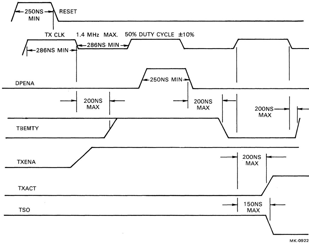
Figure C-4 Transmit Signal Timing Waveforms
