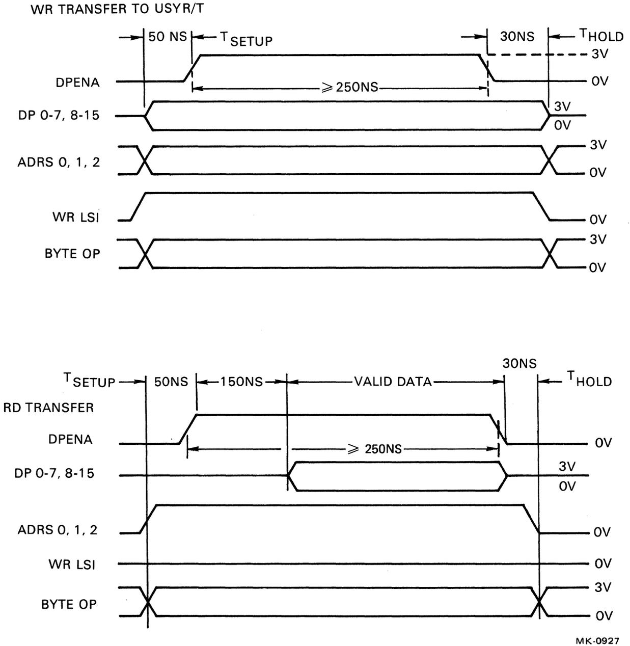
Figure C-5 Tri-State Output Waveforms
