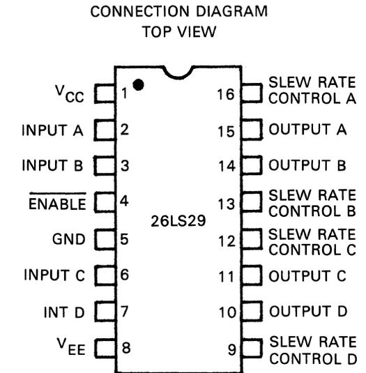
NOTE: PIN 1 IS MARKED FOR ORIENTATION.
