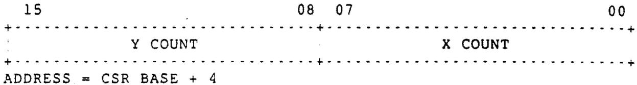
Figure 4-6: Mouse Position Register Format
