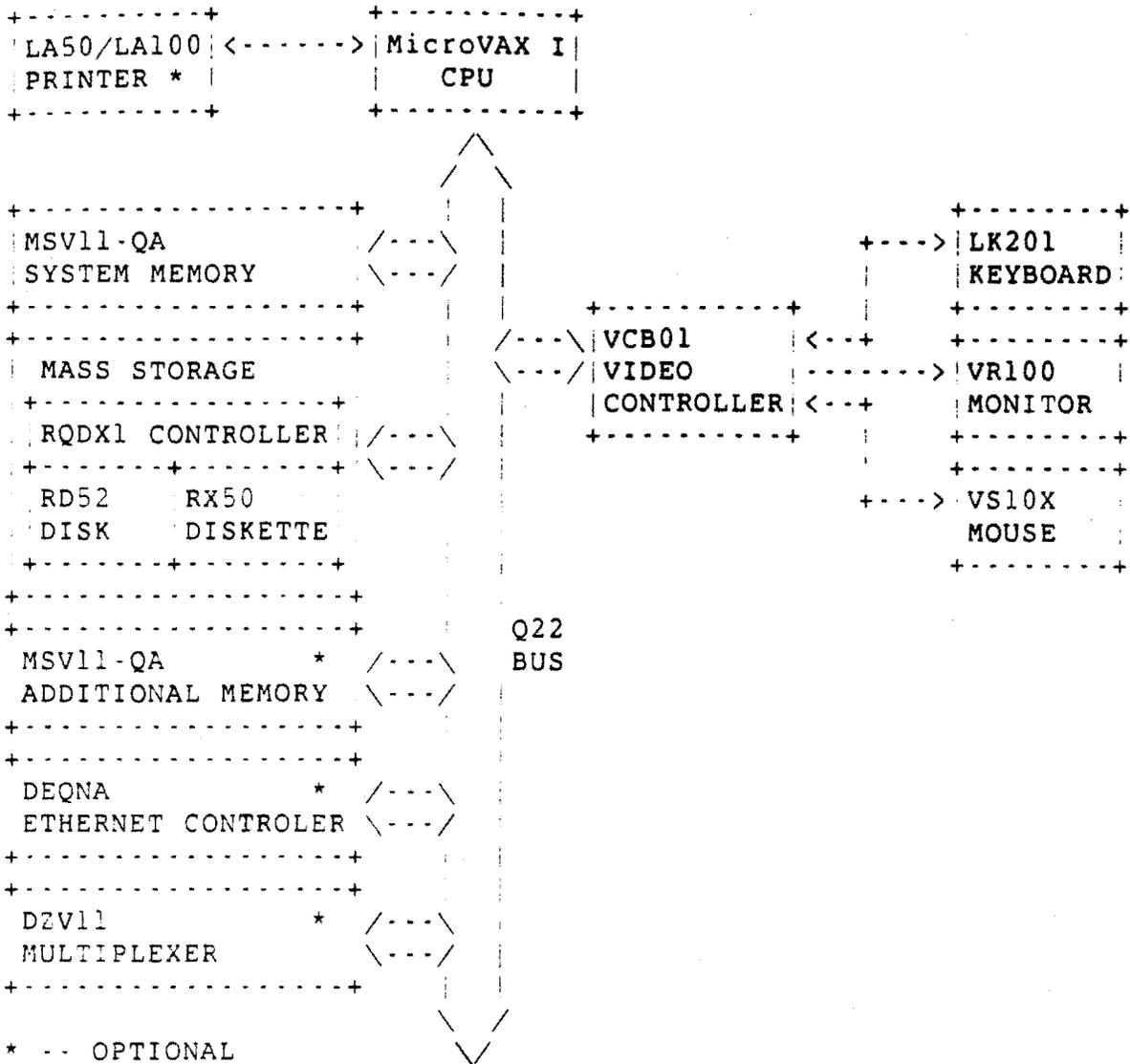
Figure 1-2: VAXstation I Block Diagram
