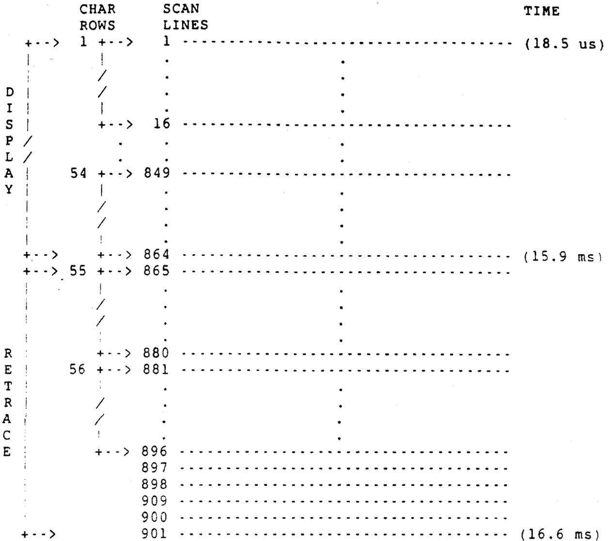
**Figure 3-8: CRTC Vertical Timing**
