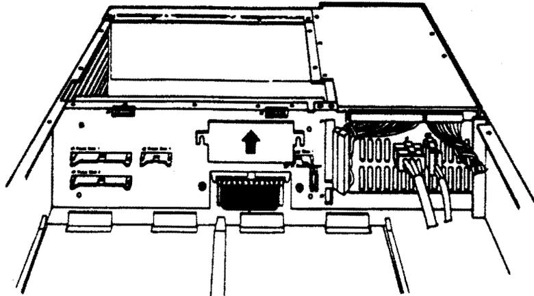
**Figure 6-26: Q22-bus Cable Backplane Connector**
