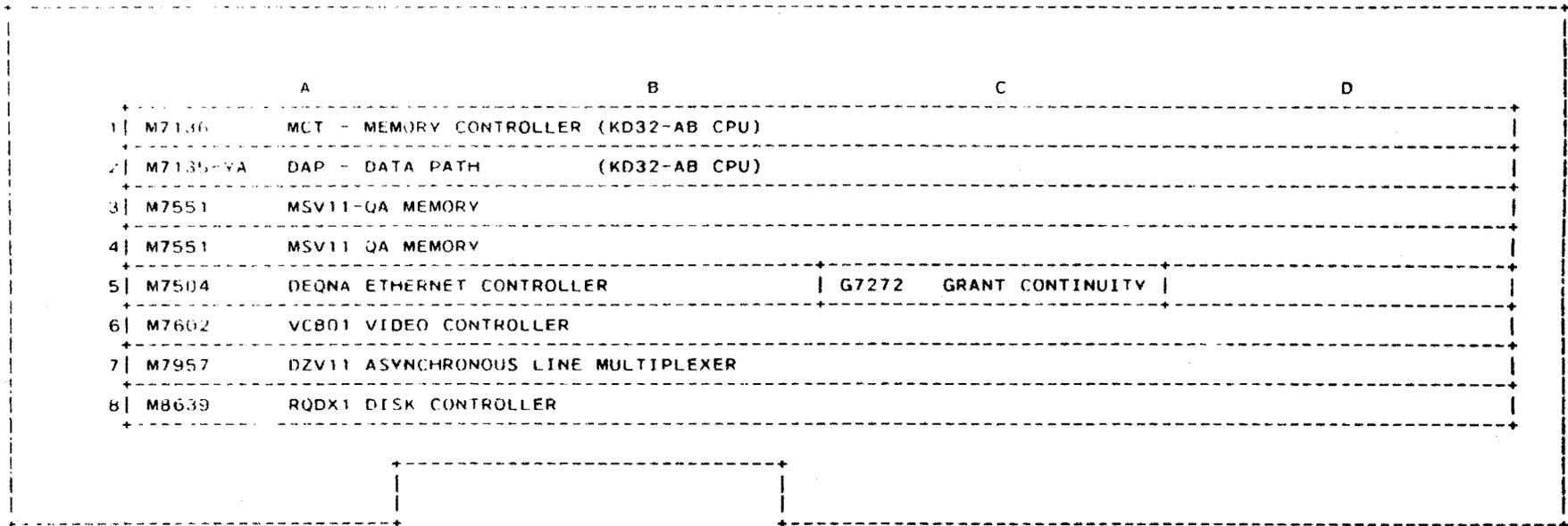
Figure 2-1: Backplane Configuration Example
