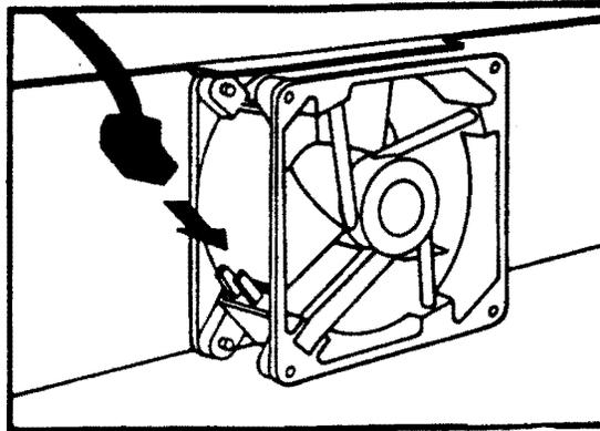
Figure 6-23: Fan Power Connector
