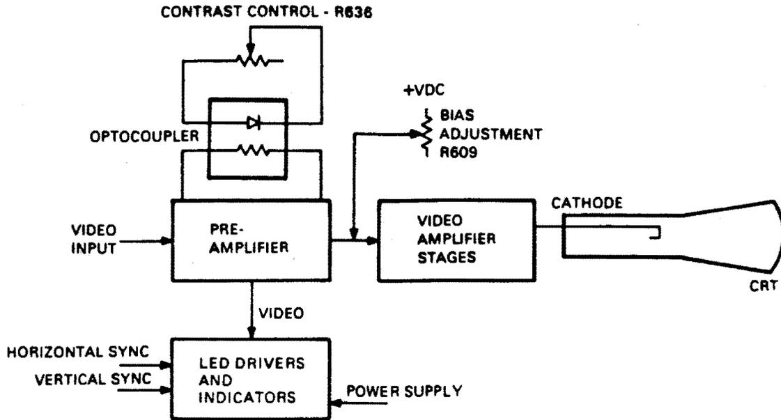
Figure 3-19: Video Module Block Diagram
