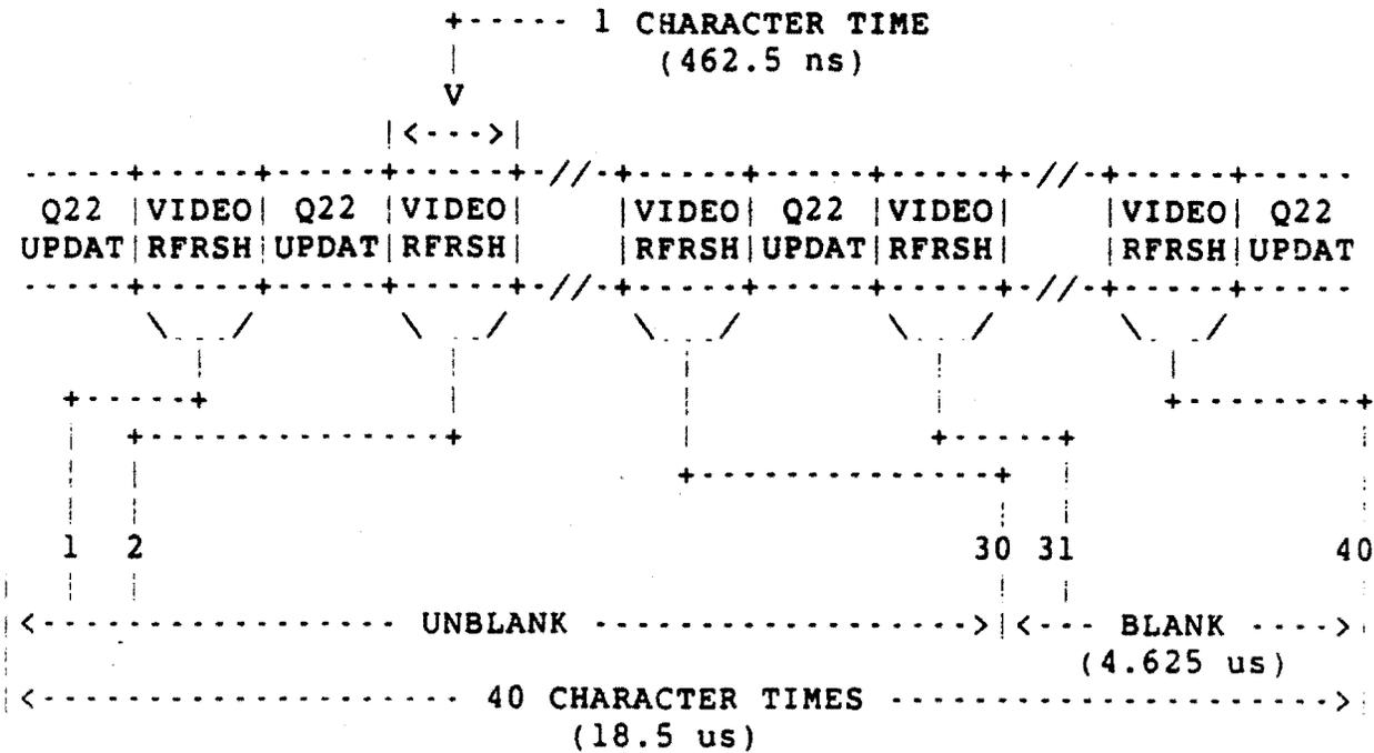
Figure 3-7: CRTC Horizontal Timing
