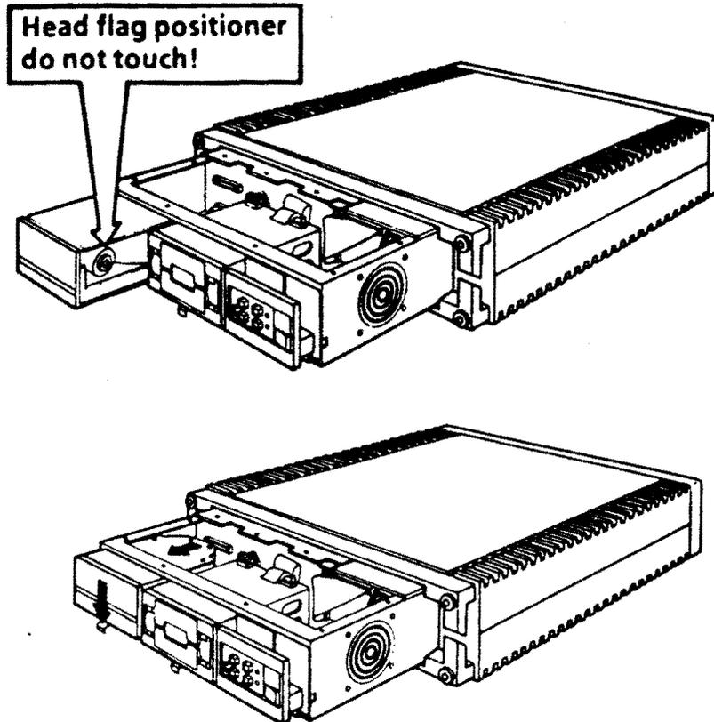
Figure 6-11: RD52 Cable Access
