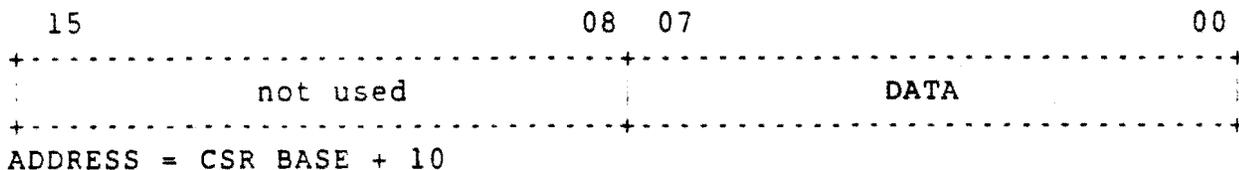
**Figure 4-8: CRTC Data Register Format**
