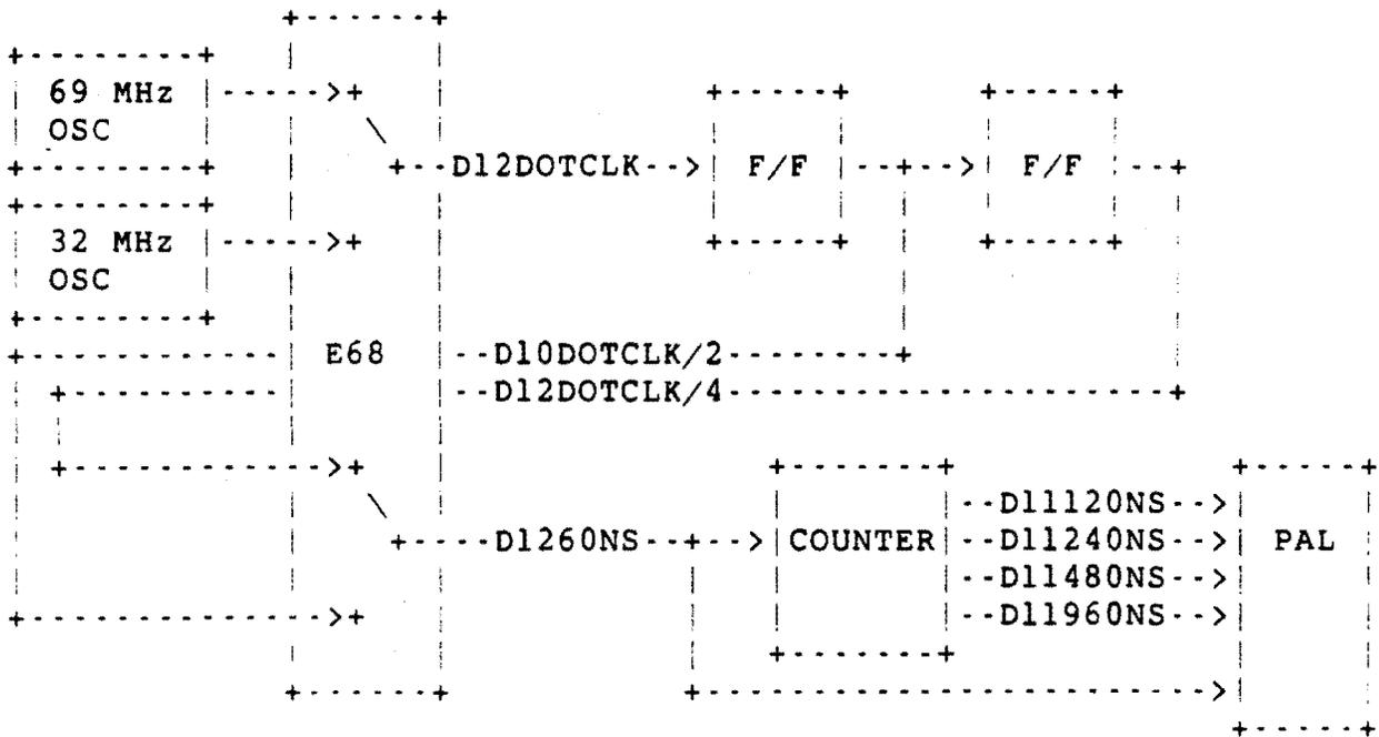
Figure 3-3: Simplified Timing Generator
