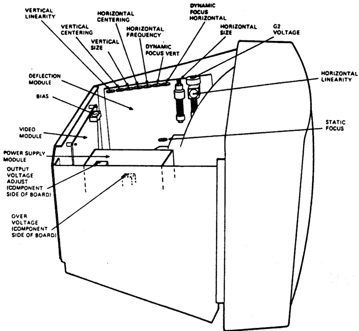
Figure 5-8: Monitor Internal Controls
