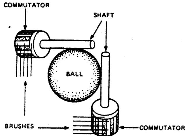
Figure 3-15: Mouse Construction
