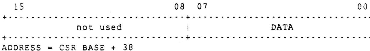
Figure 4-14: Transmit/Receive Buffer A Format
