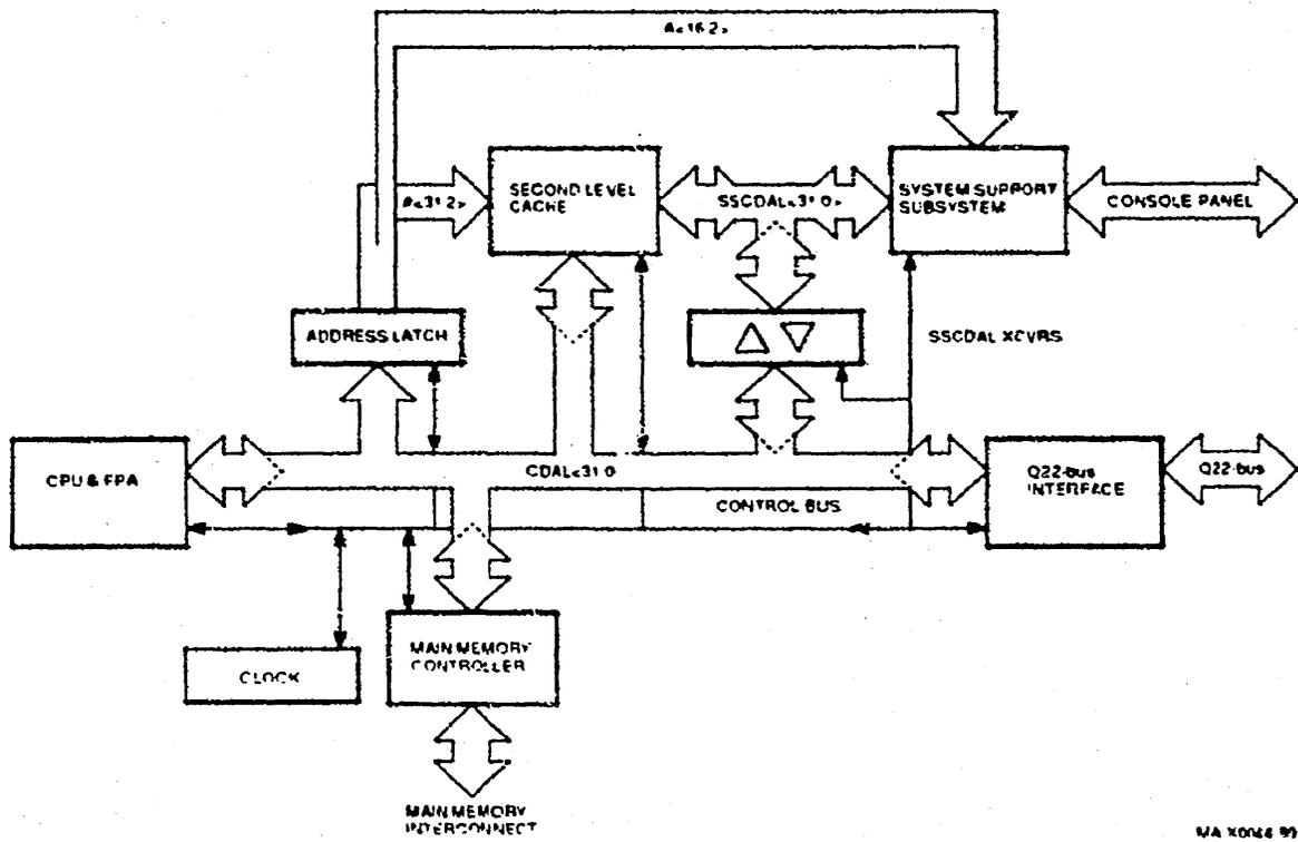
Figure 1-2 KA655 Block Diagram
