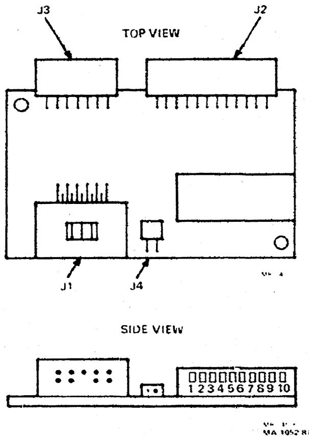
Figure 2-5 KA630CNF Configuration Board
