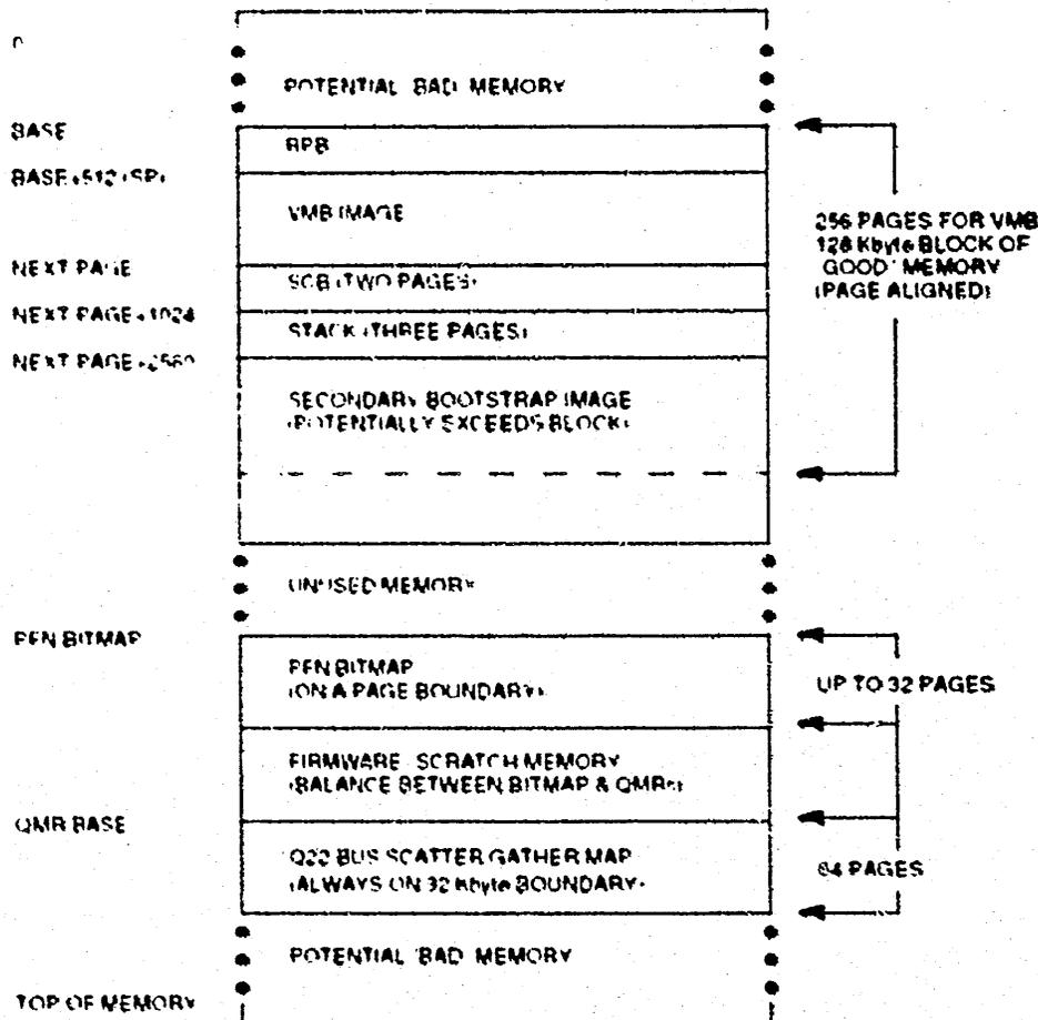
Figure 4-2 Memory Layout at VMB Exit
