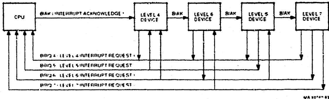
**Figure C-13 Position-Independent Configuration**
