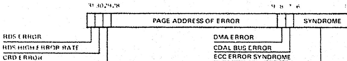
Figure 3-21 Format for MEMCSR16
