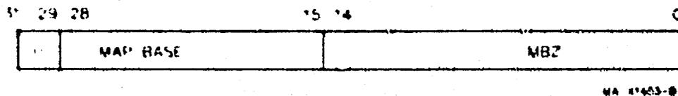
Figure 3-39 Q22-bus Map Base Address Register
