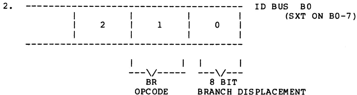
The branch displacement will be left shifted by one and sign extended on bit 7. For VAX Mode The IDMX Will Be As Follows:
