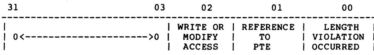
The protection violation is detected by the utrap function for data path cycles and the ubranch function for IBUF cycles. The length violation is detected by the ubranch function and the virtual address is always located in VA.
