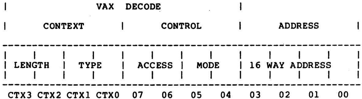
ADDRESS: THE ADDRESS FIELD IS USED TO PROVIDE A 16 WAY LITERAL DISPLACEMENT WHEN GENERATING AN EXECUTION ADDRESS. THE ADDRESS IS ONES COMPLEMENTED BEFORE GOING TO THE MICRO SEQUENCER.
