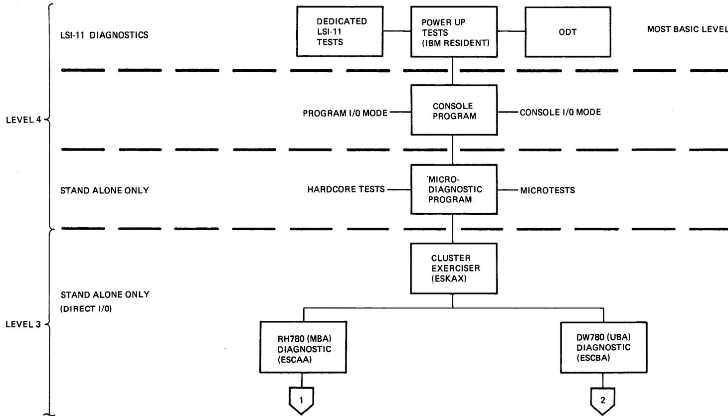
Figure 1-1 VAX-11/780 Diagnostic System Program Hierarchy (Sheet 1 of 2)
