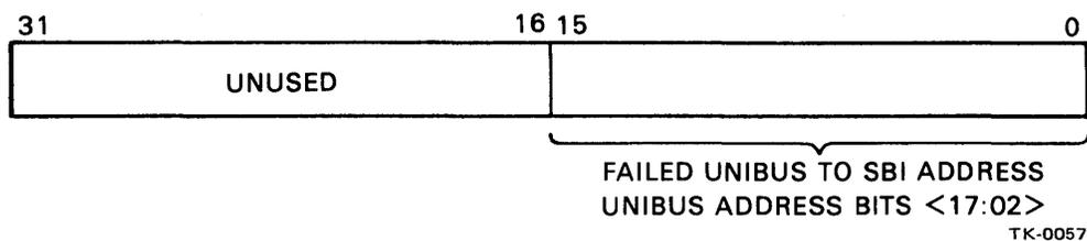
Figure 2-51 Failed Unibus Address Register, Bit Configuration
