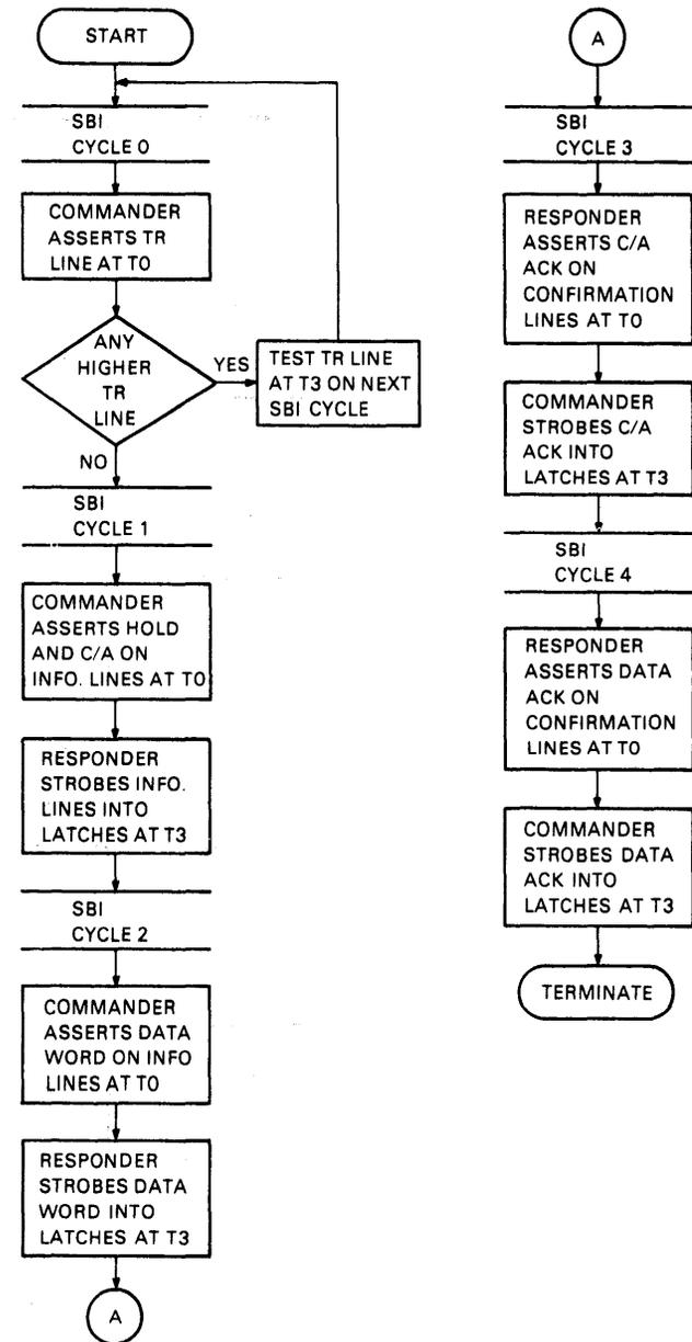
Figure 2-24 Write Masked Timing Chart and Flow
