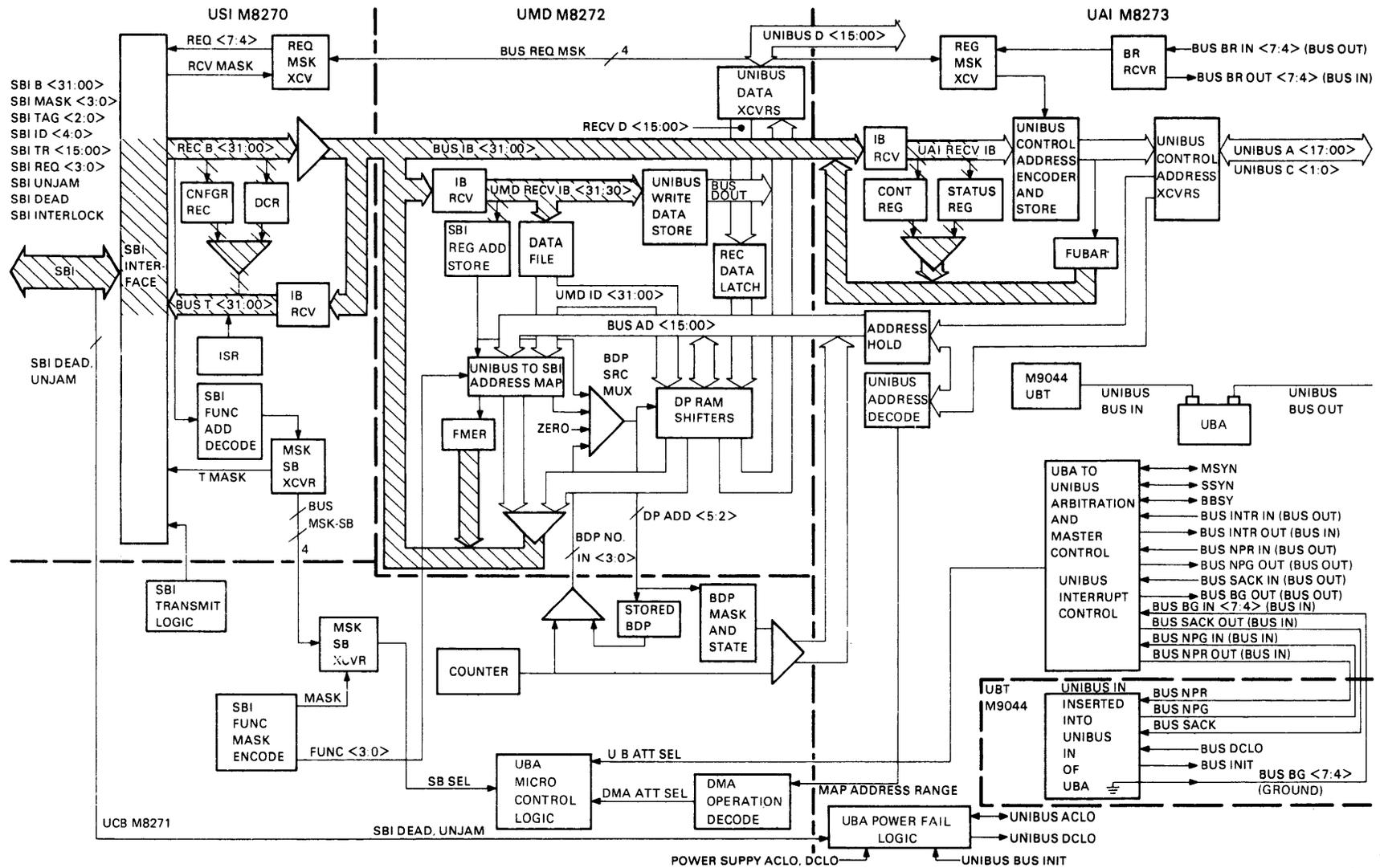
Figure 3-28 B Field Logic/UBA, Block Diagram
