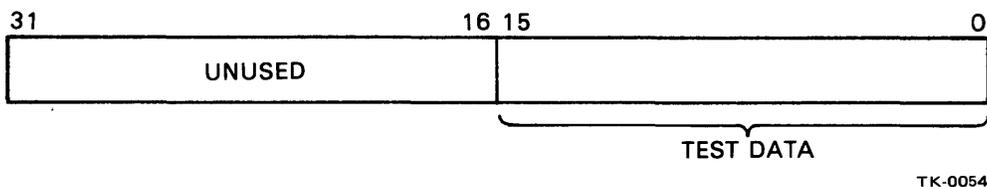
Figure 2-52 Buffer Selection Verification Register Bit Configuration
