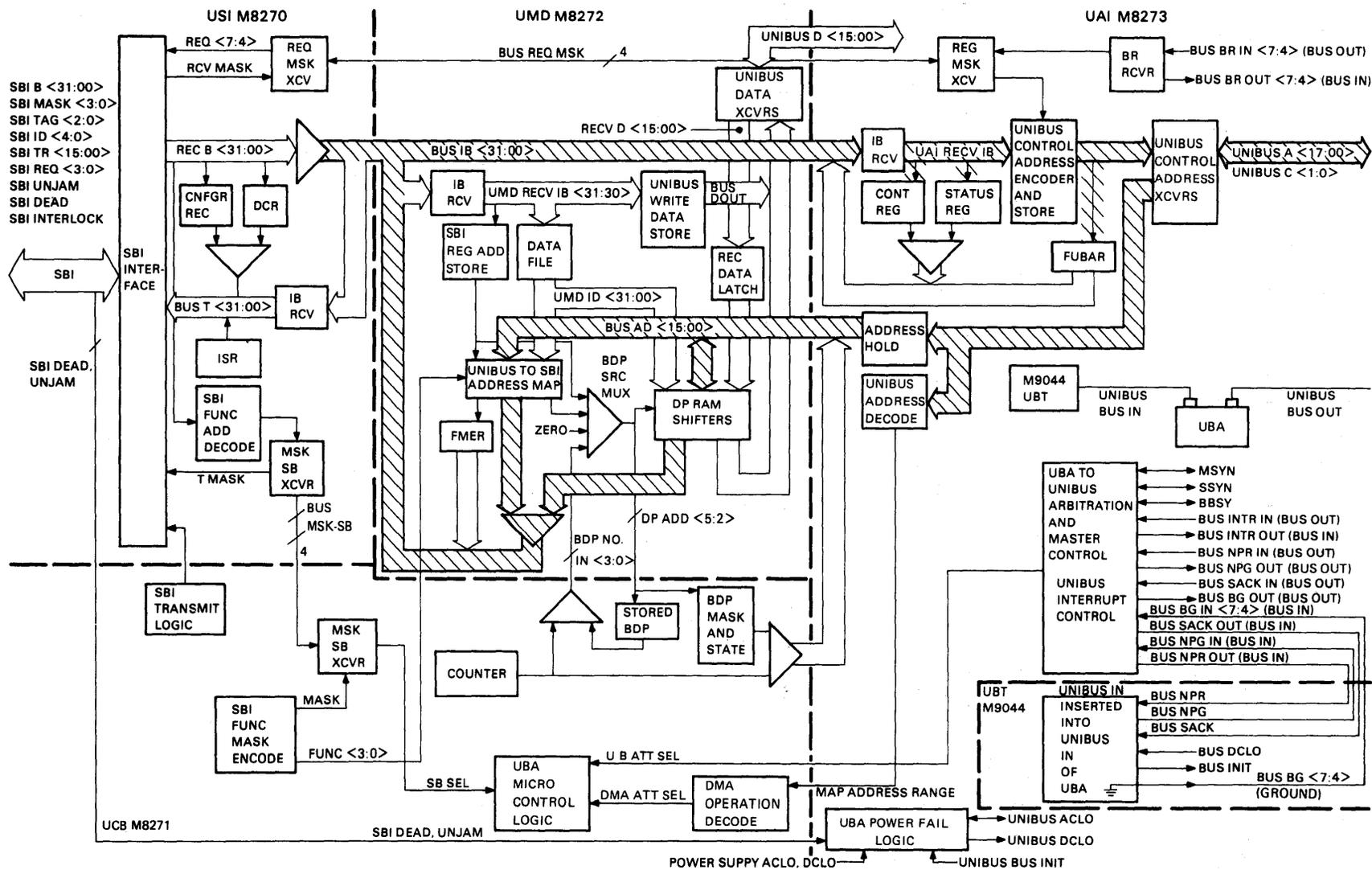
Figure 3-44 Unibus Address and Control Logic/
