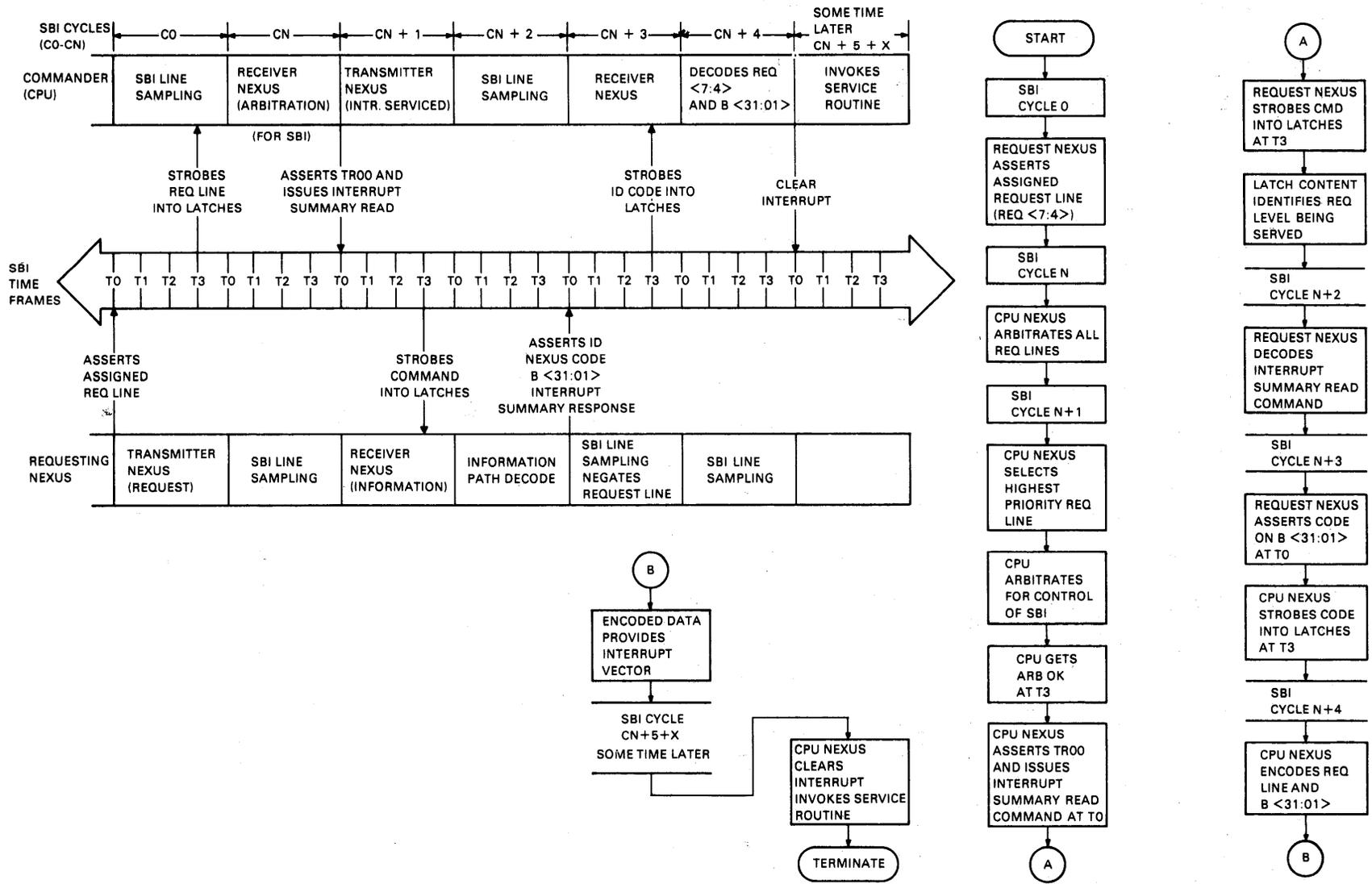
Figure 2-16 Interrupt Operation Timing and Flow
