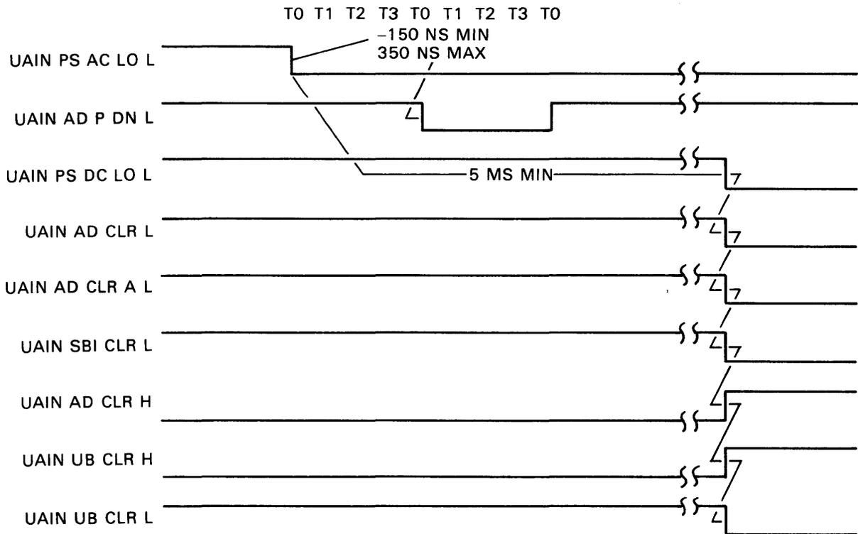
Figure 3-62 System Power Down Sequence, Timing Diagram
