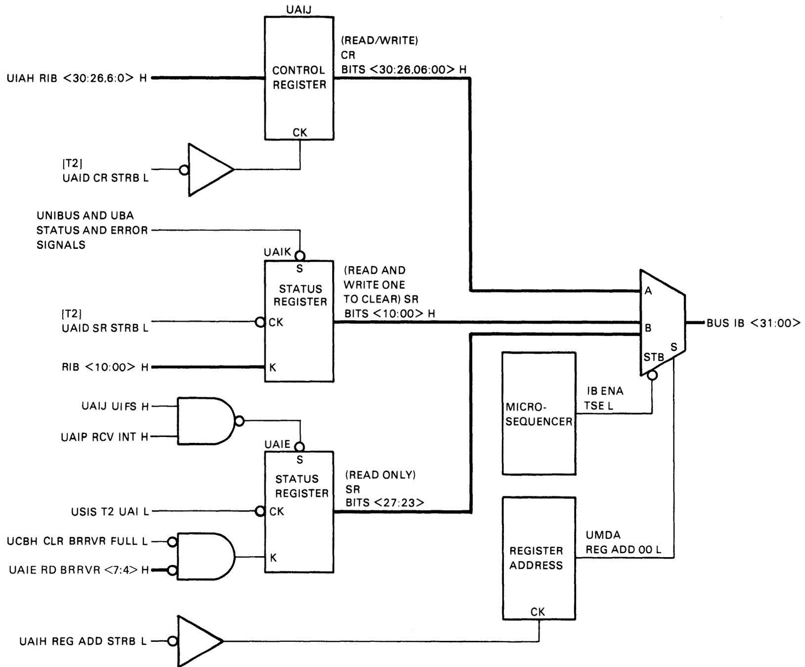
Figure 3-68 Control and Status Registers, Block Diagram
