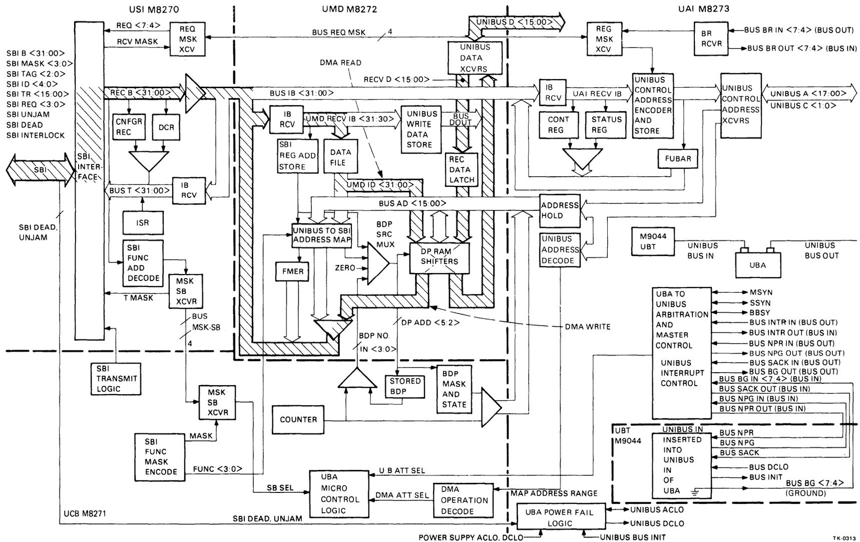
Figure 2-40 Data Paths for Unibus DMA Access to the SBI/UBA Block Diagram
