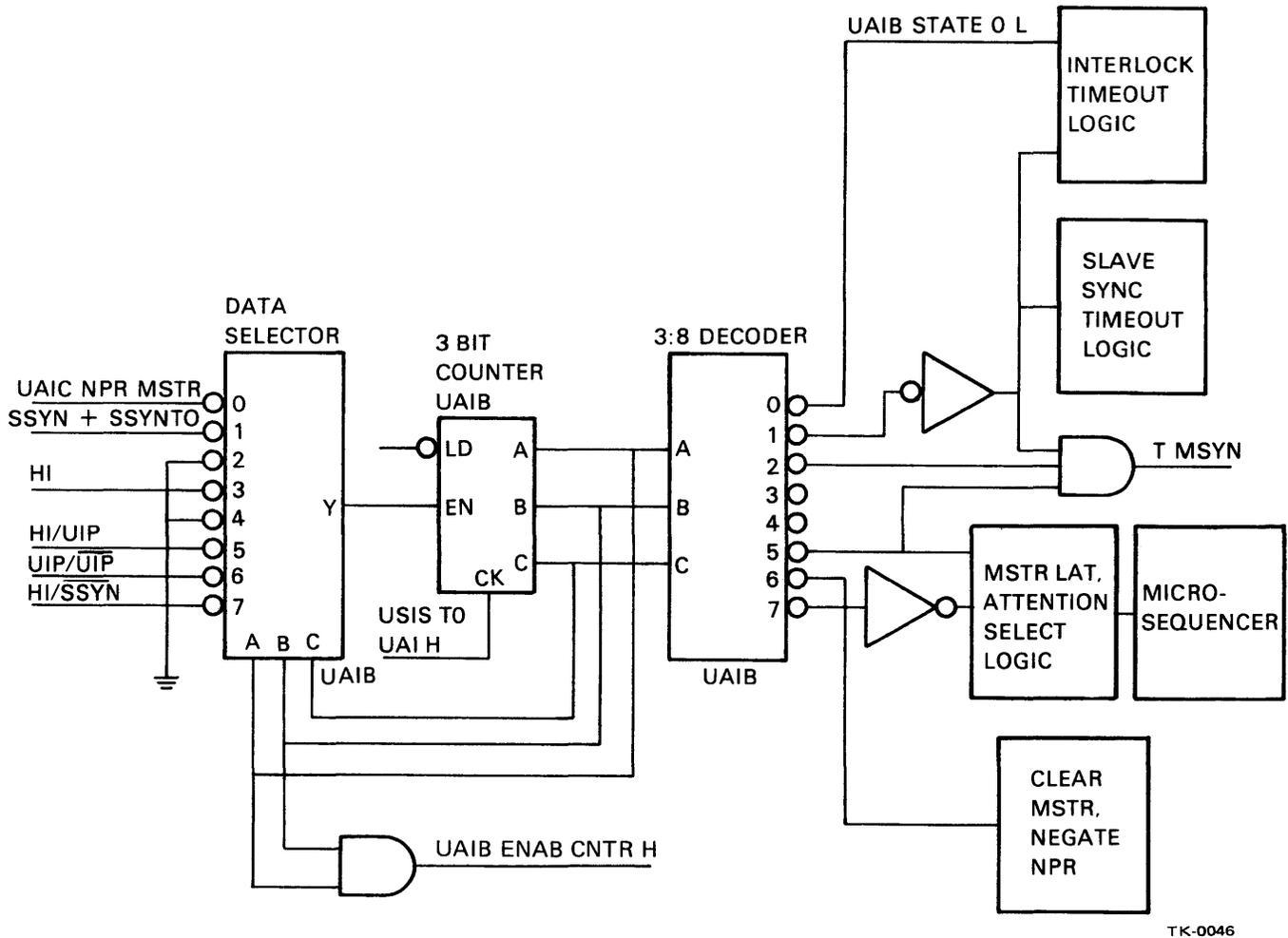
Figure 3-54 Unibus Control State Counter, Block Diagram
