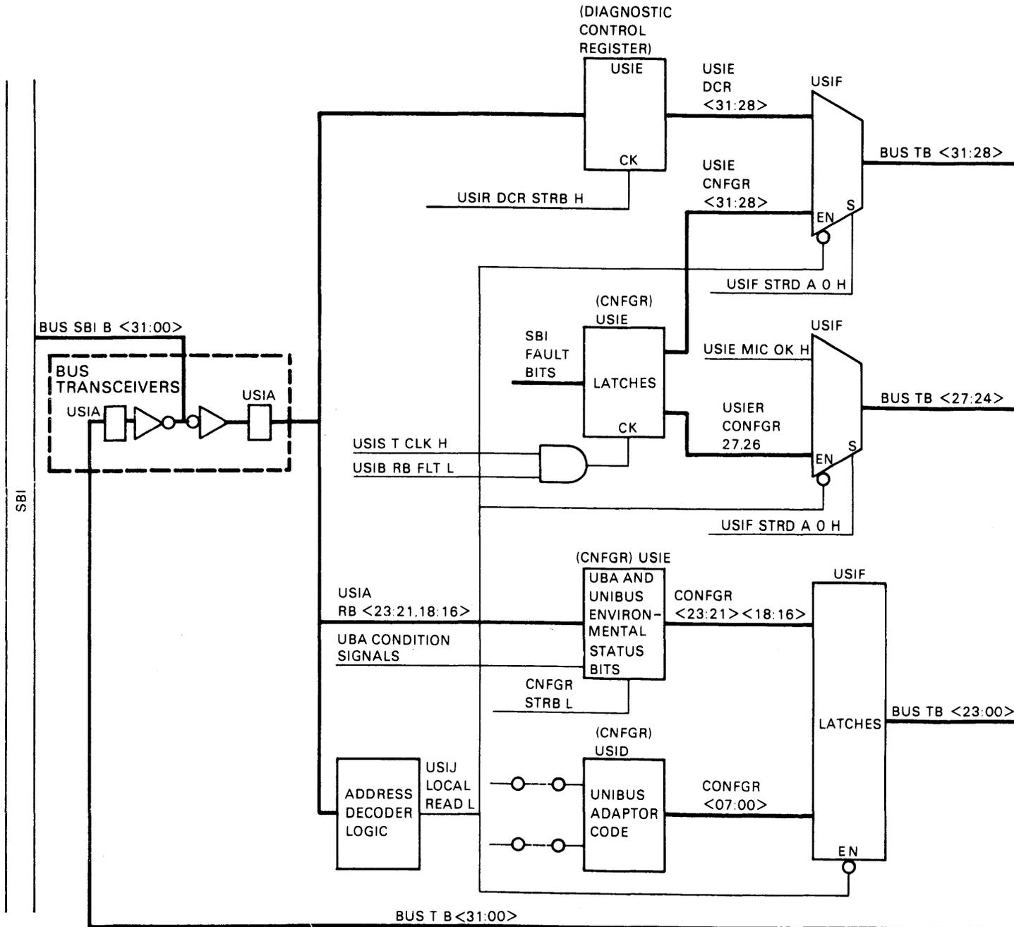
Figure 3-66 Configuration and Diagnostic Control Registers Block Diagram
