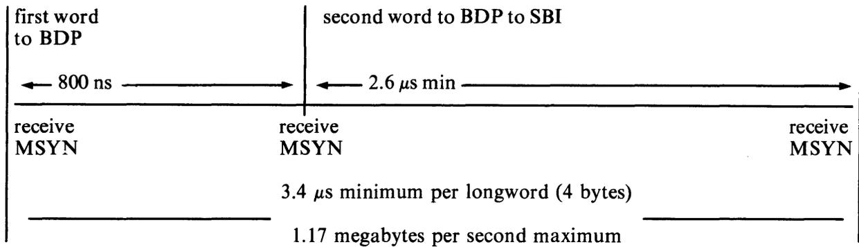
The operation of the UBA for the longword aligned 32-bit random access mode is determined by the function (DATI, DATO, and DATOB) and address (A1, A0) received from the Unibus and by the state of the buffer not empty (BNE) bit of the data path register corresponding to the BDP being used for this operation.
