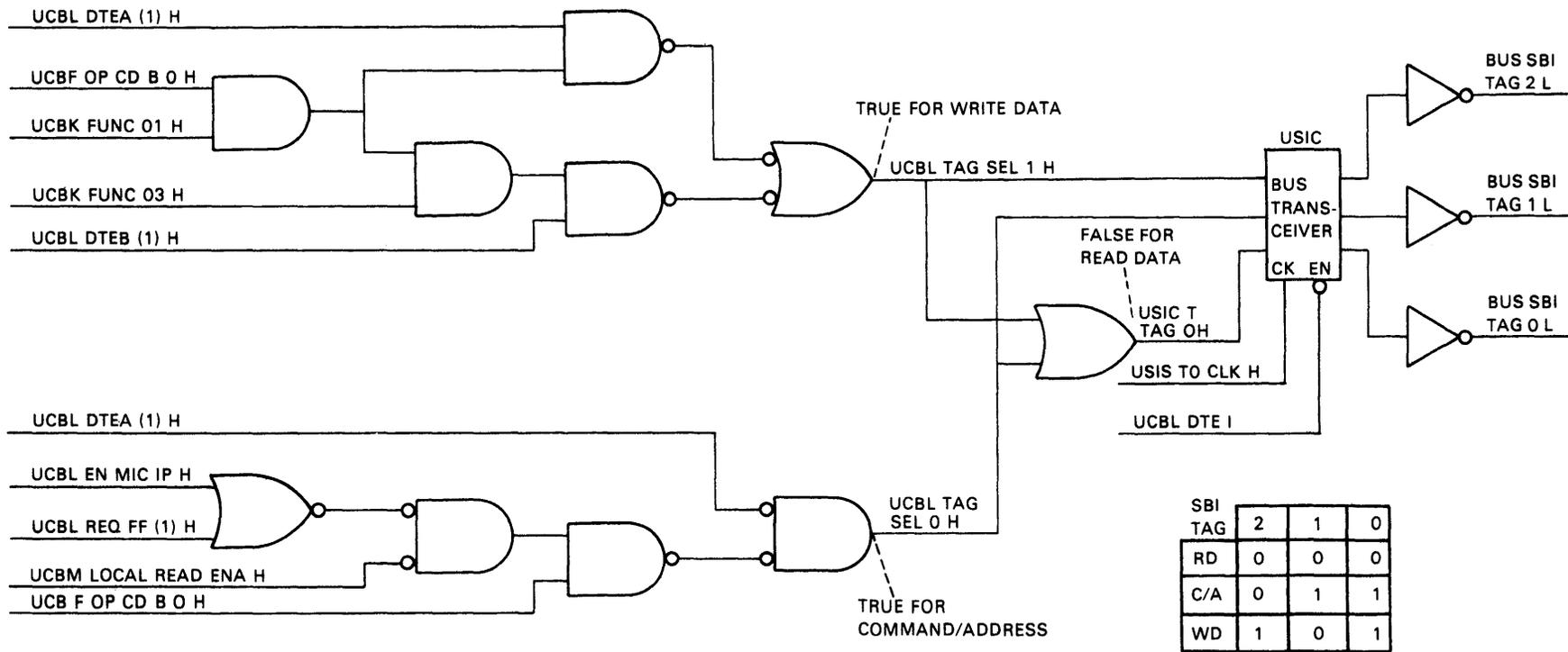
Figure 3-38 Tag Encoder Logic
