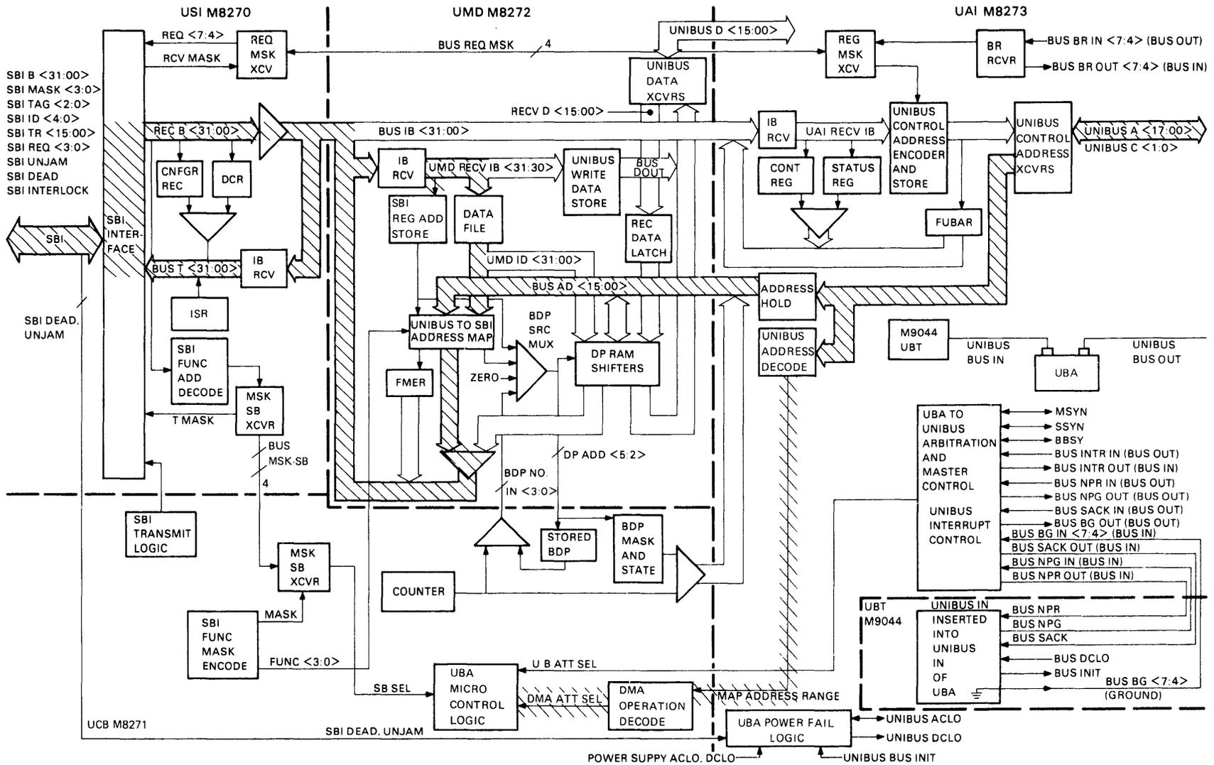
Figure 3-65 Map Register Logic/UBA Block Diagram
