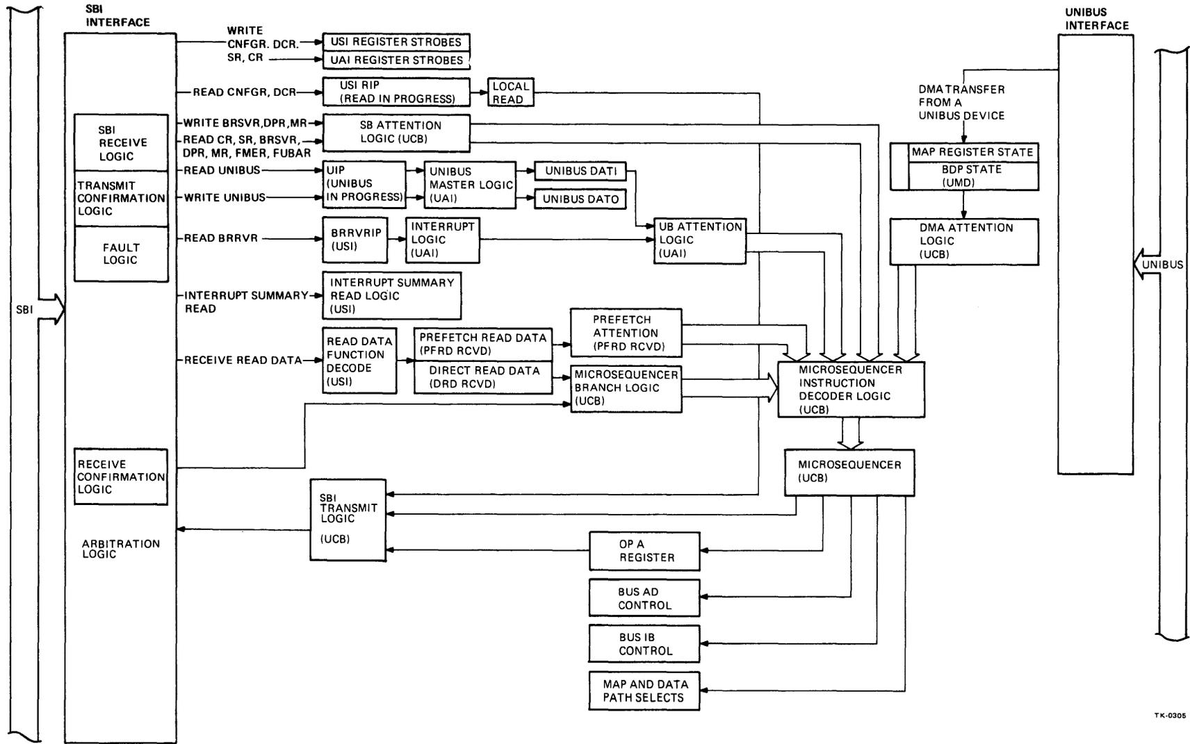
Figure 2-65 Simplified Flow of Major Control Functions within the UBA
