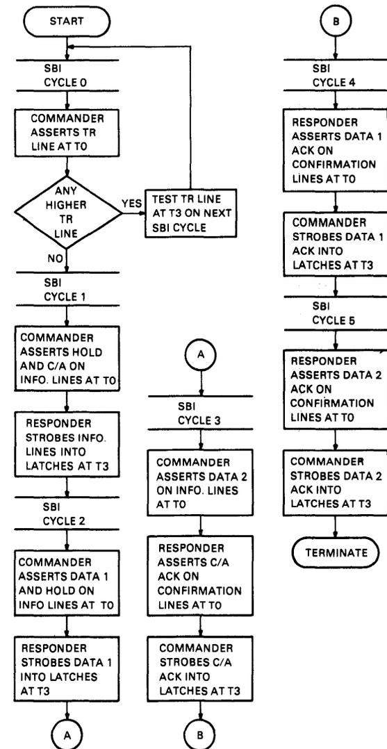
Figure 2-26 Extended Write Masked Timing Chart and Flow
