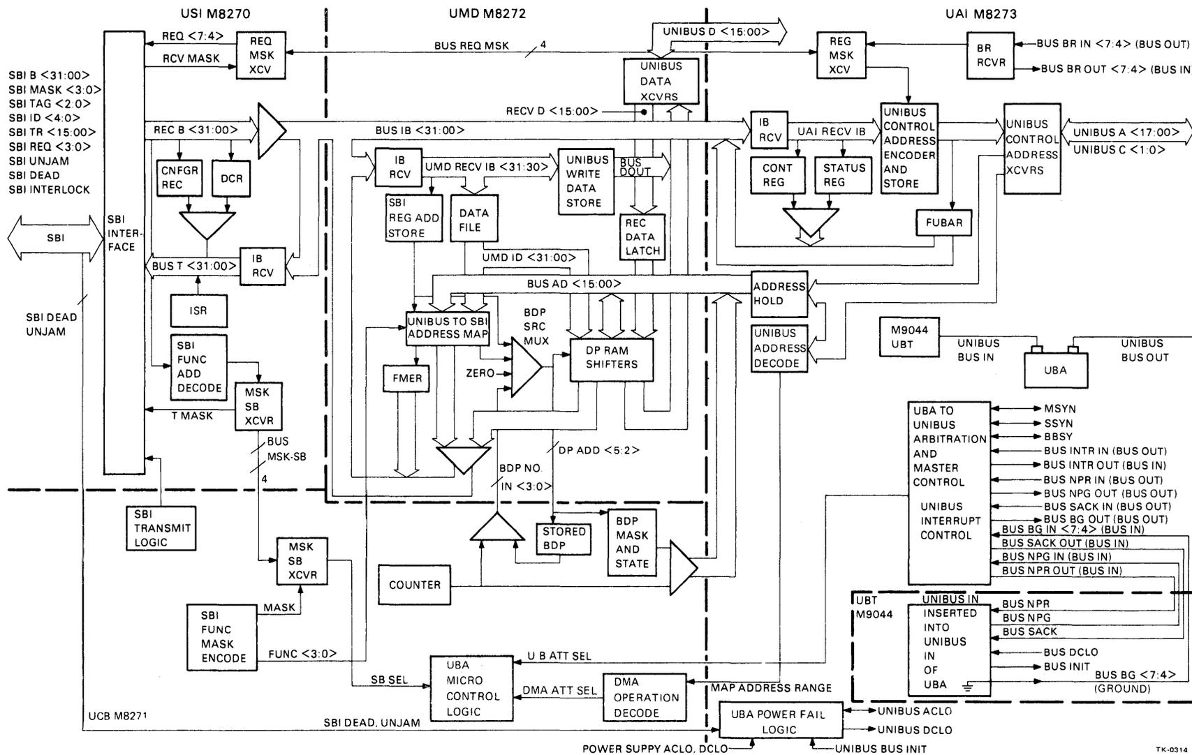
Figure 2-32 UBA Block Diagram
