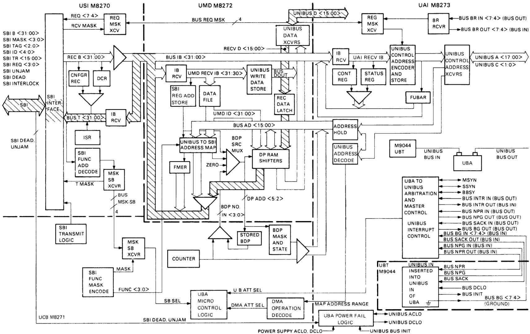
Figure 2-37 Data Route for Read Transfer to the Unibus/UBA Block Diagram
