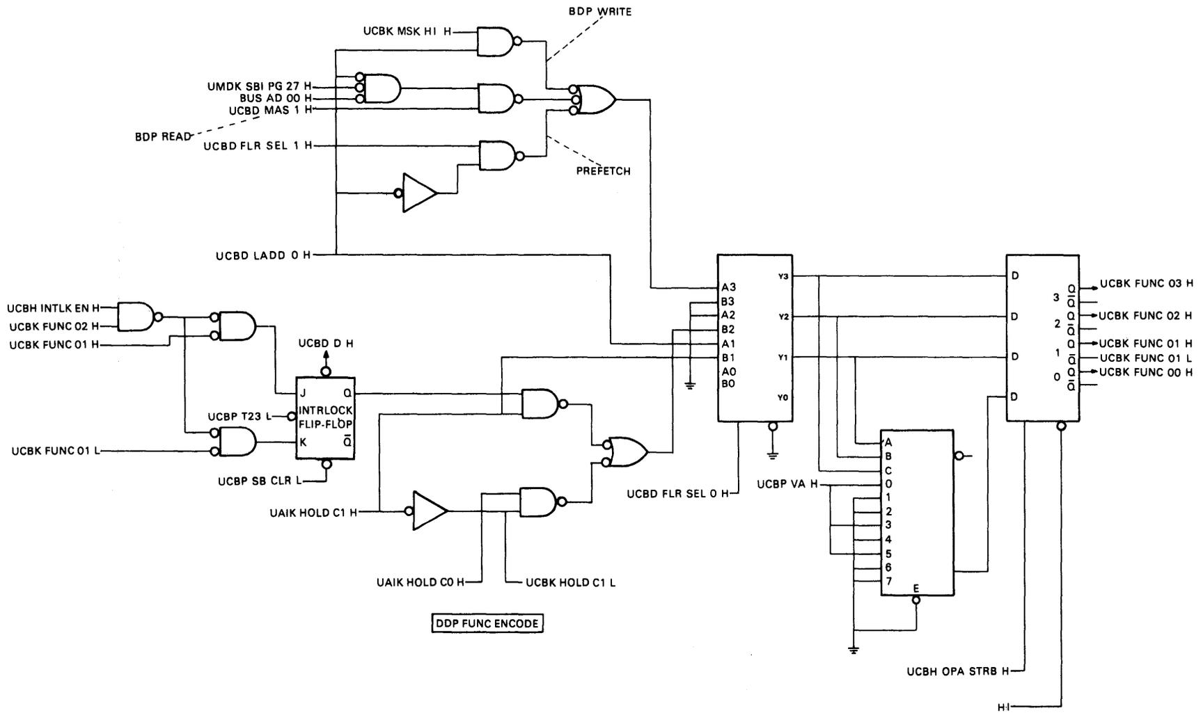
Figure 3-33 Function Encoder Logic
