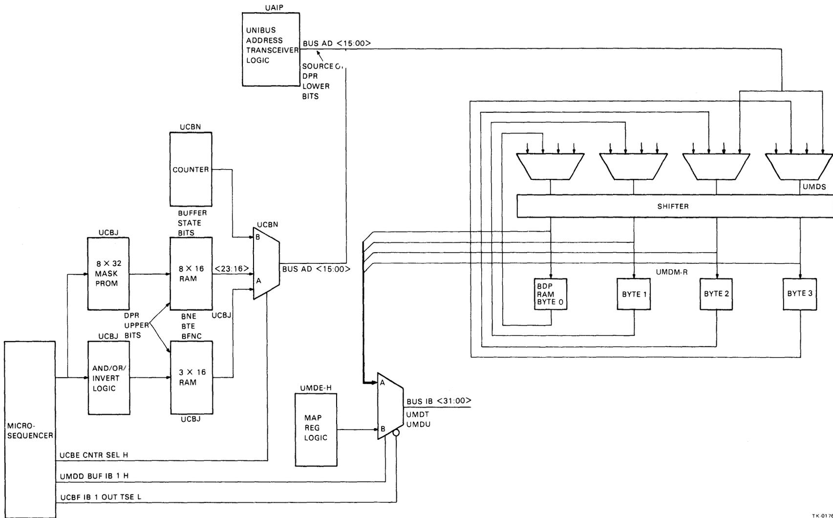
Figure 3-74 Data Path Registers, Block Diagram
