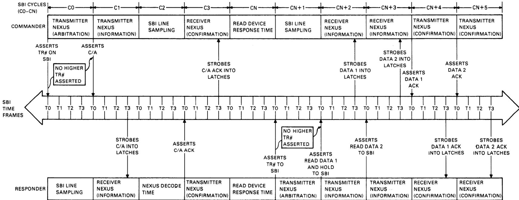
Figure 2-22 Extended Read Timing Chart and Flow (Sheet 1 of 2)
