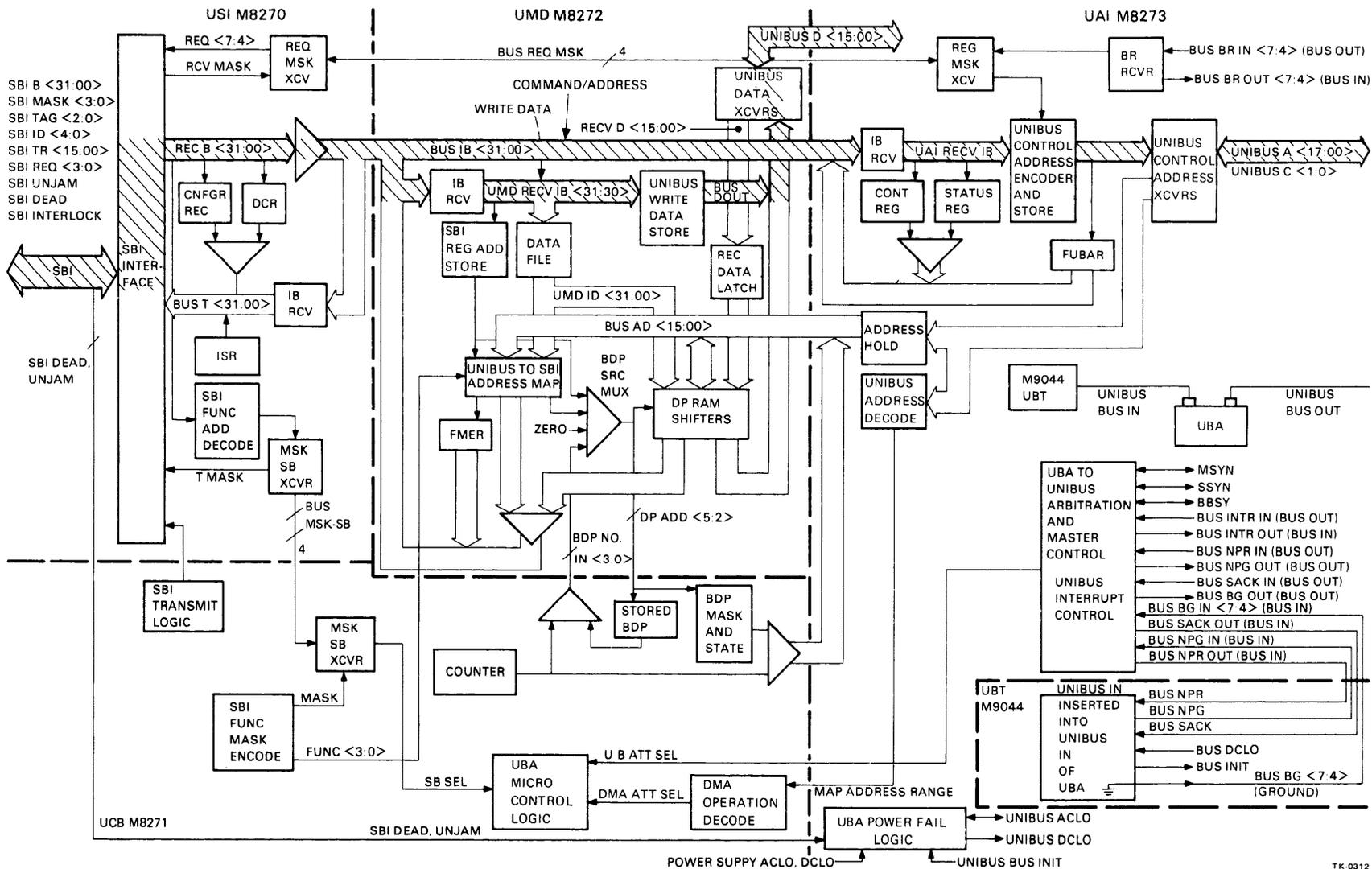
Figure 2-35 Data Route for Write Transfer to a Unibus Device/UBA, Block Diagram
