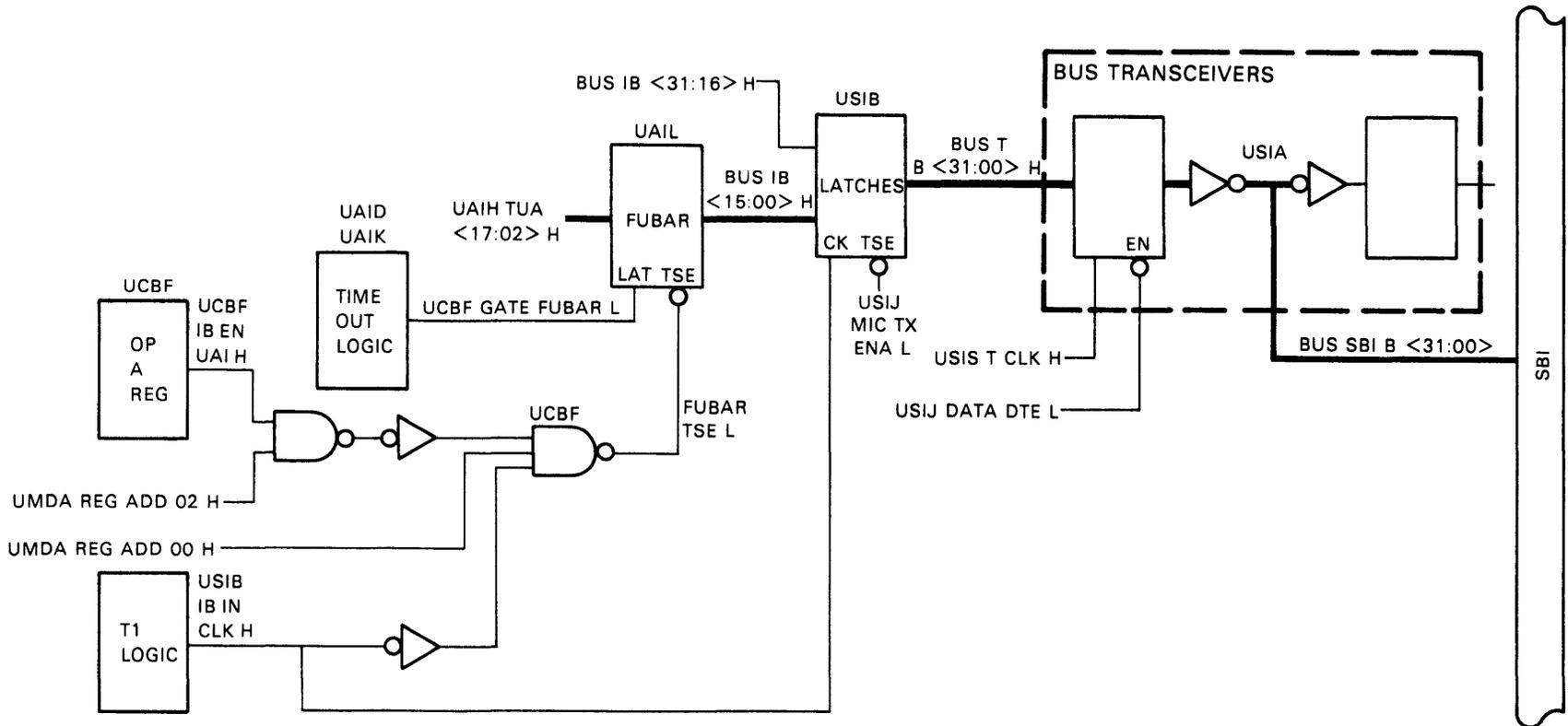
Figure 3-72 Failed Unibus Address Register and Associated Logic, Block Diagram
