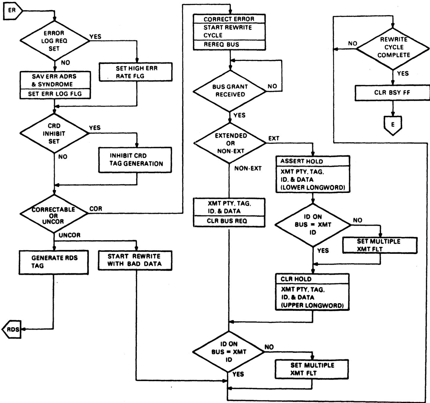
Figure 2-16 Array Read Cycle Sequence (Sheet 2 of 2)
