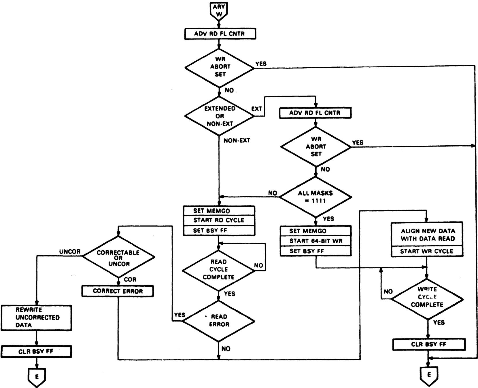
Figure 2-15 Array Write Cycle Sequence
