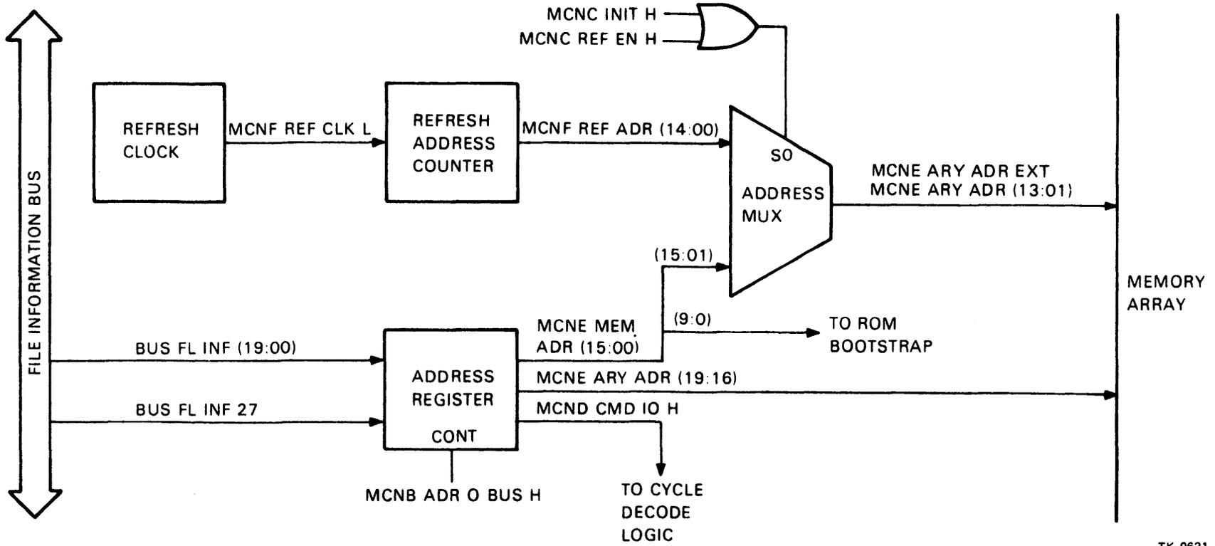
Figure 3-2 Address Logic
