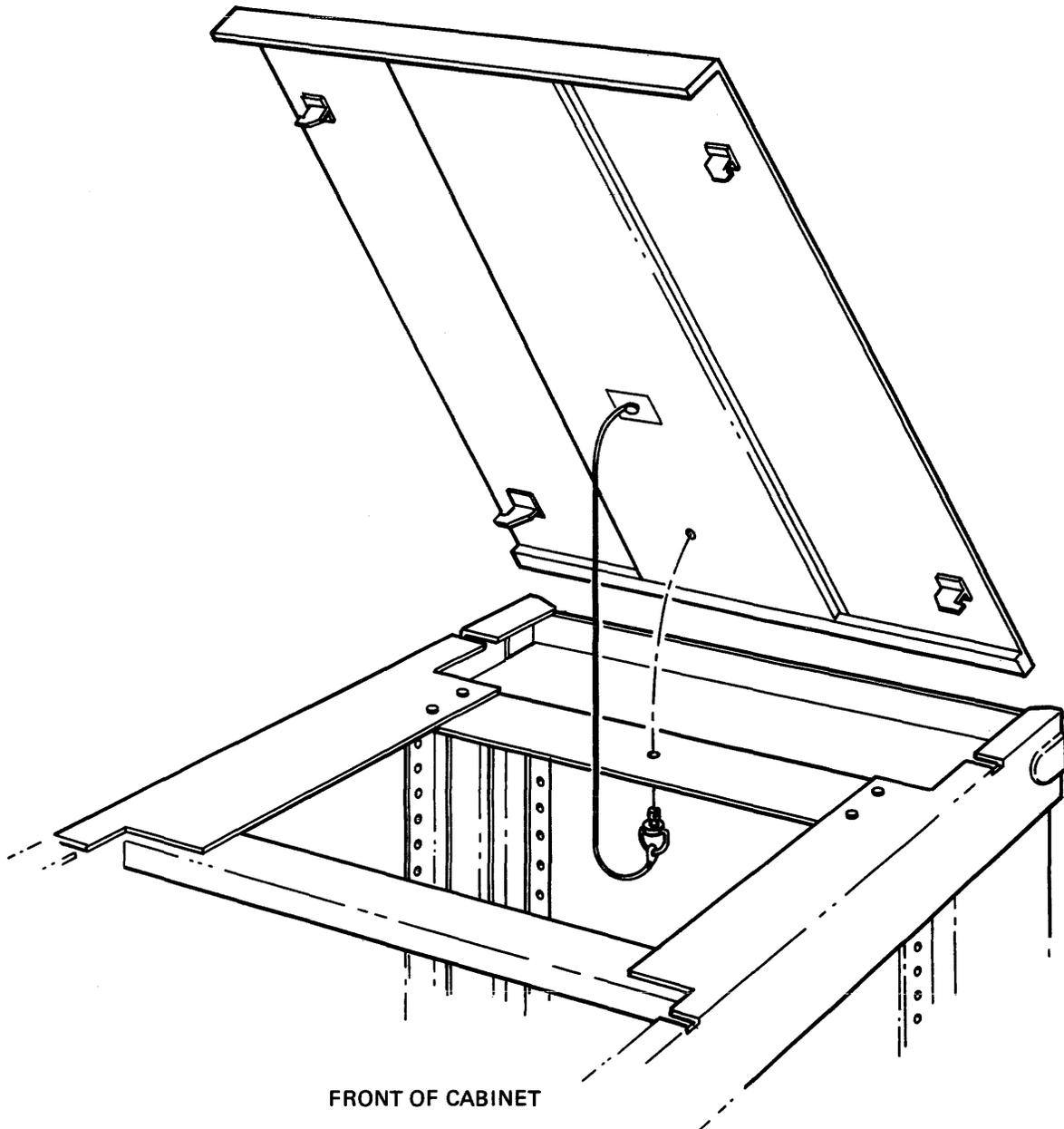
Figure 3-4 Top Cover Fastener
