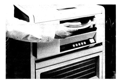
Figure 3-8 • TSV05 Streaming-tape Drive
