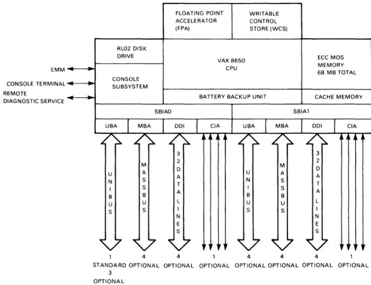
Figure 3-7 ■ VAX 8650 System Hardware Configuration
