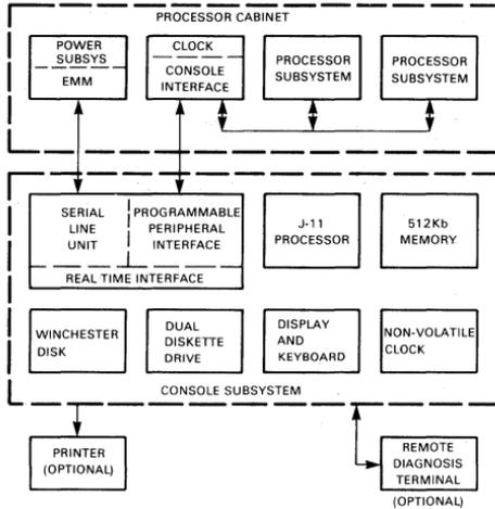
Figure 2-6 ■ Console Subsystem Block Diagram
