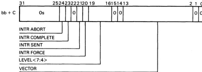
Figure 6-6 ■ Error Interrupt Control Register
