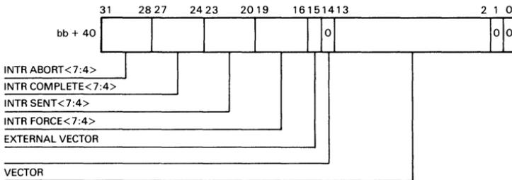
Figure 6-16 ■ User Interface Interrupt Control Register
