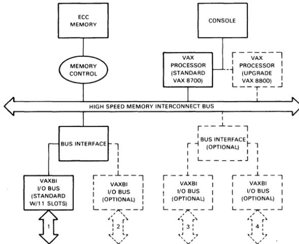
Figure 2-4 ■ VAX 8700 System Configuration
