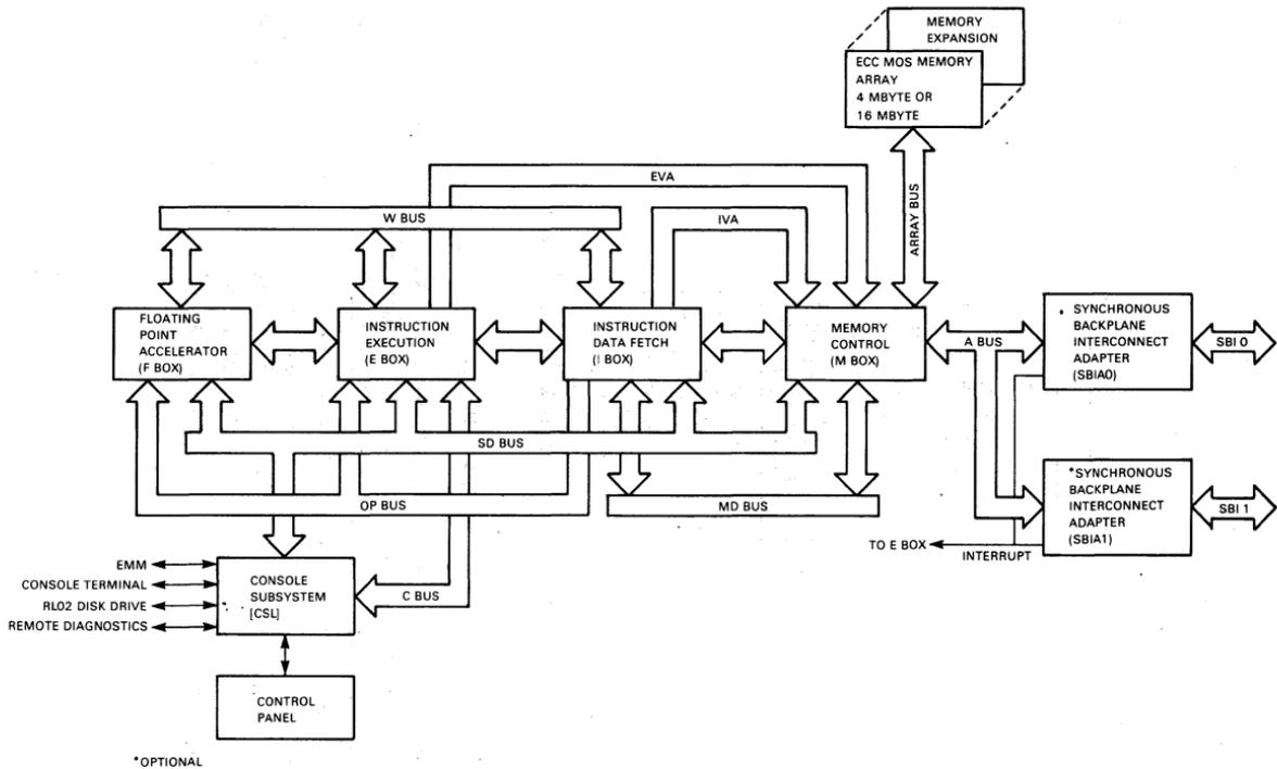
Figure 3-5 ■ VAX 8650 Processor Components
