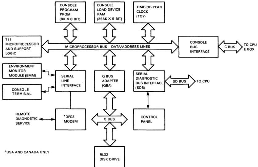
Figure 3-6 ■ VAX 8650 Console Subsystem Components
