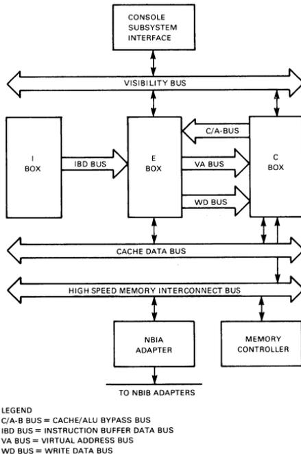
Figure 2-7 ▪ VAX 8800 and VAX 8700 Processor Block Diagram
