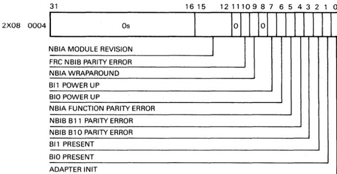
*Figure 6-29 ■ CSR1 NBIA Adapter Register*
