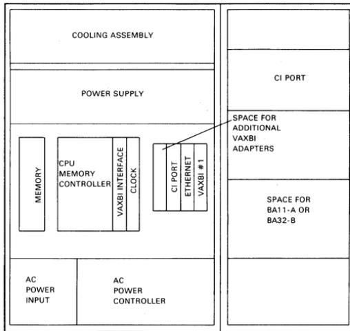
Figure 4-4 ■ VAX 8550 and VAX 8500 Processor VAXcluster Configuration
