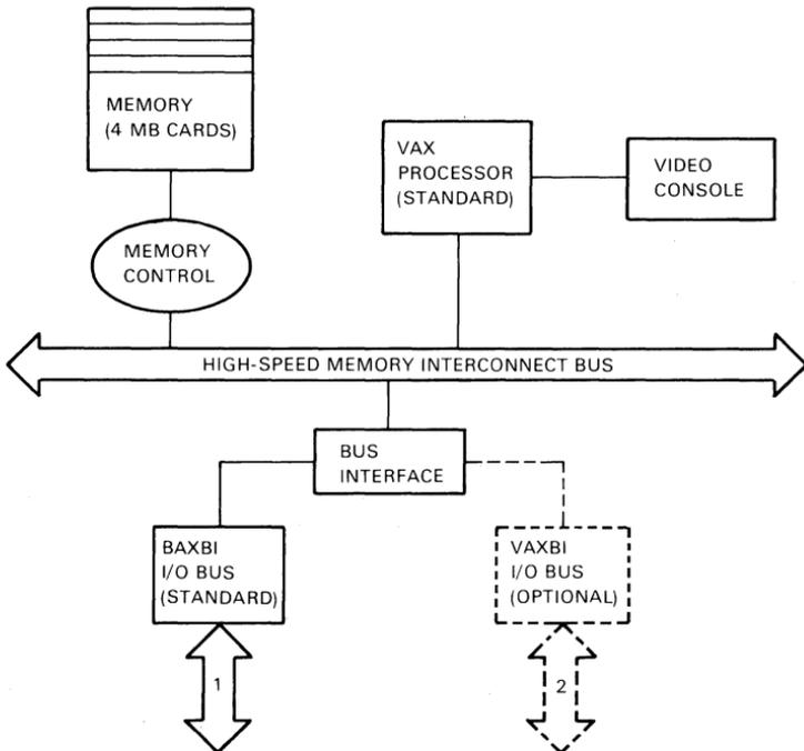
Figure 4-5 ■ VAX 8550 Processor Configuration
