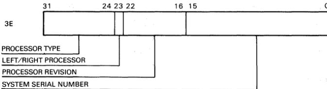
*Figure 6-1 ■ VAX 8800/8700 and VAX 8550/8500 SID Register Format*
