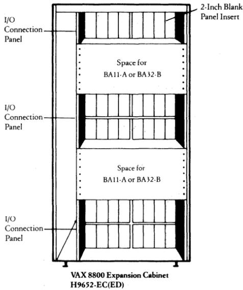
Figure 2-3 ■ H9652-EC/ED VAXBI and UNIBUS Expansion Cabinet
