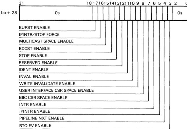
Figure 6-13 ■ BCI Control and Status Register
