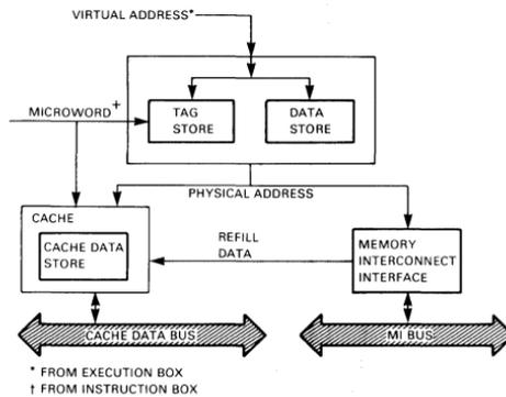
Figure 2-9 ■ Cache Box Block Diagram
