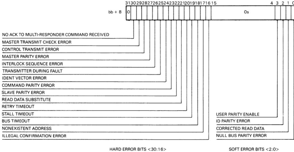
Figure 6-5 ■ Bus Error Register
