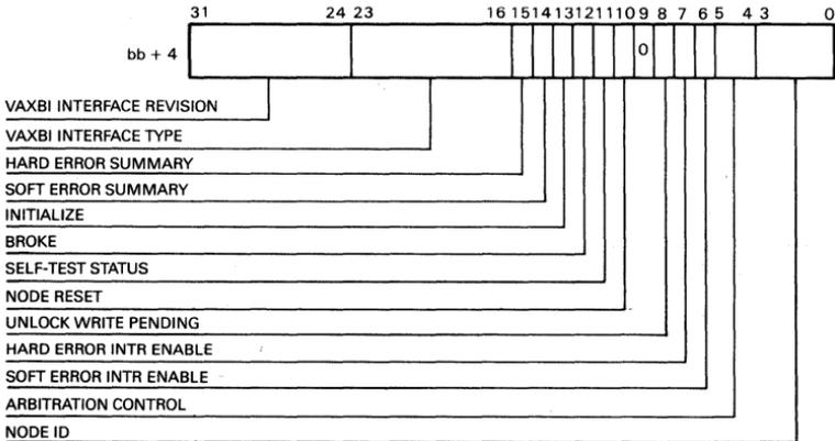
Figure 6-4 ■ VAXBI Control and Status Register
