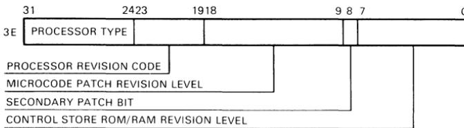
Figure 6-2 ■ VAX 8300/8200 SID Register Format
