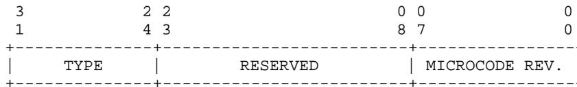
**SID<31:24> (TYPE) Processor type.** This field always reads as 12 (hex) indicating the processor is implemented using the DC595 CPU chip.
