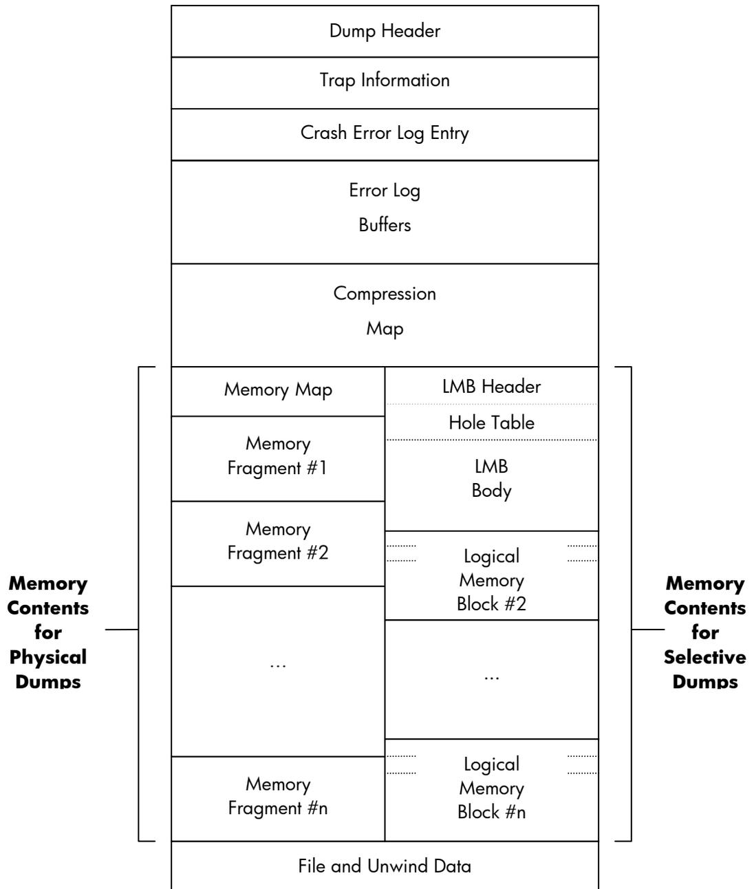
**Figure 2 Layout of Physical and Selective Dumps**
