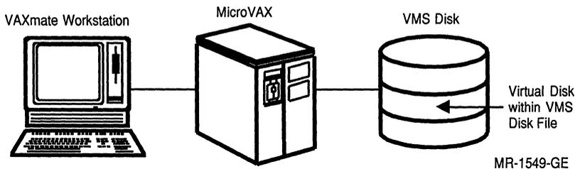
**Figure 2-1 Virtual Disk on a VMS Disk**
