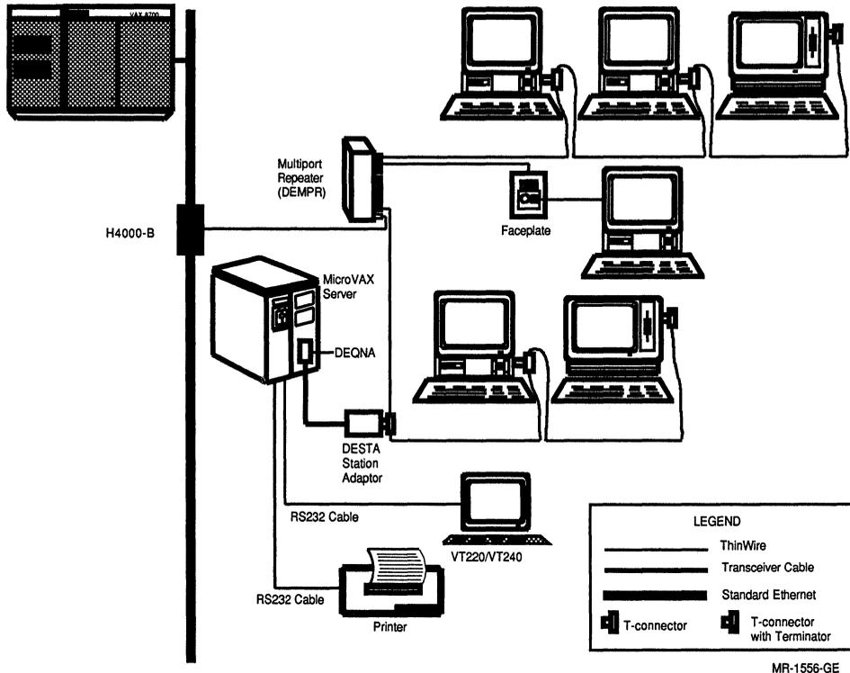
Figure 4-5 Daisy-Chain Connected to Corporate Ethernet Backbone
