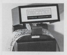
For accurate reading of standard 5, 6, 7 or 8-level paper, paper-polyester or metallized polyester tapes, DECITEK Readers provide uniform light to all channels by 9 discrete fiber optic elements, illuminated by a single, easily replaced bulb. Crosstalk and partial or bit failure are eliminated . . . photo-transistors deliver high signal-to-noise ratio outputs. Tapes of different levels can be read interchangeably without adjustment.
