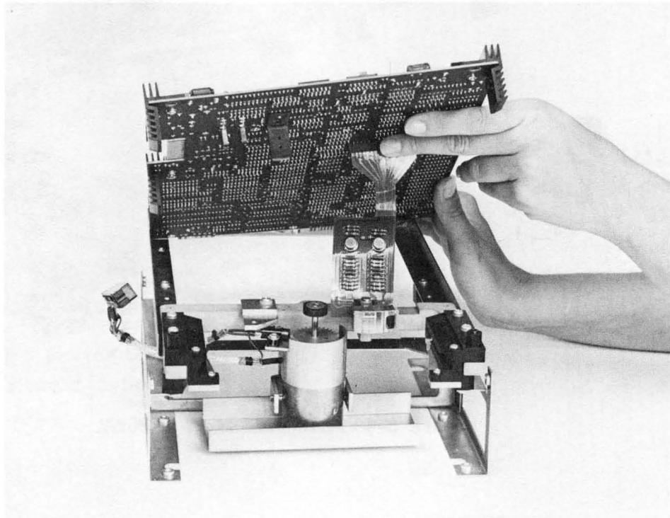
Figure 5-2 P.C. BOARD REMOVAL
