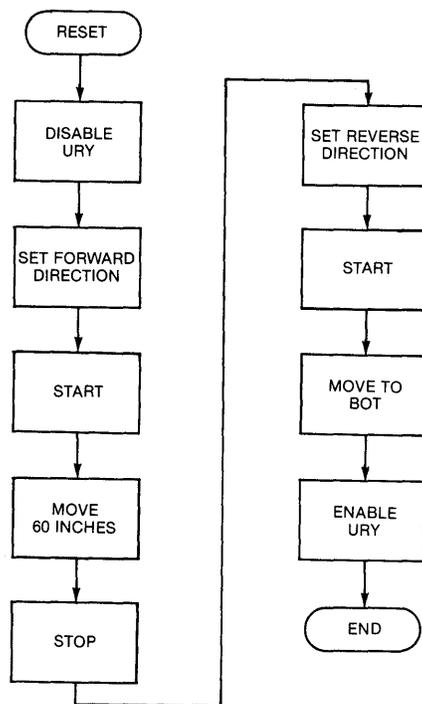
Figure 3-12 RESET OPERATION FLOWCHART
