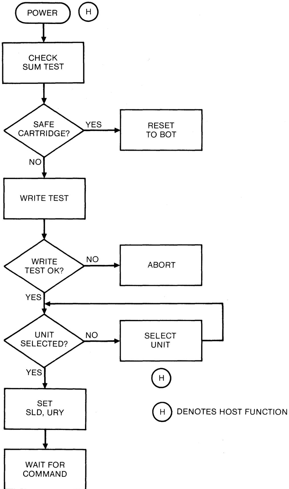
Figure 3-8 POWER-UP SEQUENCE FLOWCHART
