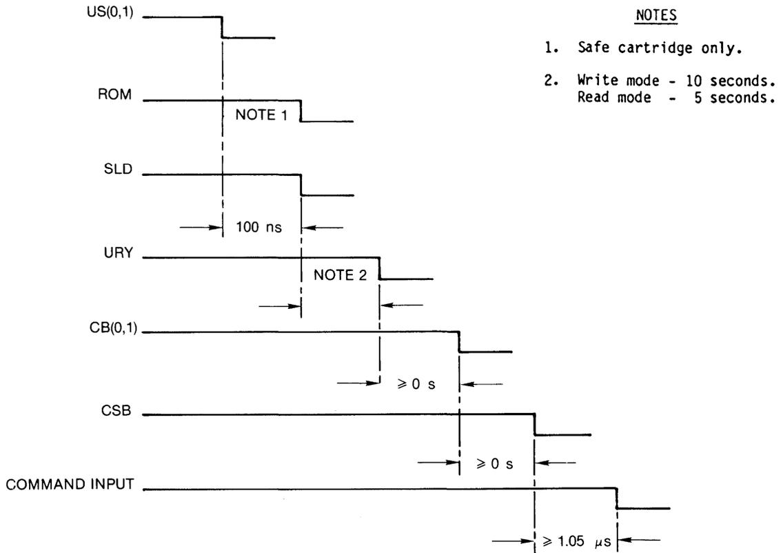
Figure 3-13 POWER-UP COMMAND, STATUS TIMING
