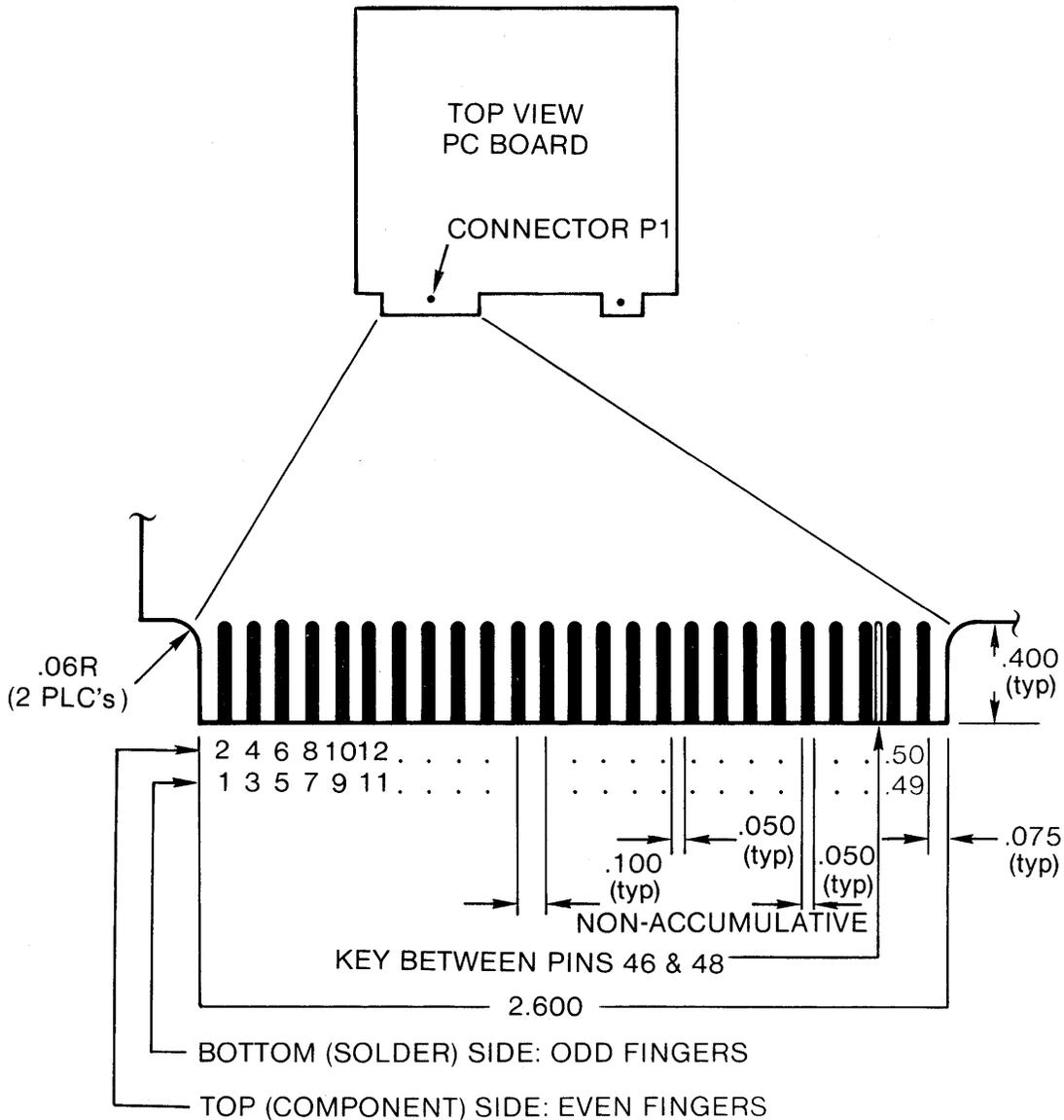
Figure 2-4 INPUT/OUTPUT CONNECTOR BOARD DETAIL
