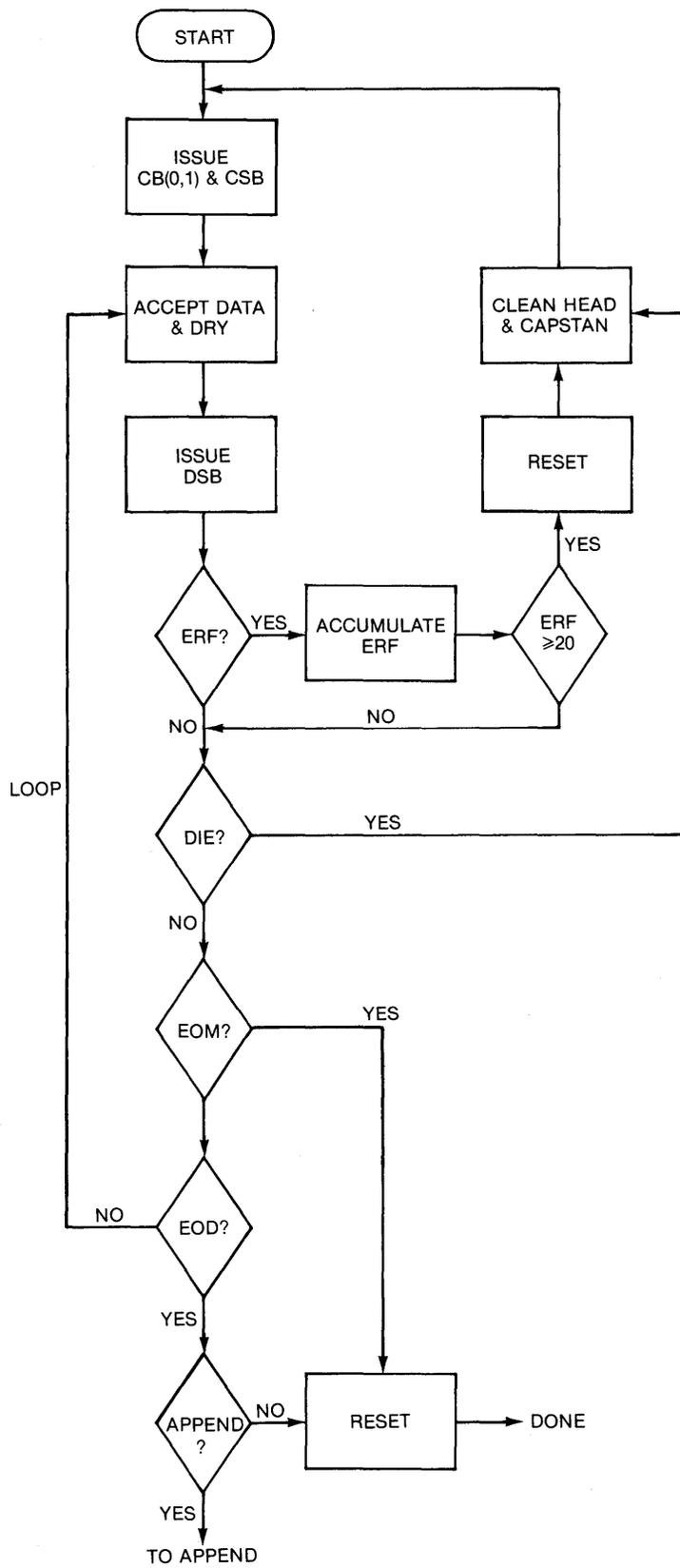
Figure 3-10 READ OPERATION FLOWCHART
