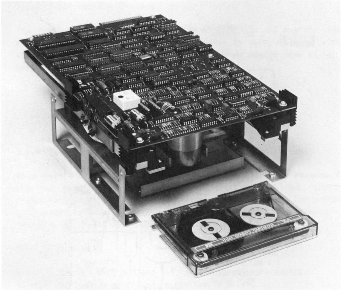
Figure 1-1 CARTRIDGE TAPE DRIVE
