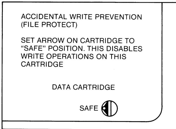
Figure 3-2 CARTRIDGE FILE PROTECTION
