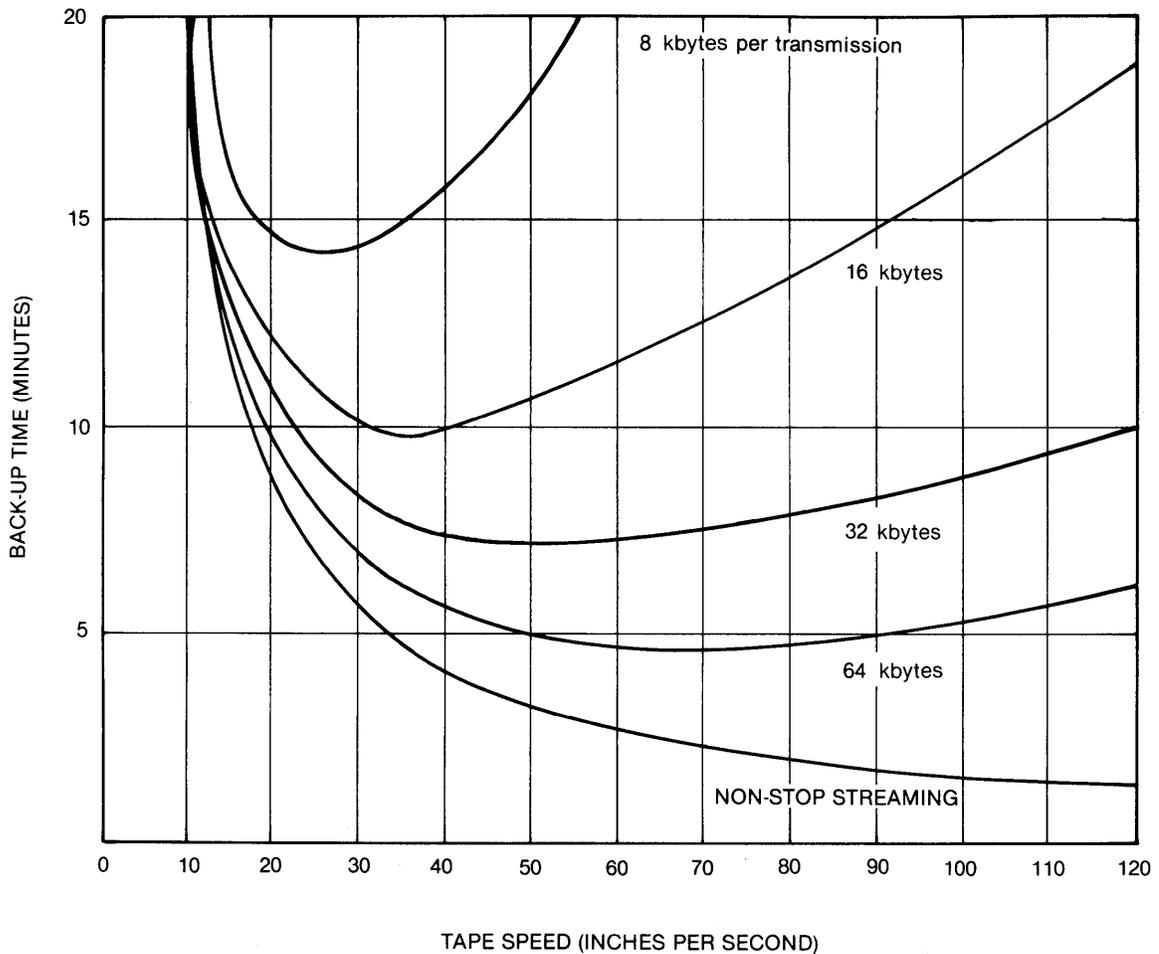
Figure 3-5: BACKUP TIME FOR 10 MBYTES OF DISK DATA VS TAPE SPEED AND DATA RECORD LENGTH
