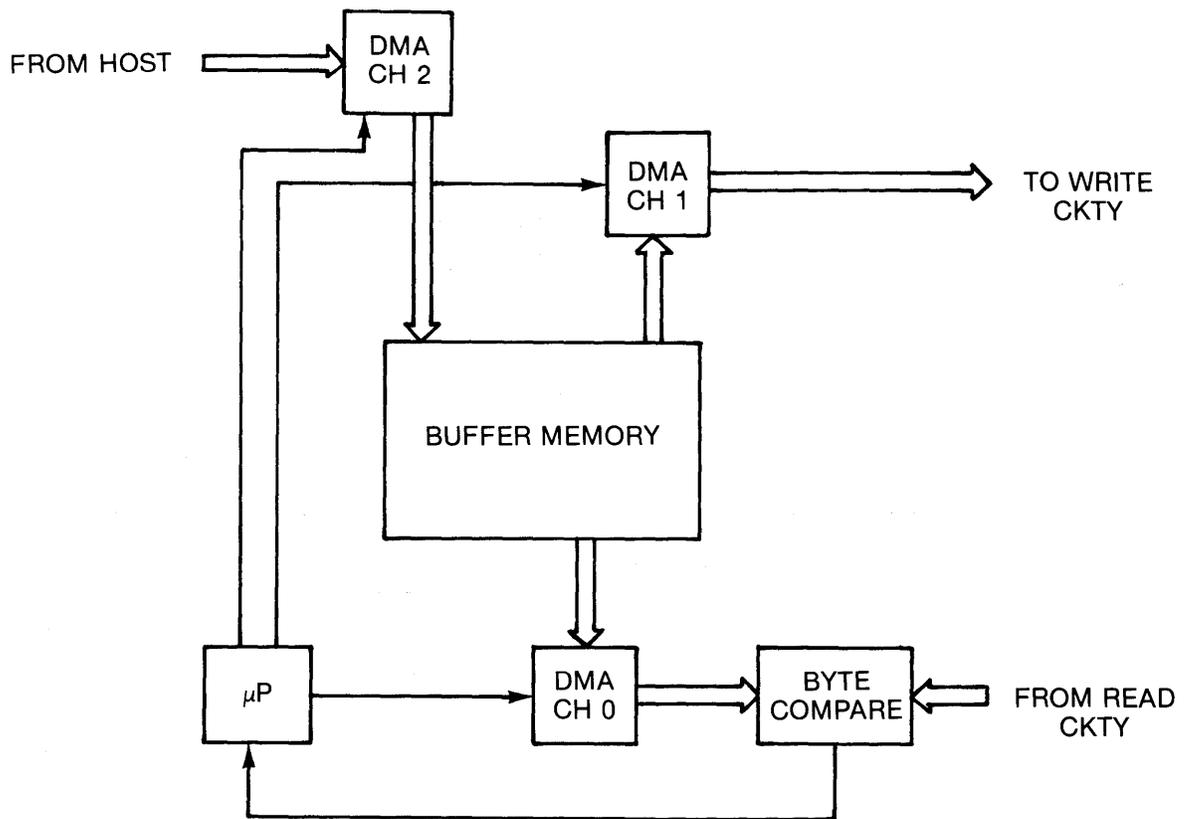
Figure 3-3 WRITE DATA FLOW
