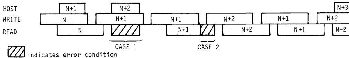
Figure 4-4 WRITE MODE ERROR REWRITES
