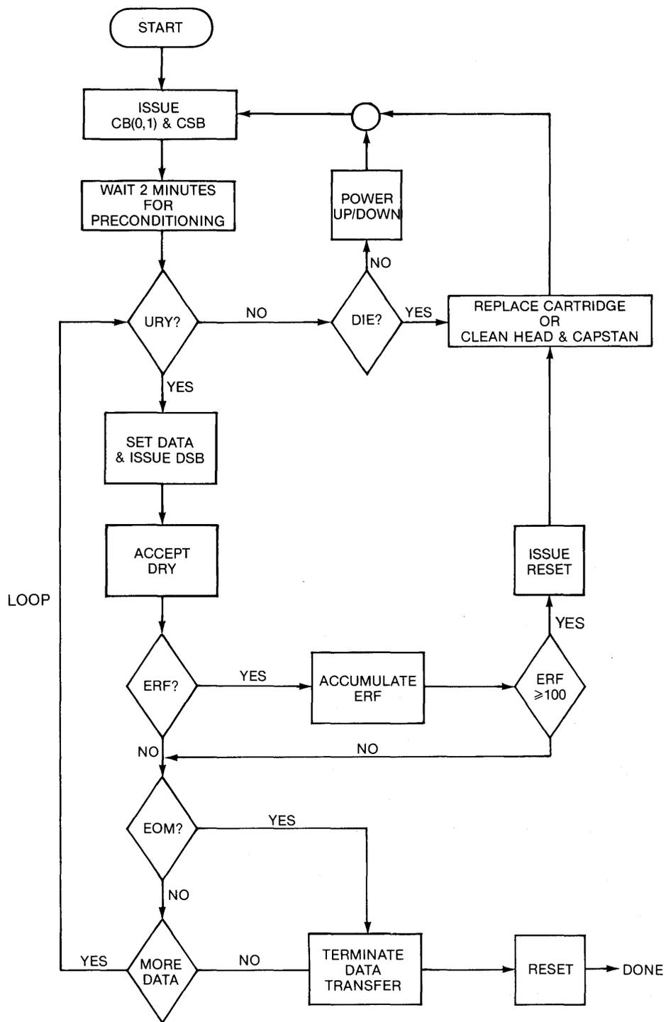
Figure 3-9 WRITE OPERATION FLOWCHART
