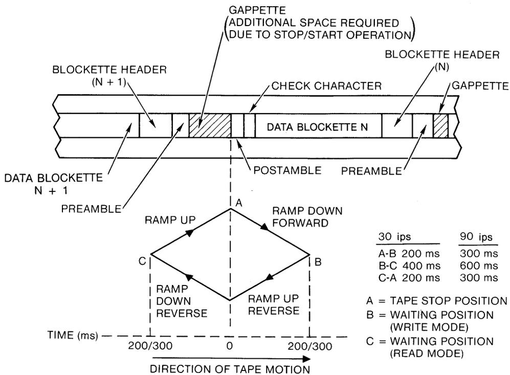
Figure 4-8 REPOSITIONING CYCLE
