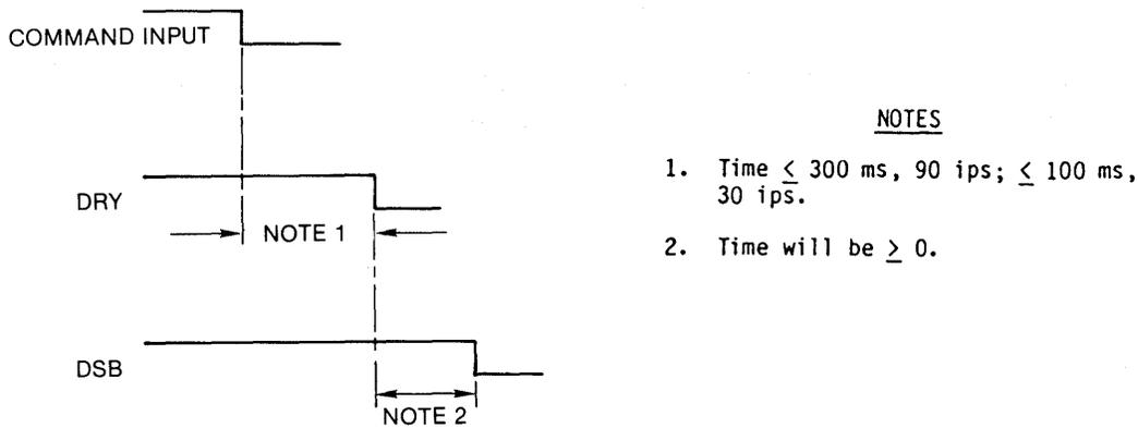
Figure 3-16 INITIAL READ TIMING
