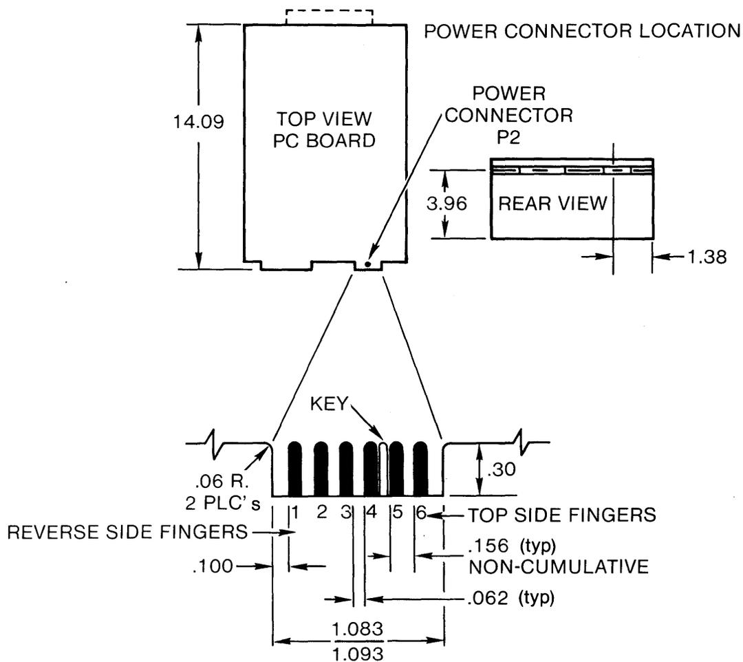
Figure 2-3 POWER CONNECTOR BOARD DETAIL
