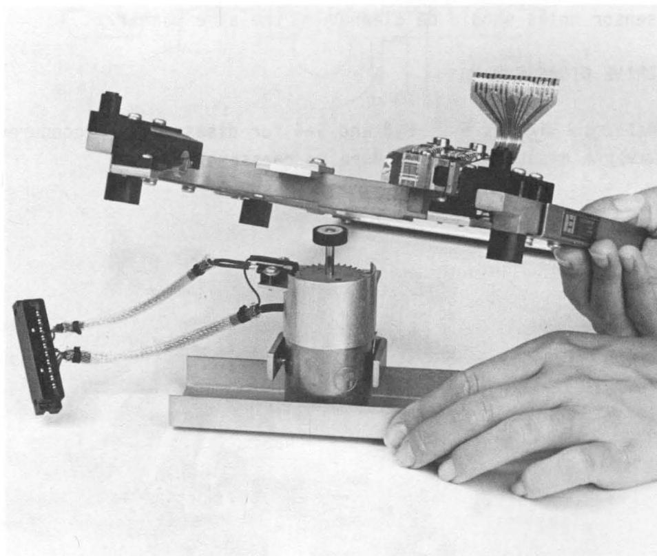
Figure 5-4 MOTOR ASSEMBLY REMOVAL
