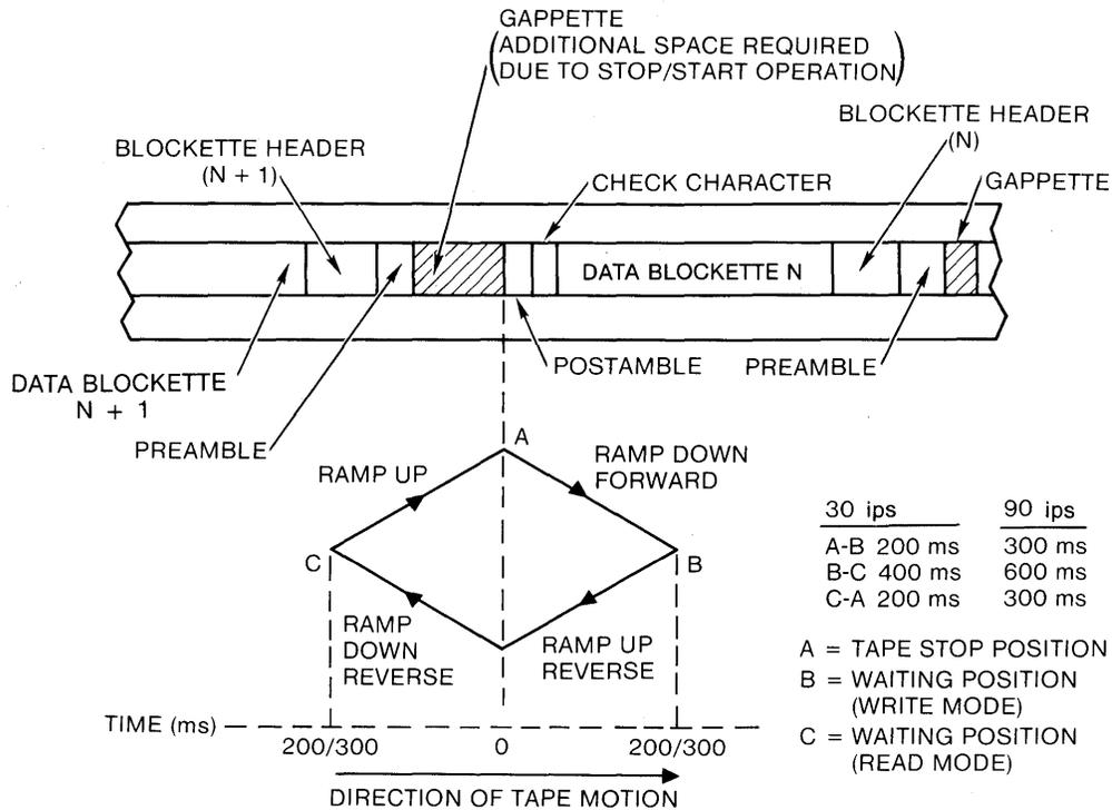
Figure 3-7 REPOSITIONING CYCLE
