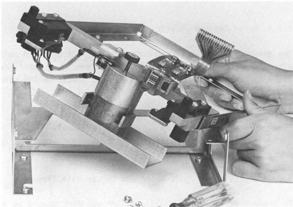
Figure 5-3 HEAD, MOTOR ASSEMBLY REMOVAL
