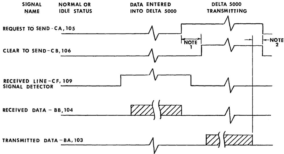
FIGURE 7-2. COMMUNICATIONS TIMING DIAGRAM
