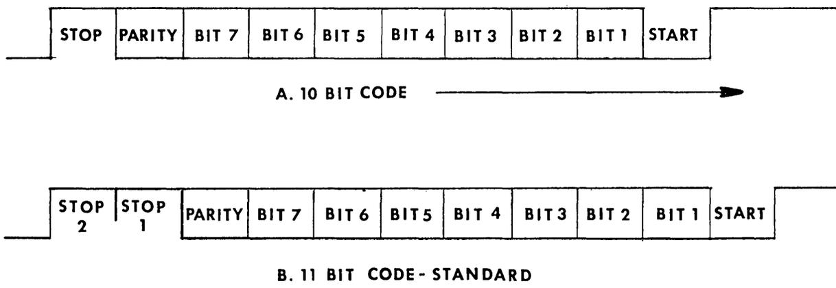
FIGURE 7-1 BIT SERIAL FORMAT
