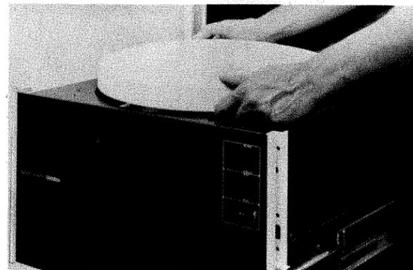
11. Slide the drive into the cabinet until the front panel latches engage and latch the drive in place.
