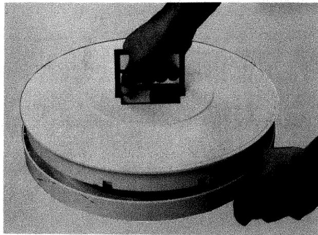
8. Hold the cartridge by the handle, and place it into the cavity on top of the drive as shown. The cartridge will fit into locating lugs when properly positioned, and slide smoothly into the cavity and seat on the spindle.
