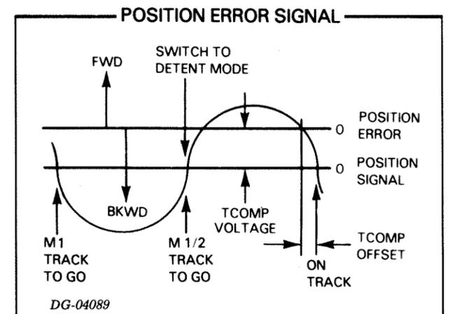
The detent operation is delayed if the linear motor current becomes excessive. This forces a reduction in the seek duty cycle and allows the motor to cool down. If an over current occurs, a 10 second cool down delay begins. During that time, all detent operations are delayed an additional 100ms.
