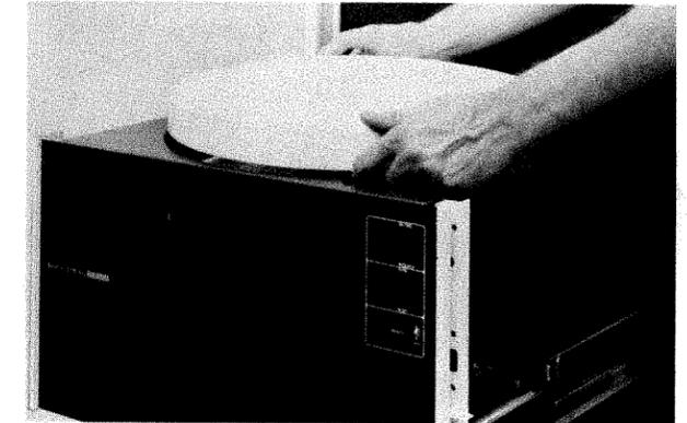
7. Remove the disc cartridge as follows:
