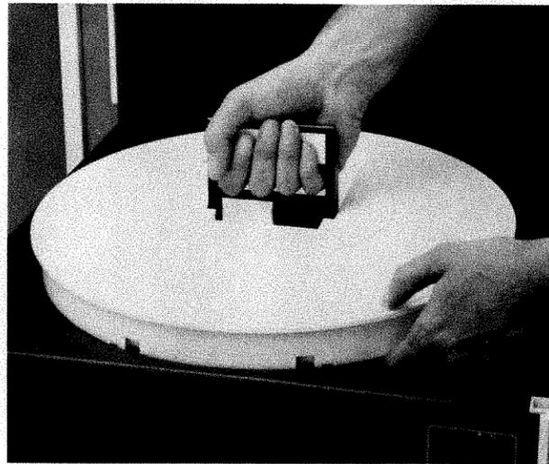
8. Place the cartridge into the dust cover, and lower the cartridge handle until it is flat on the cartridge. The dust cover will magnetically latch to the cartridge. The cartridge may now be stored in a controlled environment, in accordance with the requirements given under "Disc Cartridge Care and Handling".
