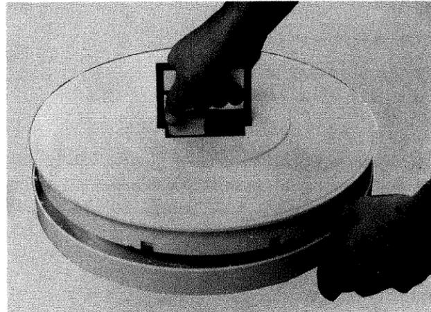
9. If another disc cartridge is to be installed, load it following the procedure under "Loading", steps 7-10. If no cartridge is to be installed, place a spare dust cover in the cavity in the disc drive, to minimize contamination in this area.
