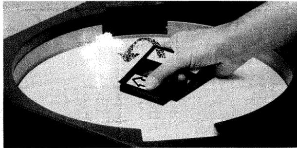
Lift the handle straight up, and carefully lift the disc cartridge straight up and out of the drive.
