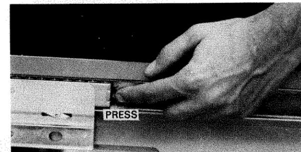
**NOTE** *If the drive is inadvertently moved beyond the operator's position by releasing the detents, it can be moved back by releasing the detents as shown.*
