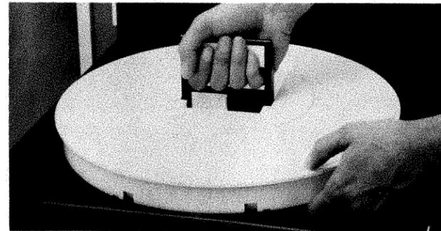
9. Lower the cartridge handle until it is flat on the cartridge.
