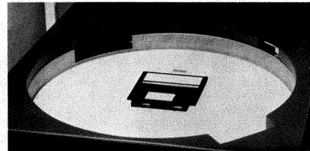
10. Place the dust cover over the cartridge. Ensure that it seats in the cavity.
