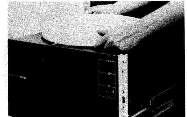
**NOTE** *It is good practice to ensure that the cavity and spindle are clean and free of dust and contaminants. Use a lint-free tissue to clean the cavity and spindle if necessary.*
