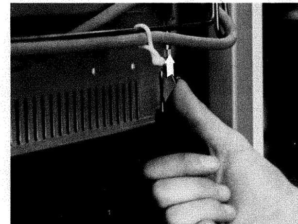
7. If the cartridge disc does not slide easily into the cavity in the drive, ensure that it is positioned correctly and engaged on the locating lugs. If difficulty is still encountered, examine the cavity and the underside of the cartridge for obstructions, such as paper clips, staples, or excess contamination. Clean the areas using a lint-free tissue and isopropyl alcohol, if necessary. If interference still persists, do not operate the drive, and contact technical personnel for assistance.
