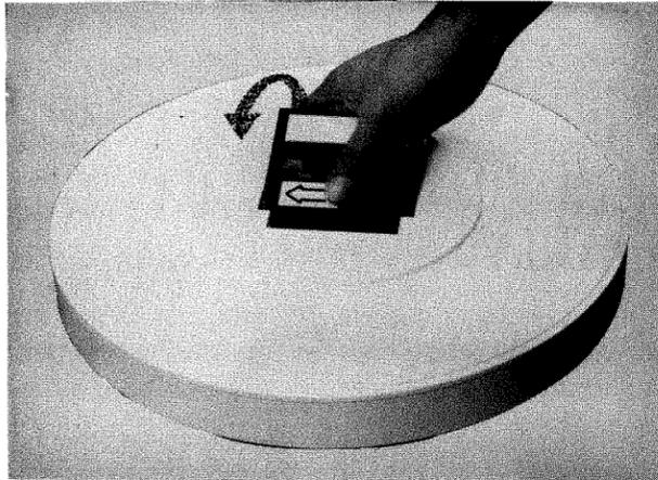
Lift the handle straight up, and lift the cartridge up and out of the dust cover.
