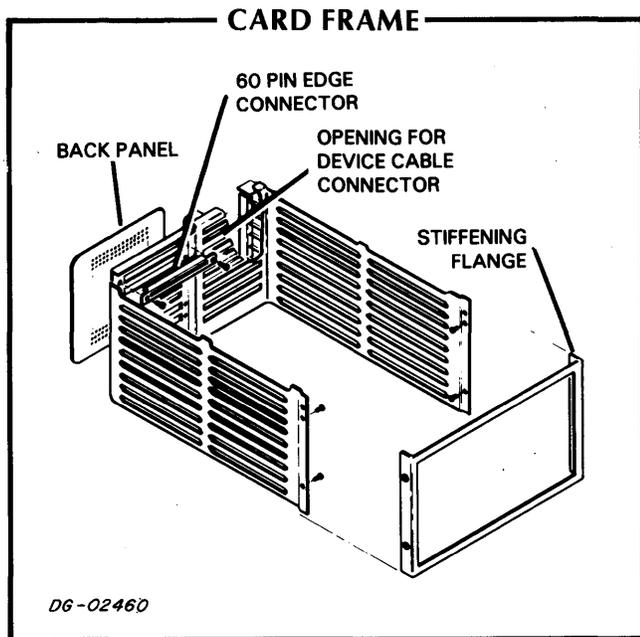
The printed circuit backpanel carries memory and I/O signals among the boards installed in the cardframe, and delivers the necessary power to the boards from the power supply. Etch on the backpanel passes all signals in parallel from one 60 pin edge connector to the next. Every contact on all edge connectors corresponds to a wire-wrap pin protruding from the rear of the backpanel; the pins are spaced so that
