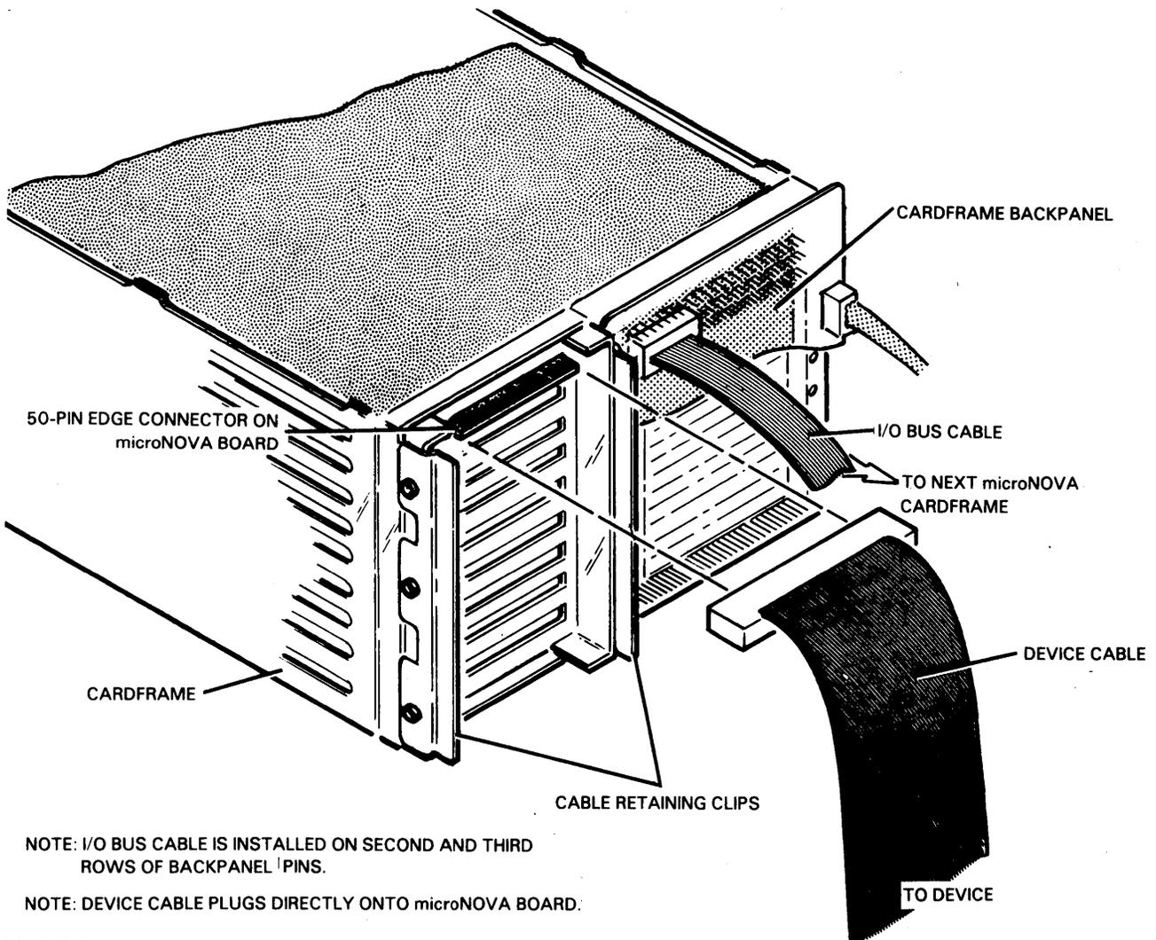
NOTE: I/O BUS CABLE IS INSTALLED ON SECOND AND THIRD ROWS OF BACKPANEL PINS.
