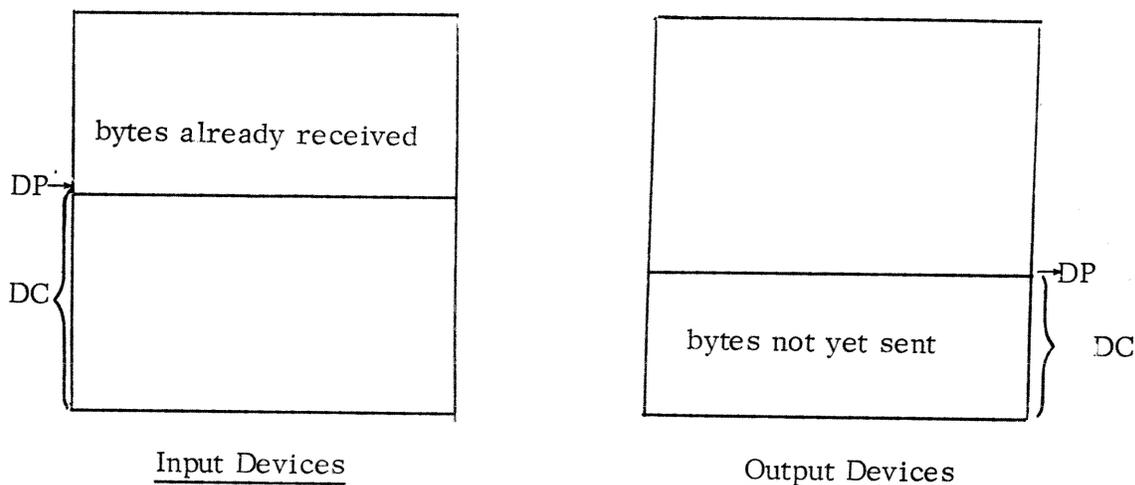
Pointer DP indicates the current slot in the user area which is targeted for storage or retrieval of data by the device. Counter DC indicates the number of slots in the area which remain to be processed.
