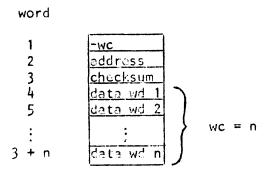
The two's complement of the number of data words in the block is given in the first word (therefore bit 0 is a 1). Normally 16 data words will be punched per data block. However, the .END and .LOC pseudo-ops may cause
