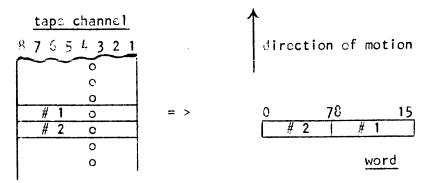
In other words, the first tape character forms bits 8-15 of the data word (Channel 8 to bit 8, etc.) and the second tape character forms bits 0-7 of the data word (Channel 8 to bit 0, etc.). The first non-null tape character signifies that start of a block. The block type is determined by the first word read. A description of each block type follows:
