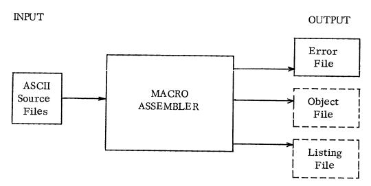
Broken boxes in the diagram represent optional output.
