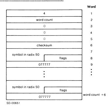
The third word of each user symbol entry in the External Displacement Block is set to 077777.
