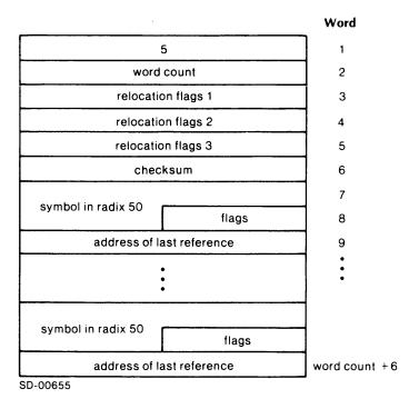
The third word of each user symbol entry in the Normal External Block contains the address of the last reference. Relocation flags are used as in .ENT blocks. There is a limit of  $^{15}10$  symbols per block because of space required for relocation flags.
