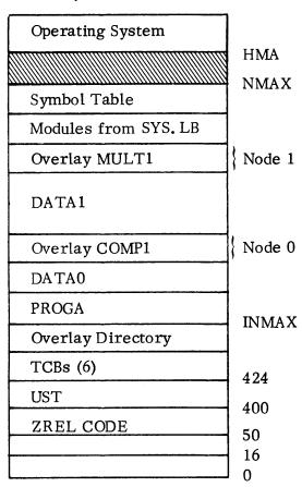
In a mapped RDOS system, the system would not be at the "top" of memory, but it would be invisible to your programs, so the example is useful nonetheless. PROGA would have the same structure if it ran in the foreground, but addresses 0 through HMA would be foreground locations. This would not affect execution.
