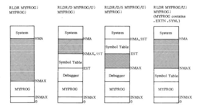
Aside from the position of the system, these diagrams apply to both mapped systems and background programs in unmapped systems.
