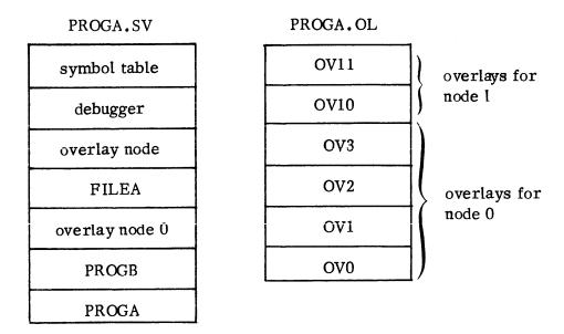
The /D global switch loaded the symbol table, but also loaded the debugger. To conserve memory space, you can load only the symbol table by including it as an external normal in one of the source modules (e.g., in PROGB or FILEA):
