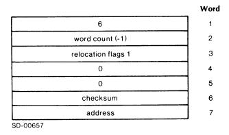
Bits 0 - 2 of the first relocation flag word are used for address relocatability; other bits of word 3 are 0.
