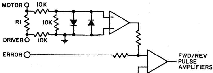
Figure 4-33 CARRIAGE FEEDBACK INSTRUMENTATION CIRCUIT
