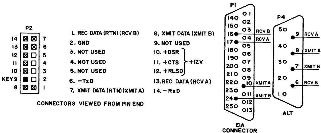
Figure 2-9 CURRENT LOOP I/O CABLE CONNECTOR PIN ASSIGNMENT
