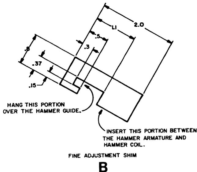
Figure 5-32 HAMMER ADJUSTMENT TOOL #40796 and SHIM
