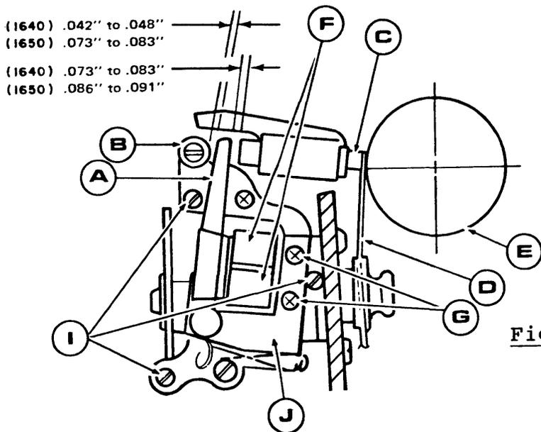
Figure 5-31 HAMMER ADJUSTMENTS
