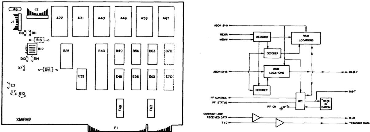
Figure 4-10 XMEM2 PCB LAYOUT AND BLOCK DIAGRAM
