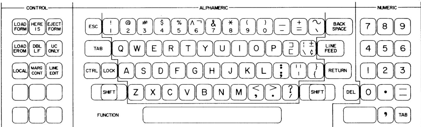
**Figure 2-14 STANDARD KEYBOARD ASSIGNMENTS - KSR MODELS**
