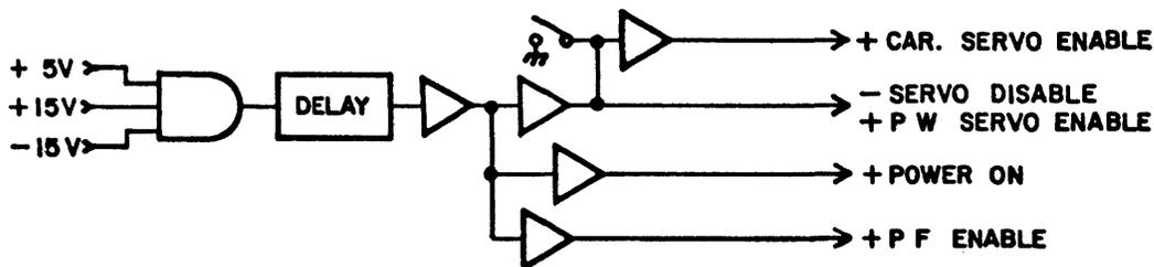
Figure 4-34 POWER MONITOR CIRCUIT BLOCK DIAGRAM
