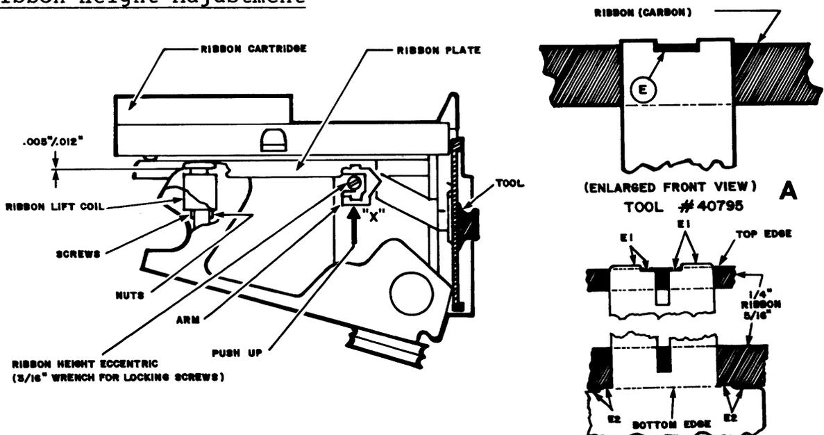
**Figure 5-23 RIBBON HEIGHT ADJUSTMENT**
