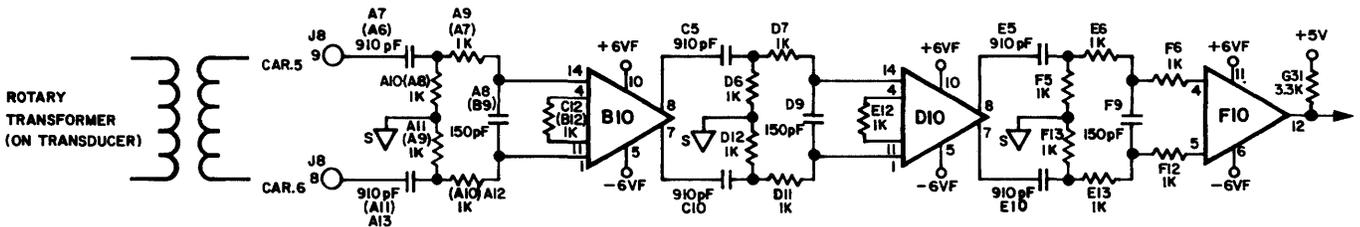
Figure 4-21 SERVO FEEDBACK AMPLIFIER
