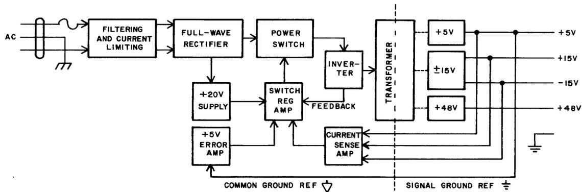
Figure 4-44 INTERNAL POWER SUPPLY BLOCK DIAGRAM, U
