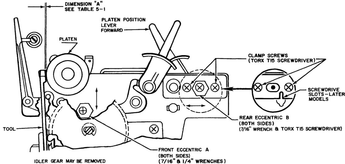
Figure 5-20 PLATEN TO PRINT WHEEL ADJUSTMENT POINTS
