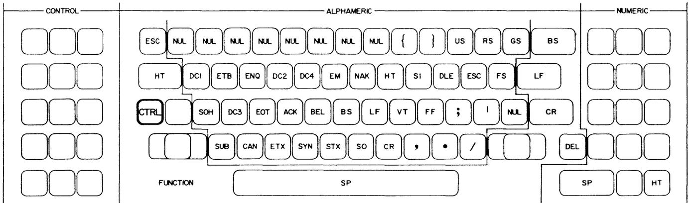
**Figure 2-16 CTRL MODE KEY ASSIGNMENT**
