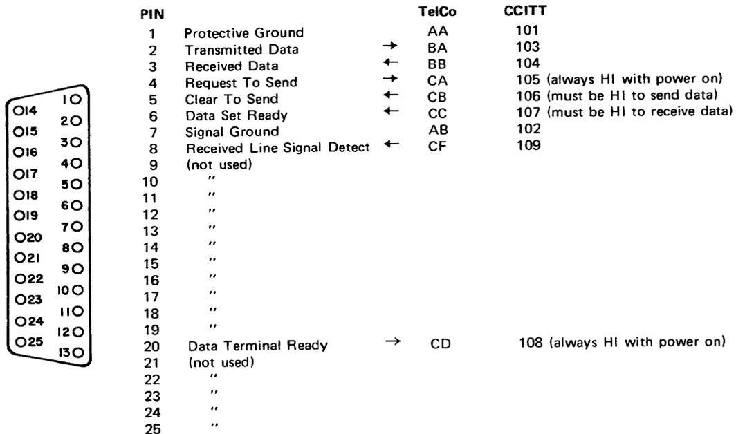
**Figure 2-7 SERIAL I/O CABLE CONNECTOR PIN ASSIGNMENT**
