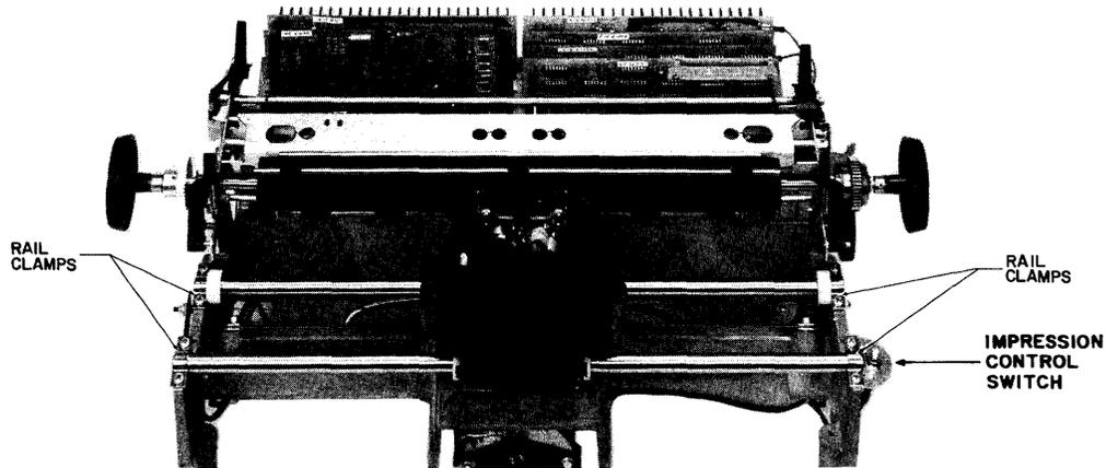
Figure 5-18 CARRIAGE RAIL CLAMPS
