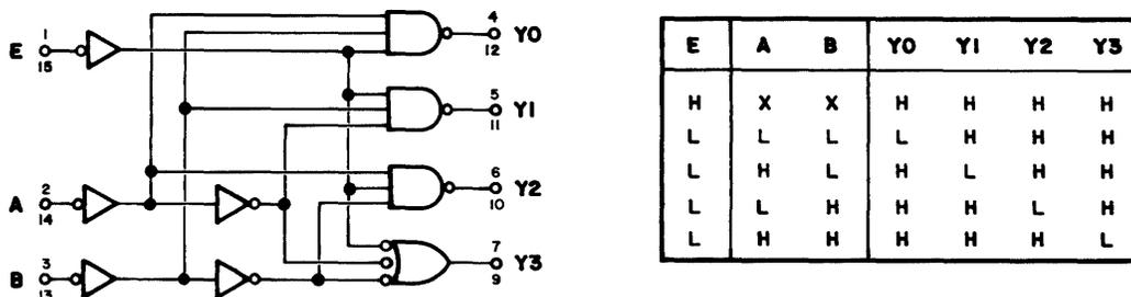
**Figure 4-11 2 TO 4 LINE DECODER DIAGRAM AND TRUTH TABLE**
