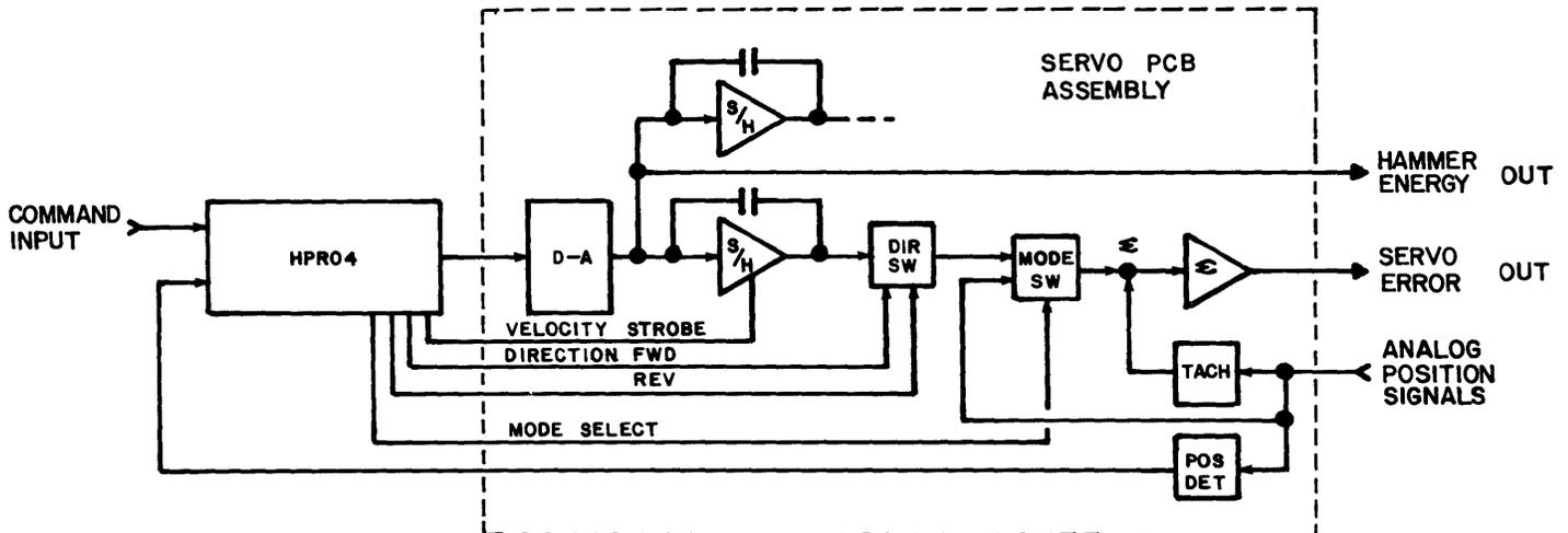
Figure 4-26 SERVO PCB BLOCK DIAGRAM
