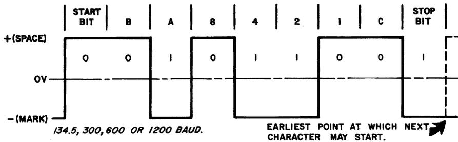
**Figure 4-6 2741 OPTION DATA FORMAT ON INTERFACE**
