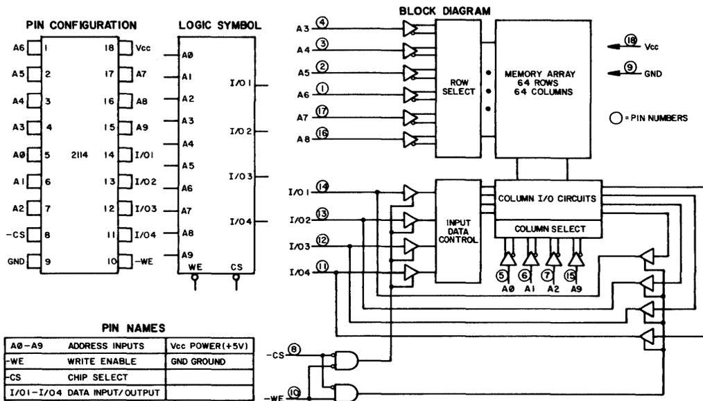
These modules are 1024 x 4 bit static RAM. They act as buffer data storage devices for both expanded memory and word processing scratch pad memory. Their I/O connections go to the data bus on the HPRO4 PCB, and their operation is controlled by the HPRO4's CPU via the address bus and the decoder modules discussed earlier. Figure 4-14 includes the RAM block diagram and chip pin assignment.
