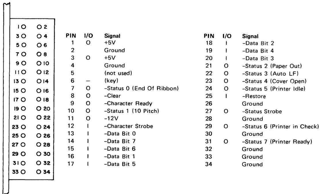
**Figure 2-8 PARALLEL I/O CABLE CONNECTOR PIN ASSIGNMENT**
