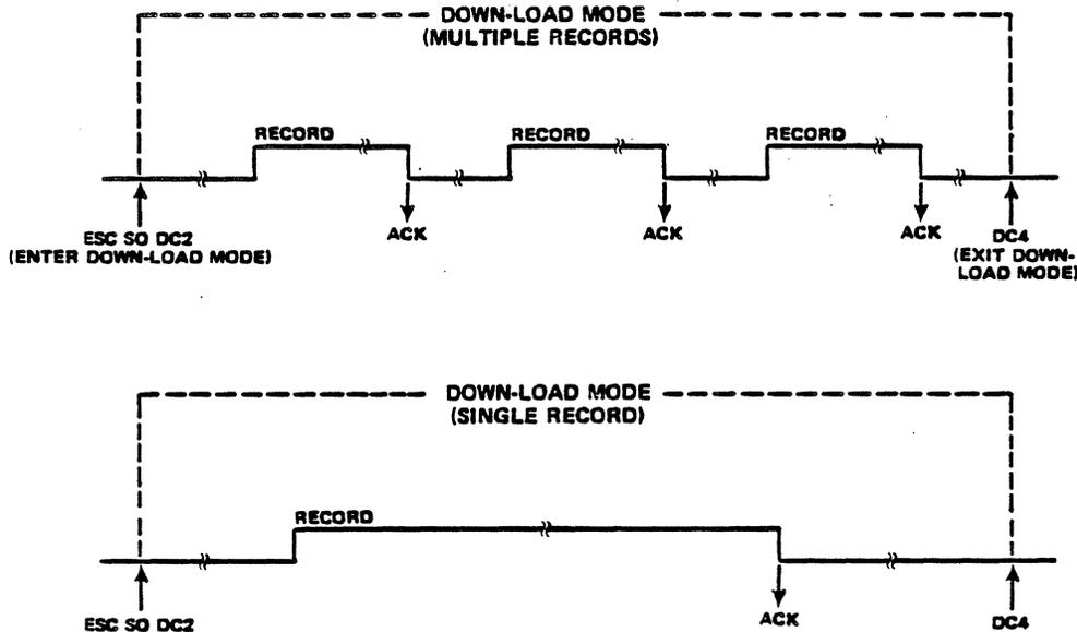
**Note:** The total amount of Table Data stored by either a Single-Record Down-Load or Multiple-Record Down-Load is 192 bytes for non-ECS table, or 384 bytes for ECS table (2 bytes for each possible character position on print wheel).
