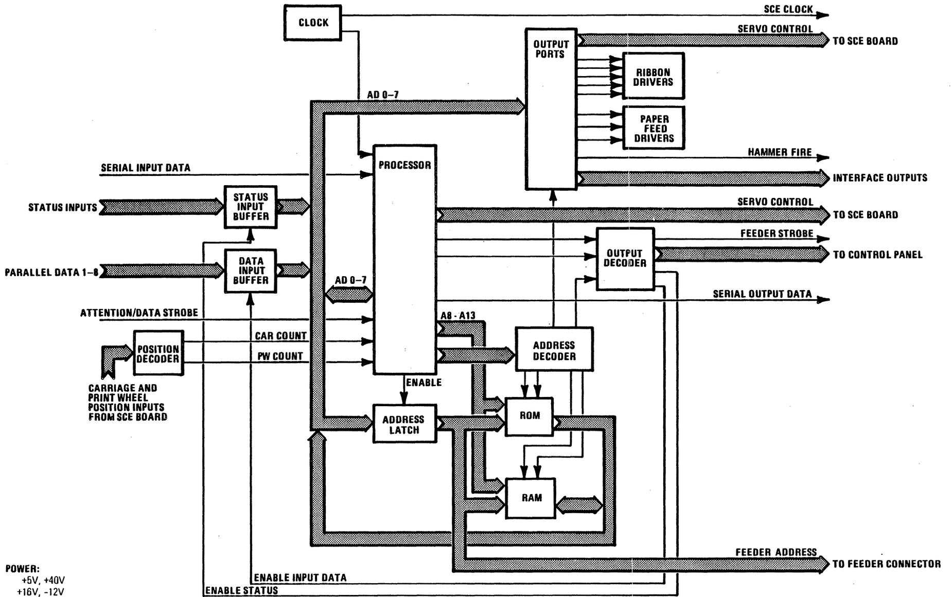
Figure 1-3. API CIRCUIT BOARD BLOCK DIAGRAM
