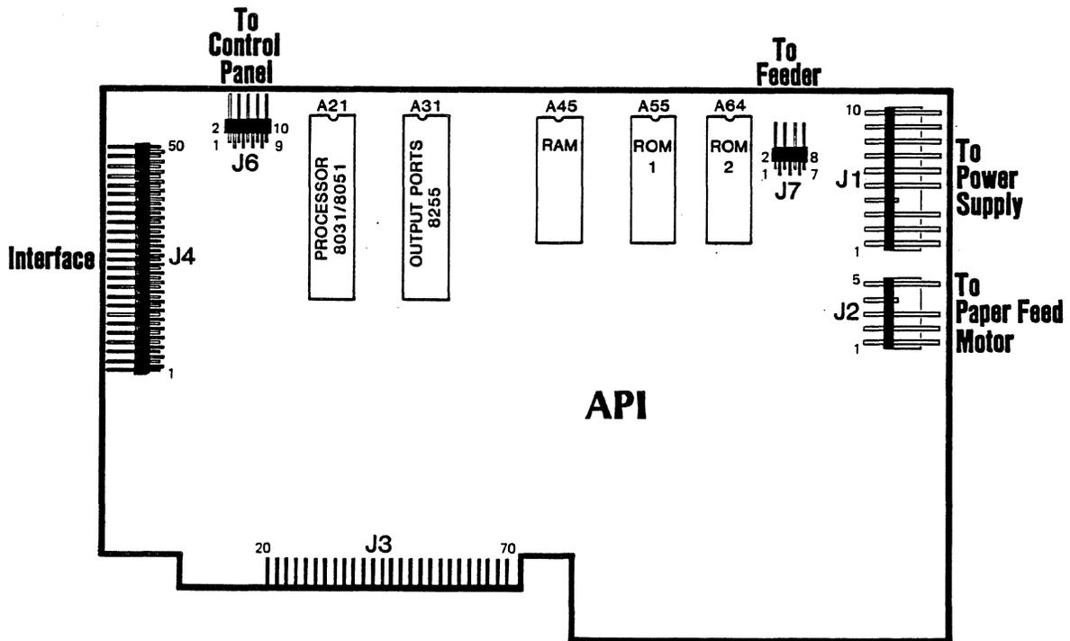
Figure 2-1. API CIRCUIT BOARD LAYOUT
