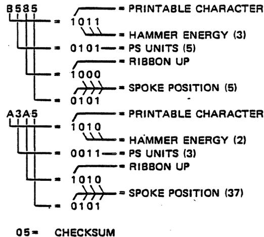
Figure 3-7. SAMPLE DOWN-LOAD STRUCTURE
