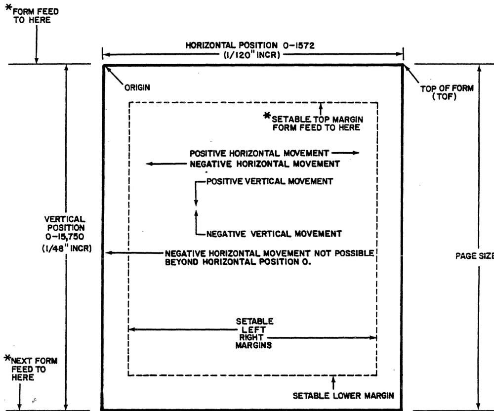
Width of Print Position = Horizontal Motion Index (HMI) and is variable from 0 to 125 (1/120") increments.
