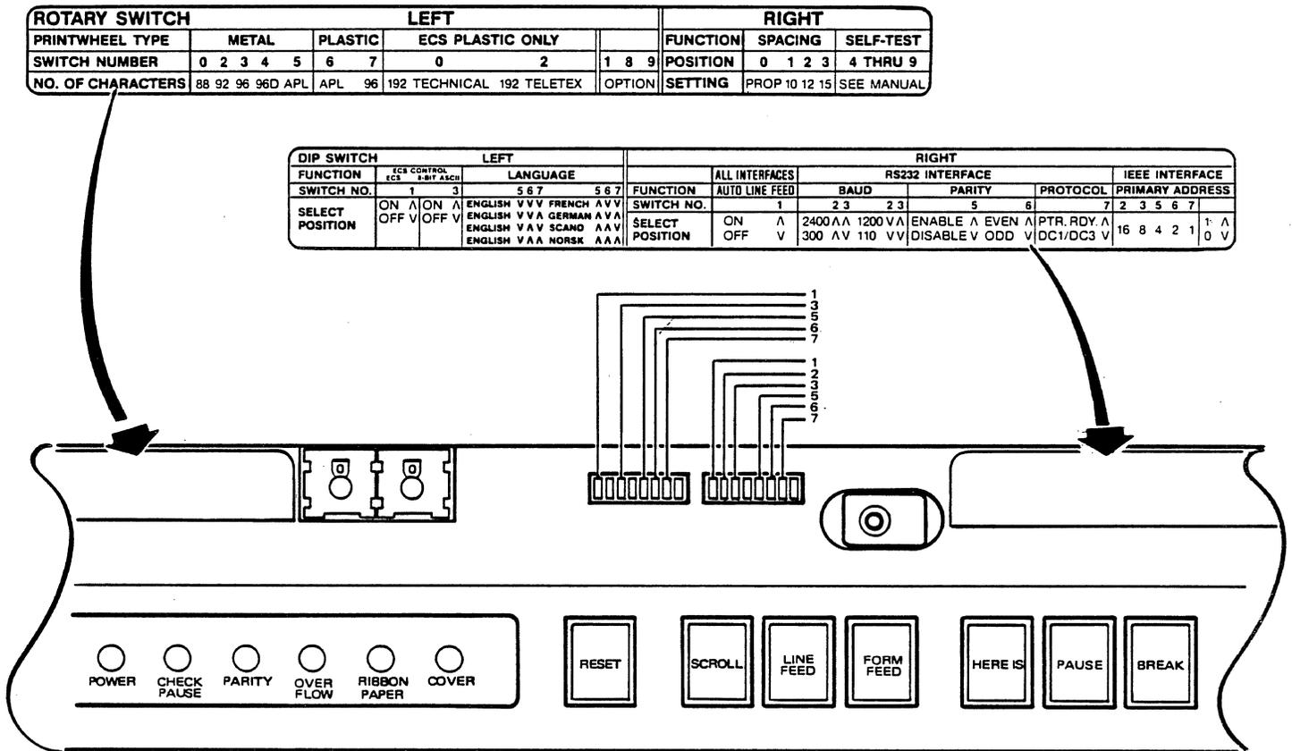
Figure 3-2. MODEL 630 API-2 CONTROL PANEL
