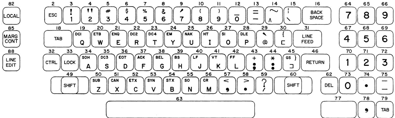
Figure 5-3. 47-KEY LOGICAL BIT PAIRED KEYBOARD
