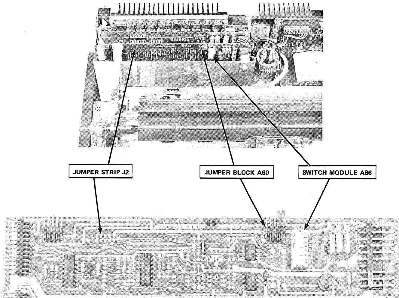
Figure 3-1. HPRO5 CIRCUIT BOARD JUMPERS AND SWITCHES
