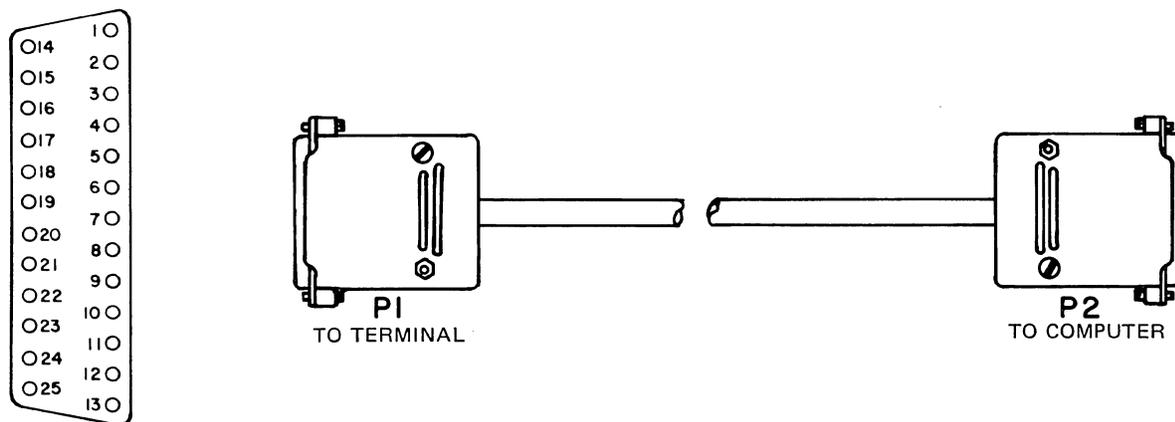
Figure 2-3. CURRENT LOOP INTERFACE CONNECTOR AND CABLE
