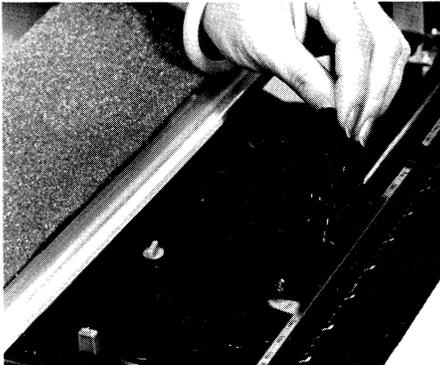
Because the printer's plastic printwheels are notchless and hubless, users are not required to position the printwheels over a drive shaft or to align the corresponding drive shaft and printwheel notches or other markings.
