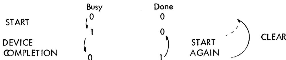
The data-in or data-out instruction that the program gives in response to the setting of Done can also restart the device. When all the data has been transferred the program generally clears Done so the device neither requests further interrupts nor appears to be in use, but this is not necessary. Busy and Done both set is a meaningless situation.
