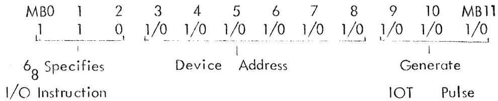
In general, if information is to be transferred to or from the peripheral device, the transfer is to or from the accumulator register to or from the device. Thus, on outputs to the device, the information to be transferred must be placed in the accumulator prior to the I/O instruction, and, on inputs, the information transferred will be in the accumulator after the I/O instruction.
