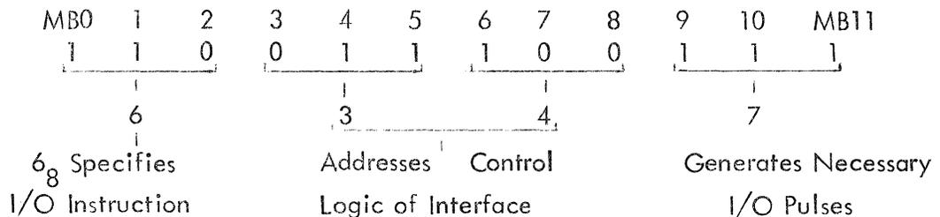
This instruction will always serve to transfer the 12-bit contents of the accumulator to the control logic section of the interface. The contents of the accumulator will then be decoded to determine whether the function to be performed is a command for tape action or for status input.
