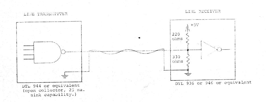
Figure 1. Transport/Controller Interface Circuit.
