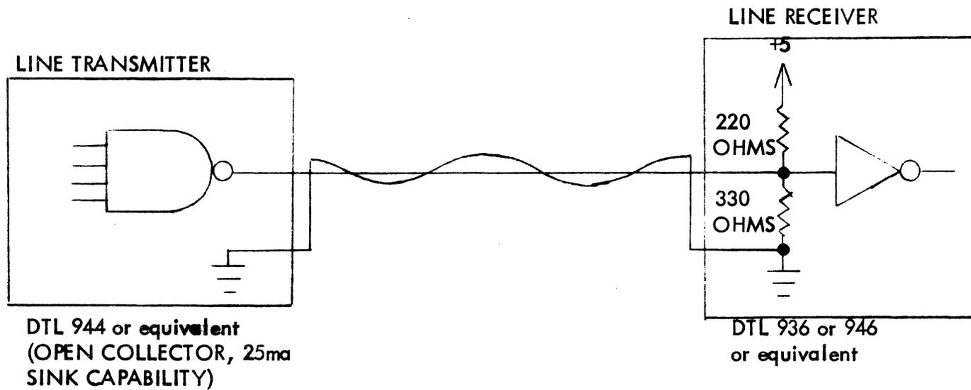
FIGURE I CONTROLLER/FORMATTER INTERFACE CIRCUIT
