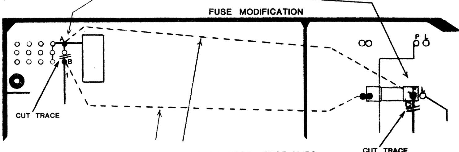
**FIG. 2 ADD TWO WIRES TO CONNECT FUSE CLIPS ON BACKSIDE OF BOARD**
