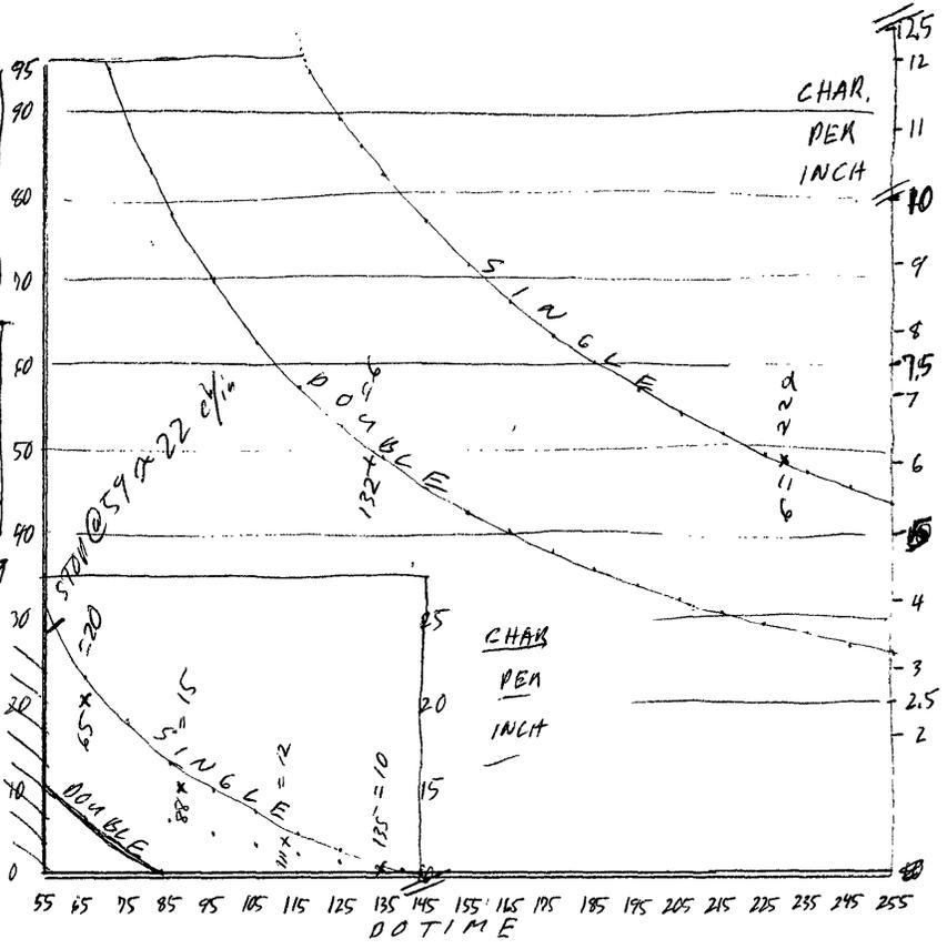
$$\text{COL. WIDTH} = A + B \times \text{NO. OF CHAR.} \times \text{DOTIME}$$
