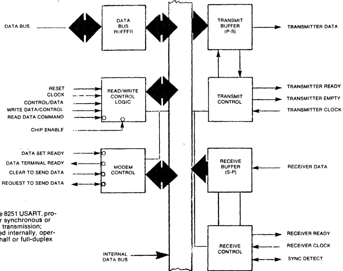
Figure 1 — The 8251 USART, programmable for synchronous or asynchronous transmission; double buffered internally, operates in either half or full-duplex mode.
