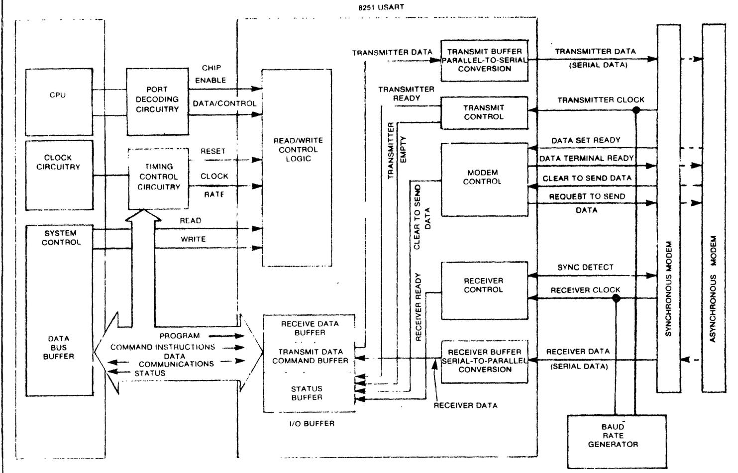
Figure 2 — 8251's implemented in a microcomputer system.
