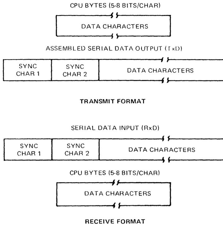
After the functional definition of the  $\mu$ PD8251 has been specified by the Mode Instruction and the SYNC character(s) have been entered, if in SYNC mode, the USART is ready to receive Command Instructions and begin communication. A Command Instruction is used to control the specific operation of the format selected by the Mode Instruction. Enable Transmit, Enable Receive, Error Reset and Modem Controls are controlled by the Command Instruction.
