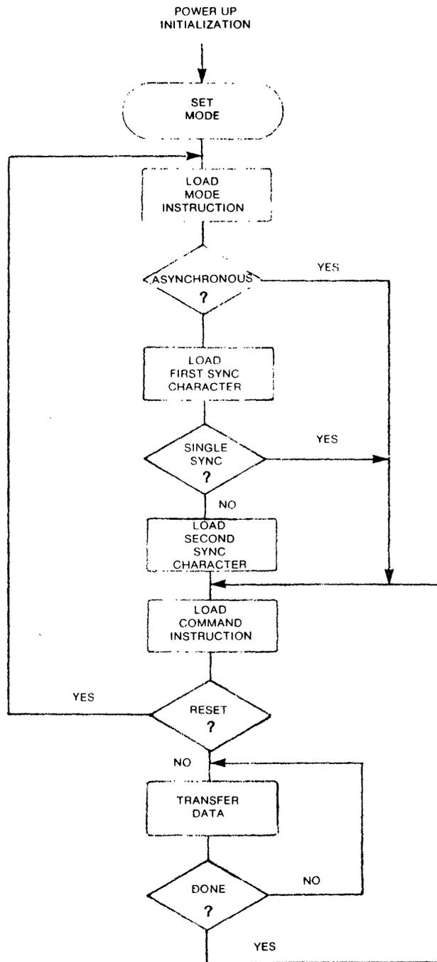
TYPICAL PROGRAMMING FLOWCHART AFTER POWER-UP RESET
