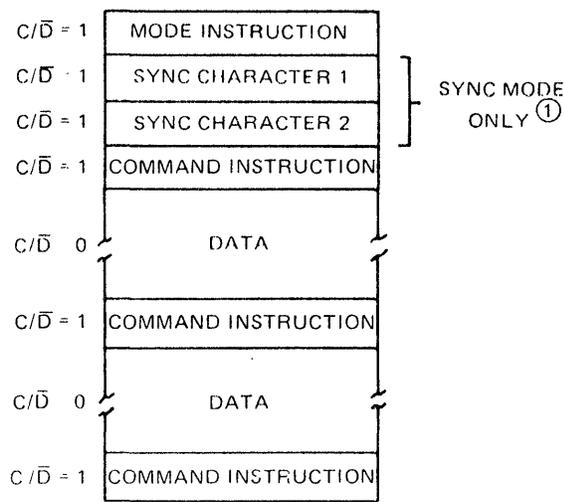
NOTE ① The second SYNC character is skipped if MODE instruction has programmed the 8251 to single character Internal SYNC Mode. Both SYNC characters are skipped if MODE instruction has programmed the 8251 to ASYNC mode.
