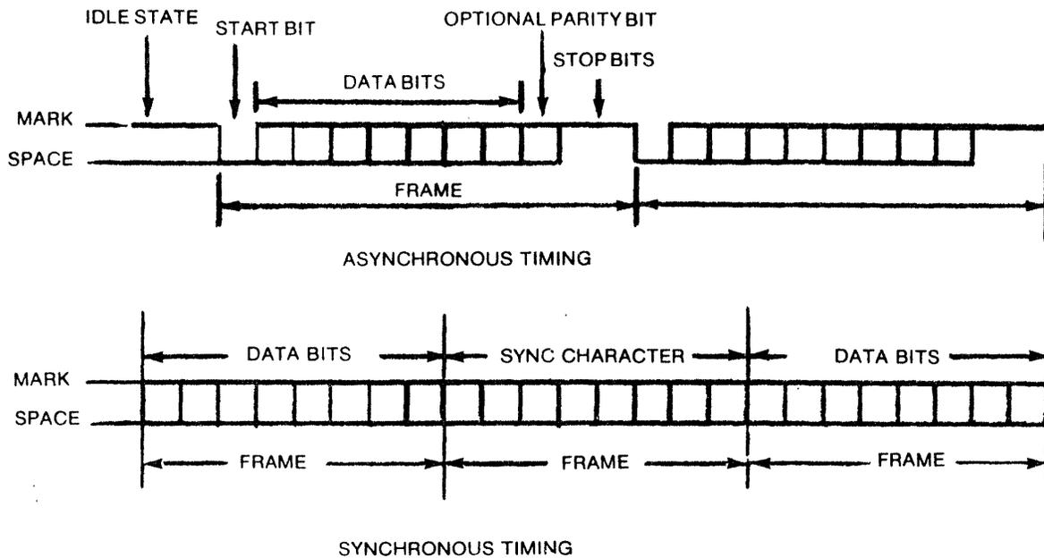
FIG. 12- TRANSMITTER/ RECEIVER FORMATS
