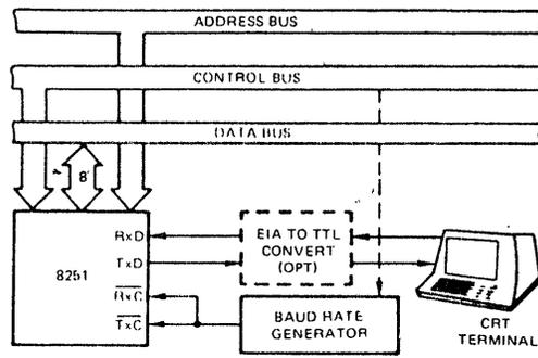
**ASYNCHRONOUS SERIAL INTERFACE TO CRT TERMINAL,
