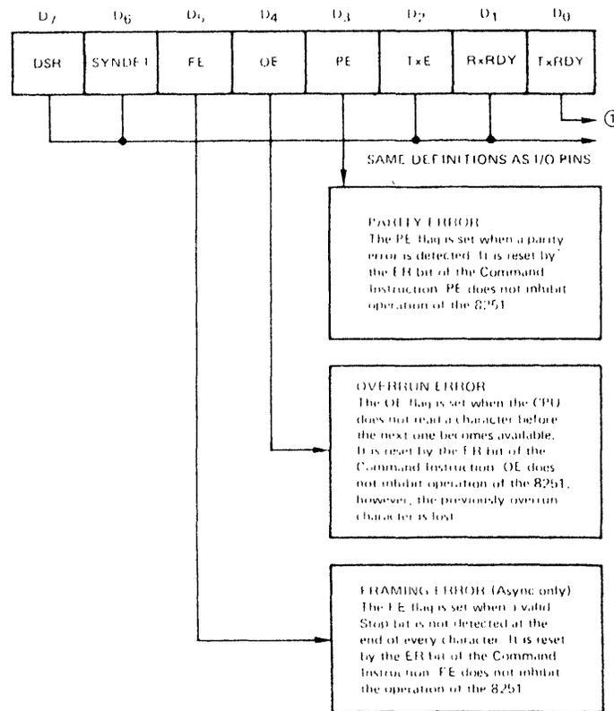
Note ① TxRDY status bit is not totally equivalent to the TxRDY output pin, the relationship is as follows:
