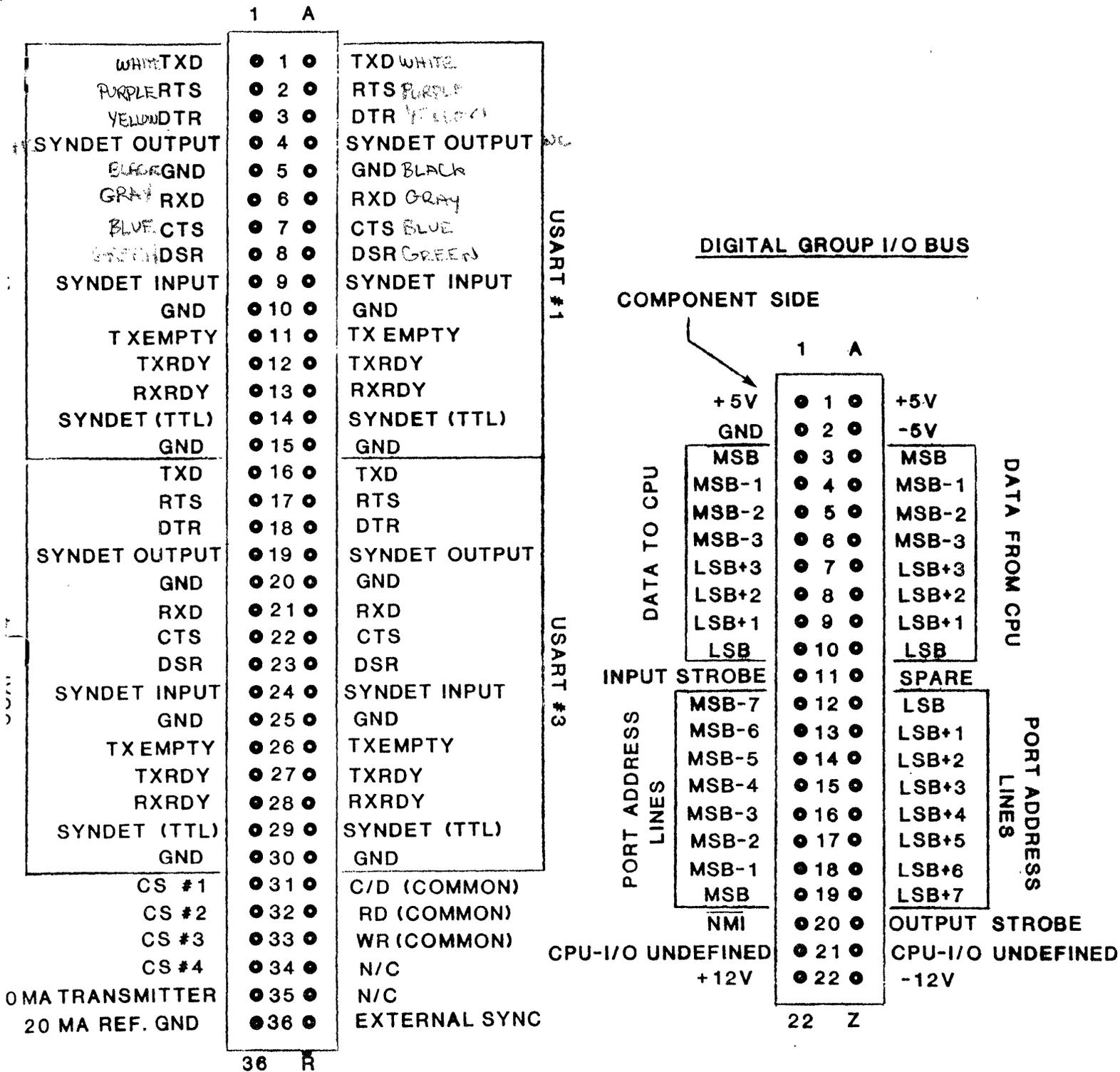
FIG. 8- PINOUT OF COMMUNICATIONS CARD 36 AND 22 PIN DUAL EDGE CONNECTORS. SEE SCHEMATIC DIAGRAM FOR LOGIC (ACTIVE HIGH AND LOW SIGNALS).
