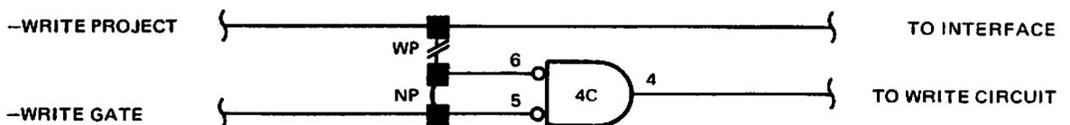
Figure 30. Write Protect Circuit
