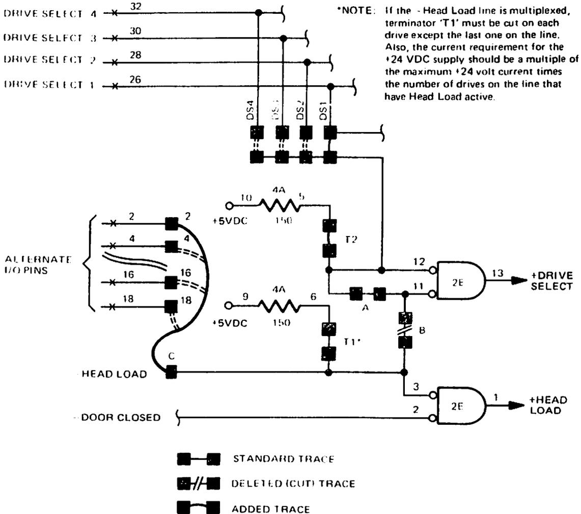
Figure 22. Select Drive Without Loading Head Circuit
