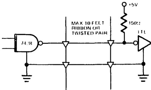
Figure 10. Interface Signal Driver/Receiver
