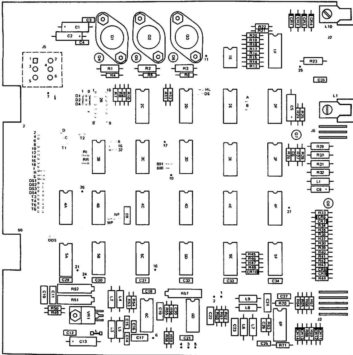
Figure 20. SA800/801 PCB Component Locations
