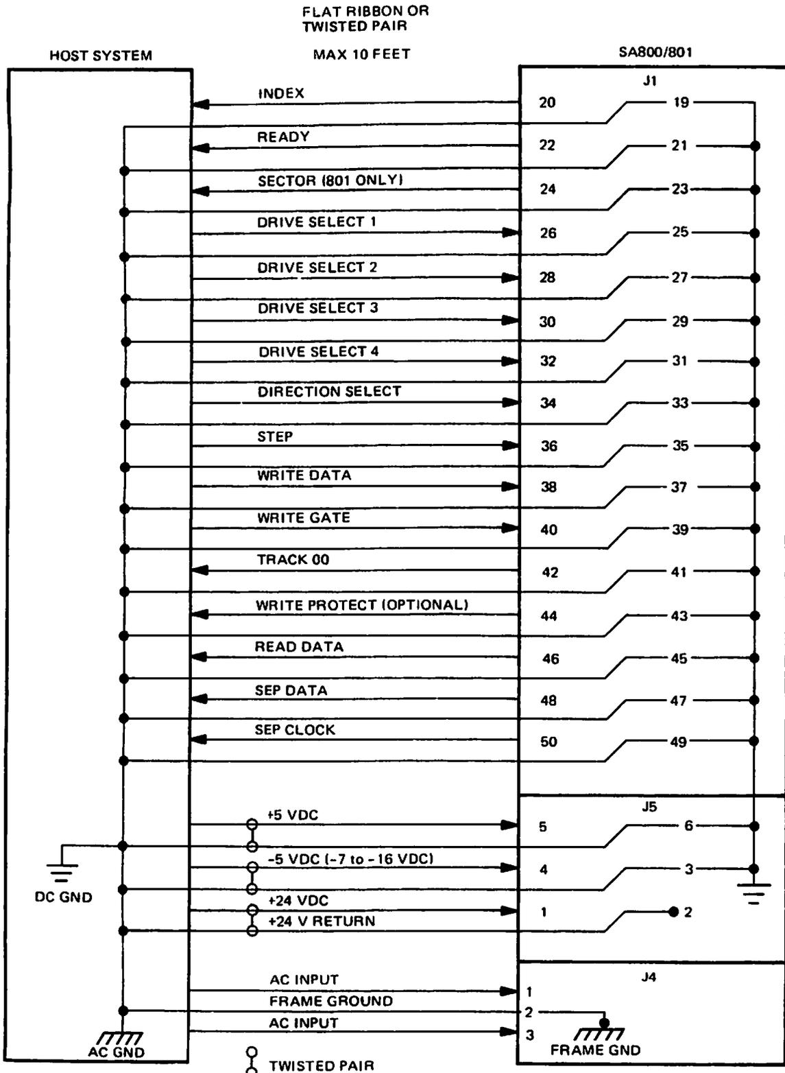
NOTE: Not shown are the nine Alternate I/O connections. The connections for these lines are on pins 2, 4, 6, 8, 10, 12, 14, 16, and 18. Signal return for these lines are on pins 1, 3, 5, 7, 9, 11, 13, 15, 17, and 19 respectively. Reference section 7 for uses of these lines.
